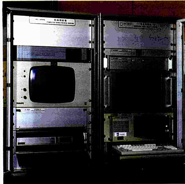
Fig. 4.16. Review station CARES for safeguards video surveillance
