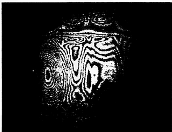
Fig. 5.2. Structural damage (decohesion between cylindrical shell and internal frame) revealed by pulsed laser holographic interferometry.
