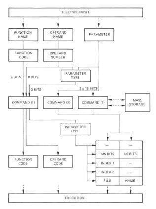
Fig. 2 Structure of the command coding and decoding in the CAMAC Operating System
