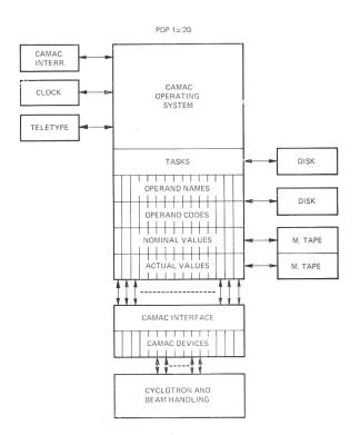
Fig. 1 Scheme of the hardware and software of the cyclotron control system
