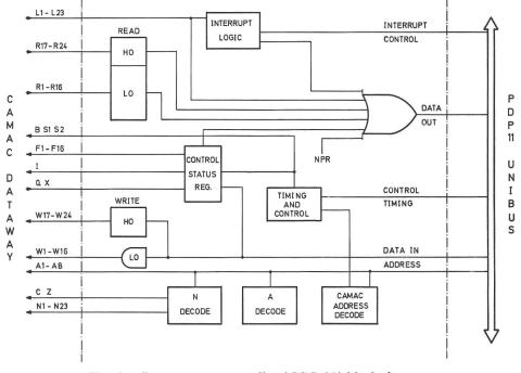
Fig. 1 Crate system controller (CSC 11) block diagram
