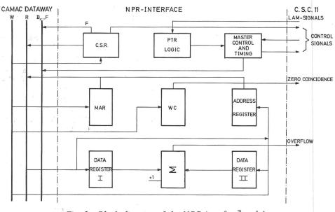
Fig. 2 Block diagram of the NPR interface module
