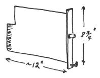
The front panel has a nominal height of  $8\frac{3}{4}$  inch and a single-width is one half the width of a single NIM module—which makes it slightly under 0.7 inch. The length of the circuit board is almost exactly one foot to the end of the edge-connector. As is the case with NIM, modules can come in any multiple of the single-width, with the single and double-widths being especially popular.
