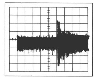
Fig. 2 Pinger pulse superimposed on sea state noise. Horizontal: 100 ms/cm. Vertical: 3.18 µbar (sound pressure)/cm. The latter data are averaged results covering a period of 30 seconds or longer.
