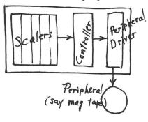
I've shown a one-way-flow from scalers to Controller to peripheral driver to peripheral. Actually, there's a two-way conversation as the Controller issues instructions to the scalers and looks for status information from the various modules.
