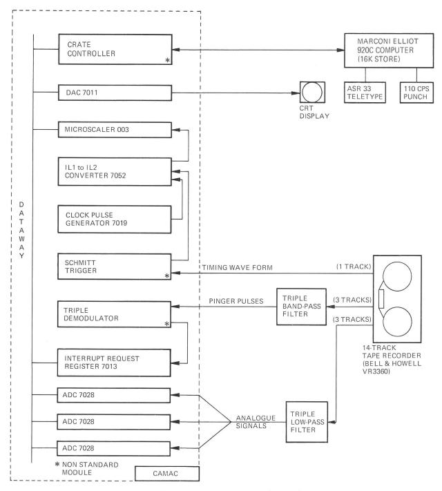
Fig. 1 Computer based sound recording analyser
