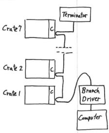
Again we note that the Controller communicates with its own crate and with the Branch Driver and has no interest in the type of computer involved.
