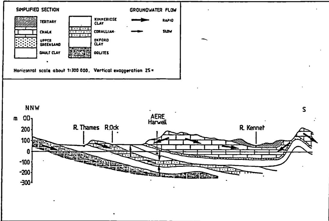
Figure 1. Geological cross-section NNW-SSE through the Harwell site, and conjectured groundwater flow
