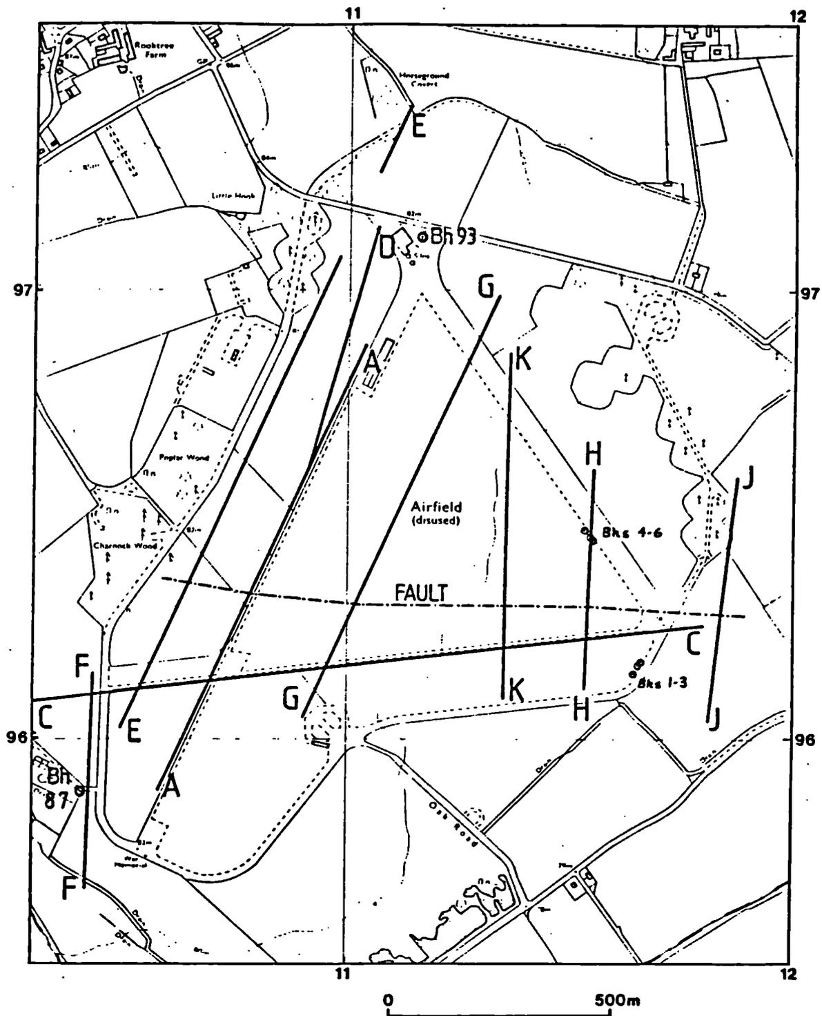
Figure 1. The airfield, boreholes, resistivity traverse lines and the position of the interpreted fault at the Down Ampney site
