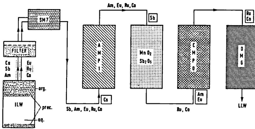
Fig. 1: Flowsheet of the chromatographic decontamination of ILW solutions.
