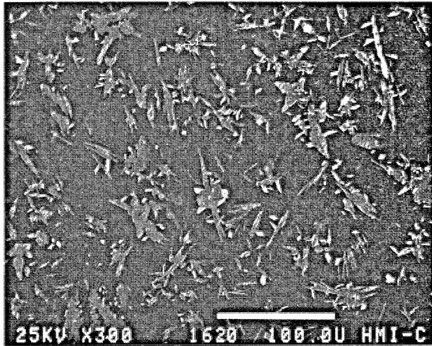
Figure 1 SEM micrograph of HLW glass SM513LW11 annealed at 620°C for 100 days. (White bar = 100 μm)
