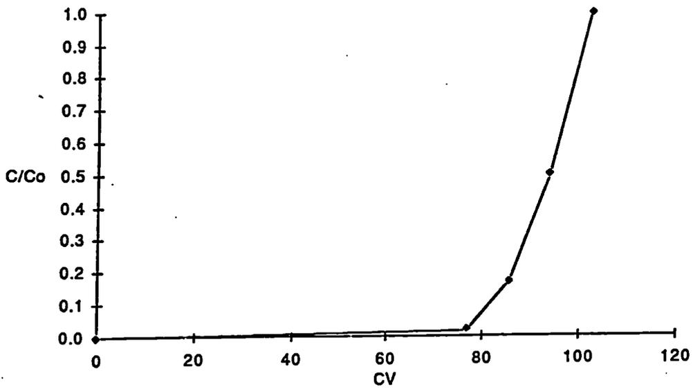
Fig.3 IE-96 Zeolite break-through curve
