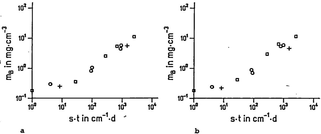
Figure 3. Amount of reacted glass per leachant volume,  $m_B$  (determined by boron analysis of leachate) as a function of  $s \cdot t$  for the corrosion of the HLW glass SON 68 in solution 1 (a) and solution 2 (b) at 190 °C; □ : 30 d; ○ : 120 d; + : HMI test
