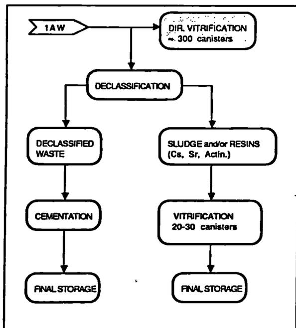
Fig. 1 Conceptual flow-sheet for the management of 1AW-MTR liquid waste
