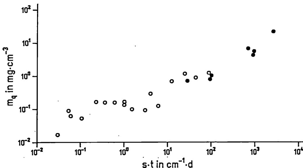
Figure 1. Amount of reacted glass per leachant volume  $m_g$  as a function of the product  $s \cdot t$  for the corrosion of the HLW glass SON 68 in solution 1 at 190 °C;  $s$ : ratio of glass surface area to leachant volume;  $t$ : corrosion time;
