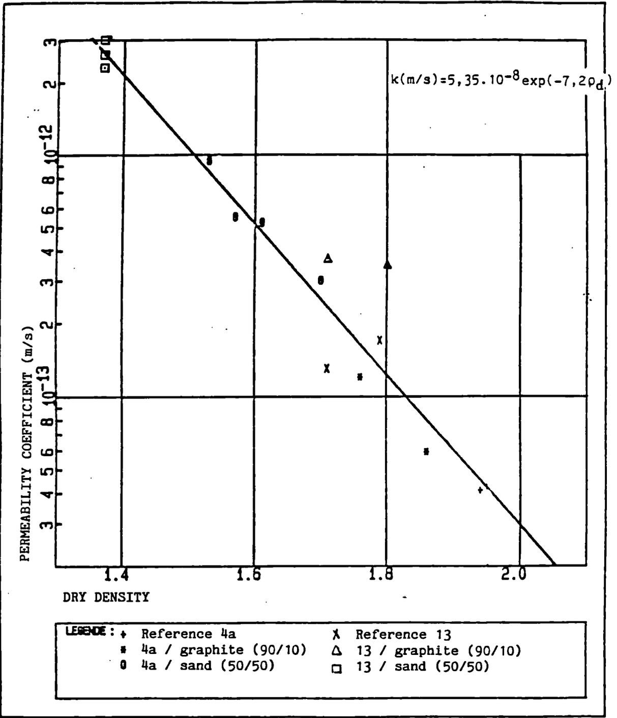
Figure 2 : Permeability coefficient as a function of dry density
