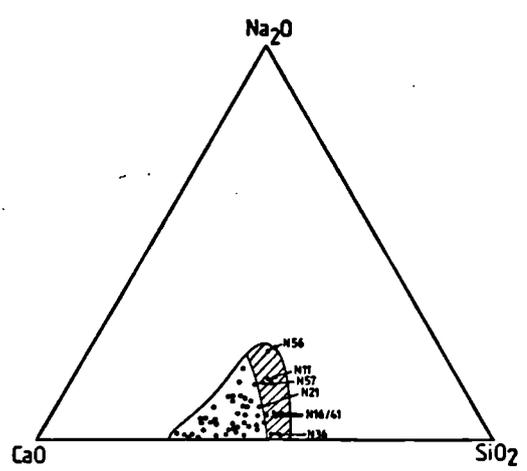
Fig. 4. Anhydrous compositions of representative  $\text{Na}_2\text{O}-\text{CaO}-\text{SiO}_2-\text{H}_2\text{O}$  gels aged up to 182 days.
