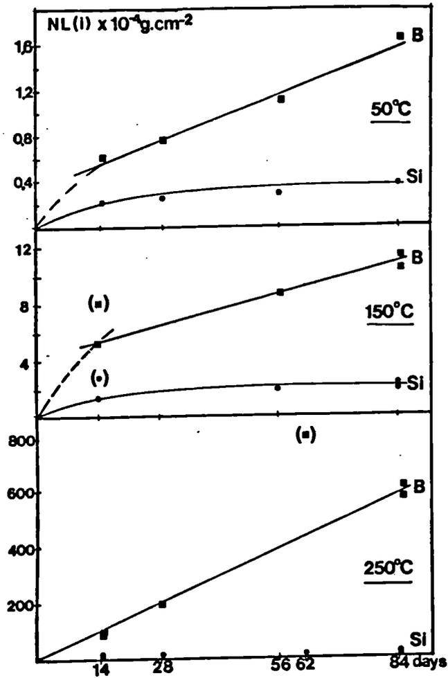
FIGURE 2 : NORMALIZED MASS LOSS FOR BORON AND SILICON AT 50°C, 150°C, AND 250°C
