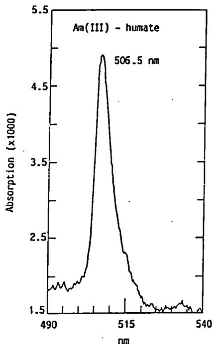
Fig. 3: Absorption spectrum of the Am Humate ( $1.1 \times 10^{-5}$  mol/L Am) in 0.1 M  $\text{NaClO}_4$  (pH 9.2; 10mg/L HA)
