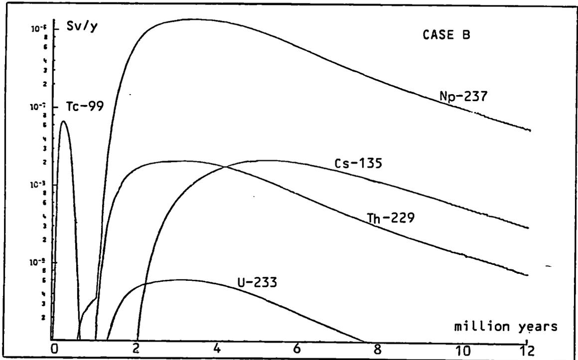
Figure 3 - Individual dose rate as function of the time (United Kingdom site, main discharge zone and disposal concepts A and B)
