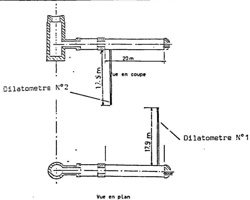
Fig. 1 : SITUATION OF THE DILATOMETER CREEP TEST
