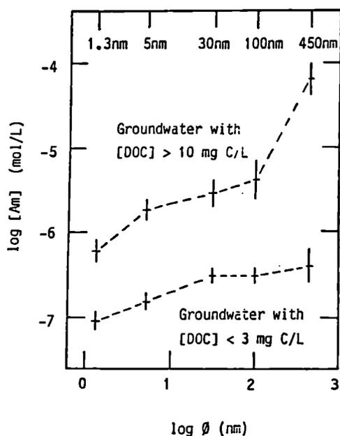
Fig. 1: Ultrafiltration of Am(III) humic colloids in groundwaters with different DOC concentrations. The Am(III) concentration in filtrate varies with filter pore size.
