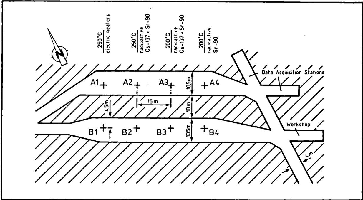
Figure 1: HAW Test Field at the Asse Salt Mine
