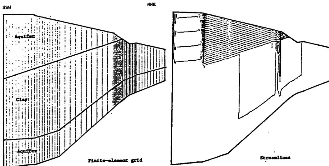
Figure 2. Groundwater-flow calculations for an improved finite-element grid
