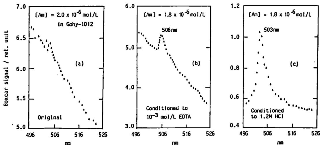
Fig. 4: Photoacoustic spectra of the Am(III) pseudocolloids (humic colloids) in the Gohy-1012 groundwater (a), the Am(III)-EDTA complex (b) and the  $\text{Am}^{3+}$  ion (c). The latter two spectra are taken after conditioning of colloids for 6 months in EDTA or HCl.
