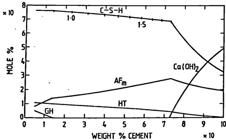
Fig. 2. Phase distribution in slag-cements
