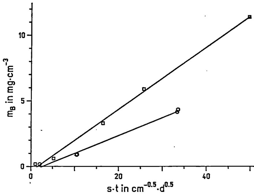
Figure 2. Amount of reacted glass per leachant volume,  $m_B$  (determined by boron analysis of leachate) as a function of  $\sqrt{s \cdot t}$  for the corrosion of the HLW glass SON 68 in solution 3 at 150 °C; □ : 30 d; ○ : 120 d
