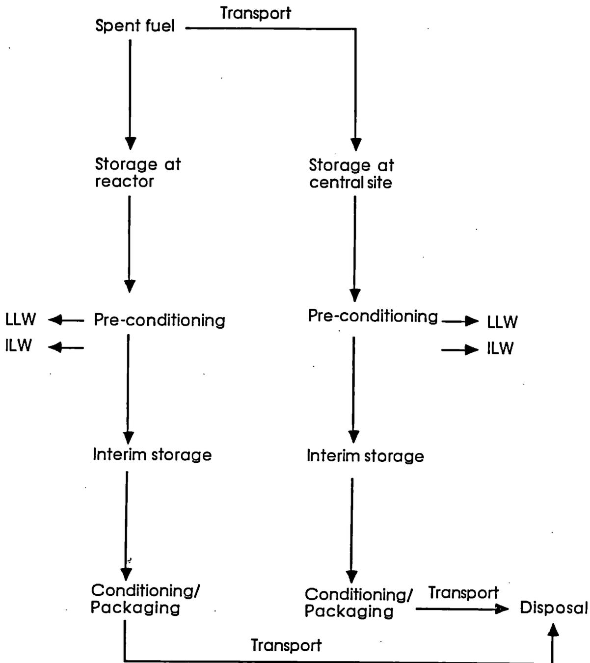
Figure 1 Schematic diagram of direct disposal options
