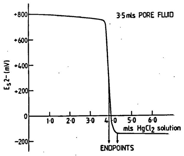
Fig. 5. Typical titration curve for aqueous sulphide determination.
