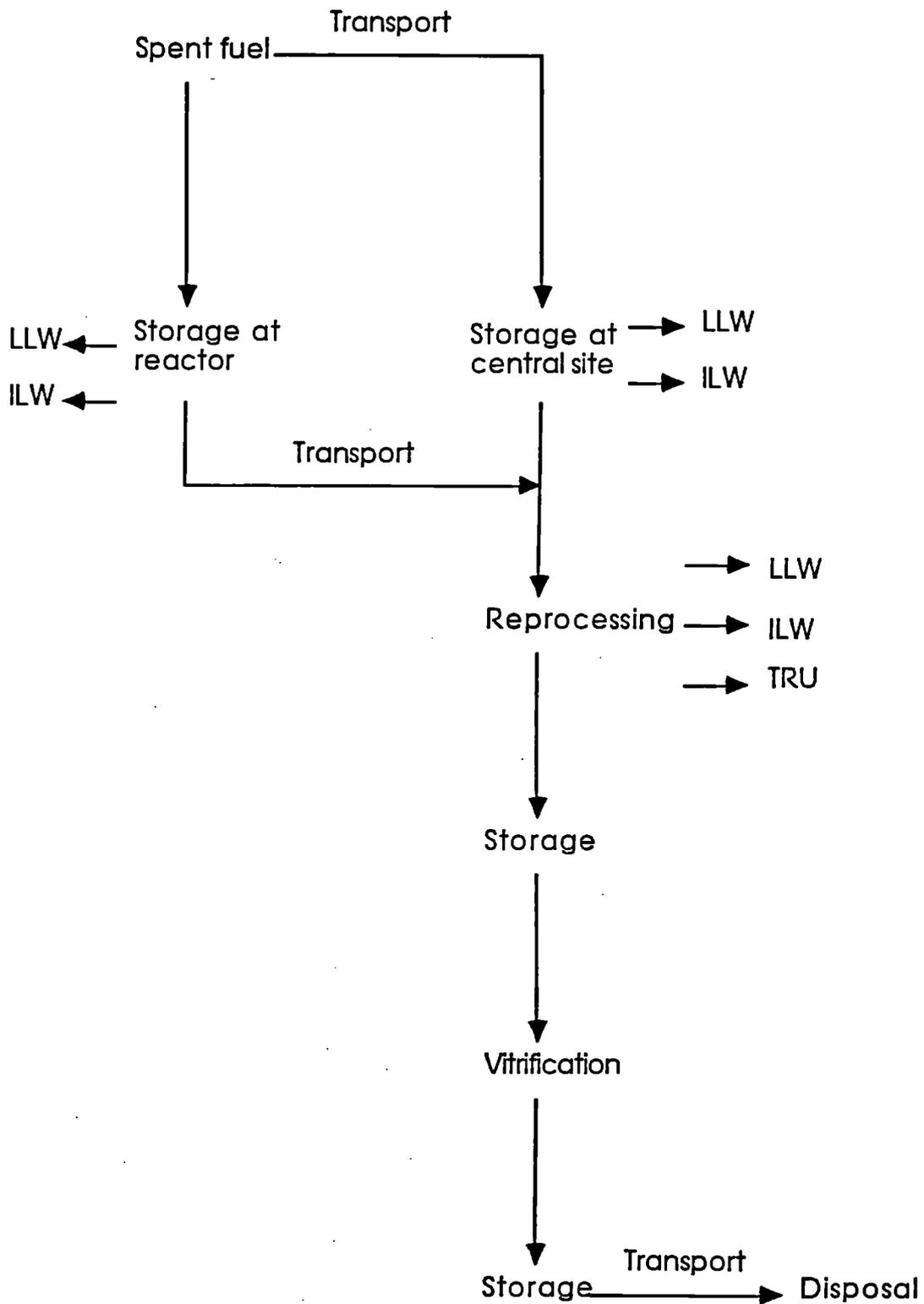
Figure 2 Schematic diagram of reprocessing options
