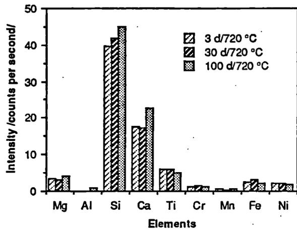
Figure 2b X-ray intensities of elements from SEM-EDS analysis of the annealed HLW glass SM513LW11. Annealing times: 3, 30 and 100 days. Annealing temperatures: 620, 720 and 820 °C. From analysis of the large, dark crystals in Figure 1.
