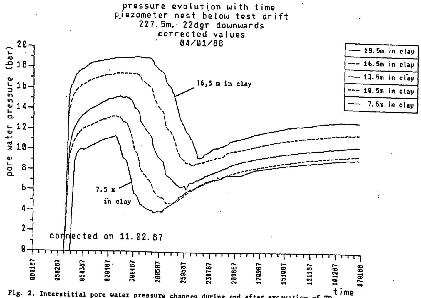
Fig. 2. Interstitial pore water pressure changes during and after excavation of TD
