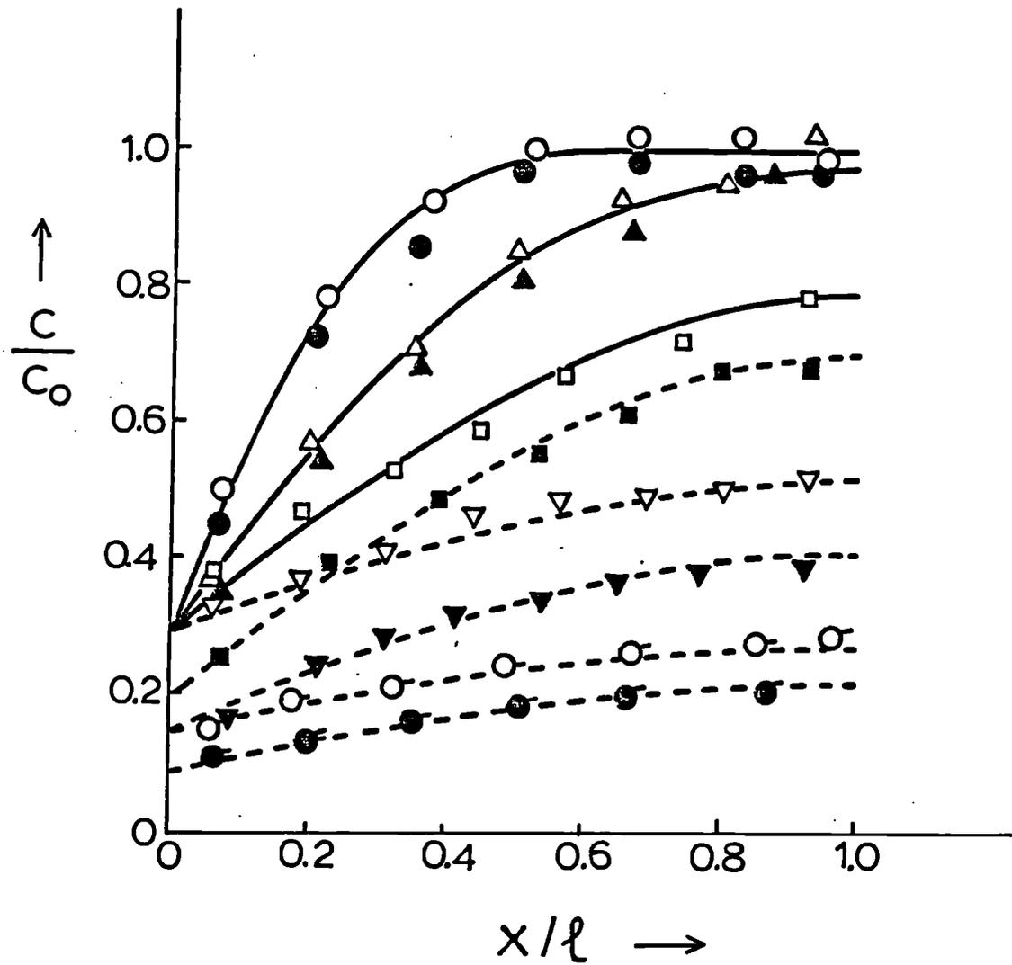
Figure 2. Distribution of Cs in cement samples after 6 (o,●), 21 (Δ,▲), 57 (□,■), 114 (▽,▼) or 174 (σ,σ) days of elution at 70°C. Amounts eluted (%): 10.2 (o), 11.5 (●), 22.1 (Δ), 24.0 (▲), 37.1 (□), 45.0 (■), 54.5 (▽), 65.0 (▼), 76.0 (σ) or 82.0 (σ). The theoretical concentration profiles correspond to  $D=7.5 \times 10^{-7} \text{ cm}^2 \text{ s}^{-1}$  (—) or  $8.9 \times 10^{-7} \text{ cm}^2 \text{ s}^{-1}$  (---) and  $C_1/C_0=0.30$  (o,●,Δ,▲,□,▽), 0.20 (■), 0.15 (▼,σ), 0.09 (σ).
