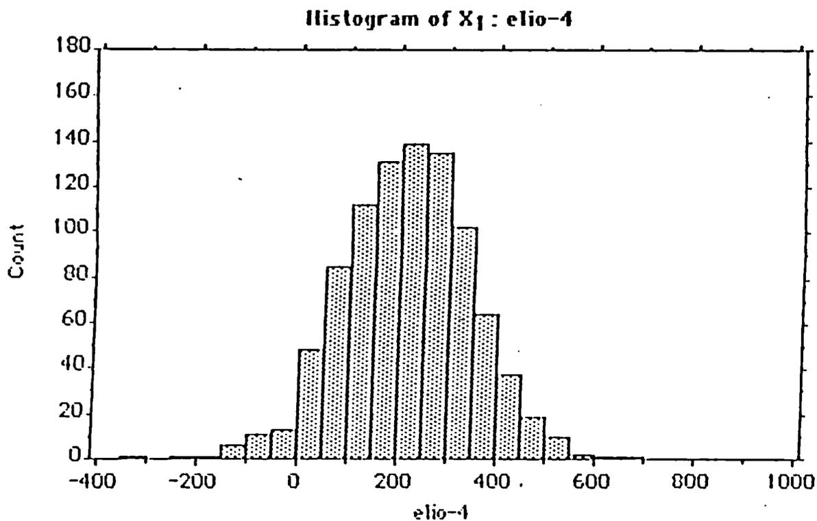
FIG. 1 - Frequency histogram of helium contents, expressed as differences (ppb) with regard to helium content in the atmosphere. The values are homogeneously distributed. Most of them furthermore display weak enrichment with regard to the helium concentration in the atmosphere ( zero reference ).
