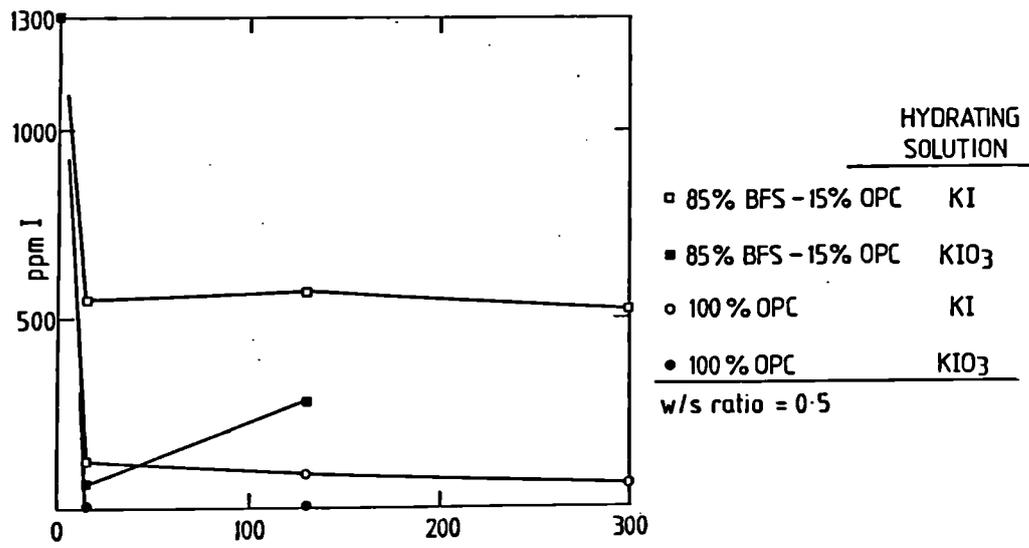
Fig. 8. Sorption of  $I^-$  and  $IO_3^-$  in cement and slag-cement pastes..
