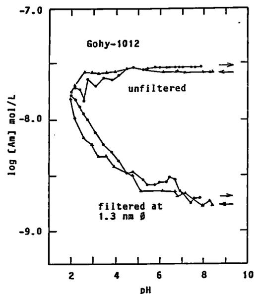
Fig. 2: Generation of Am(III) pseudo-colloids (humic colloids) in the Gohy-1012 groundwater by dissolving the Am hydroxide precipitate and diluting it with the fresh groundwater. The pH titration is made from pH = 8.4 to 2.0 and back titrated. The Am concentration is determined in unfiltered solutions and filtrates at 1.3 nm pore size.
