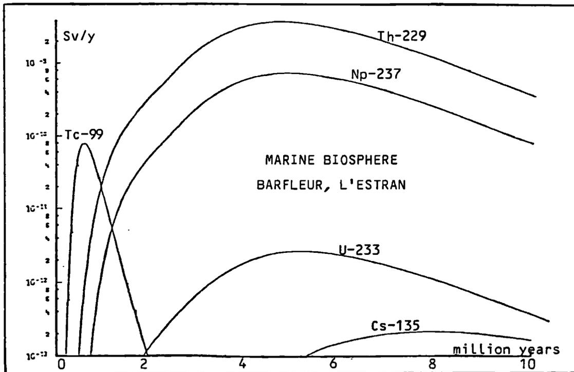
Figure 4 - Individual dose rate as function of the time at the Barfleur site for the two discharge zones and the diposal concept A.
