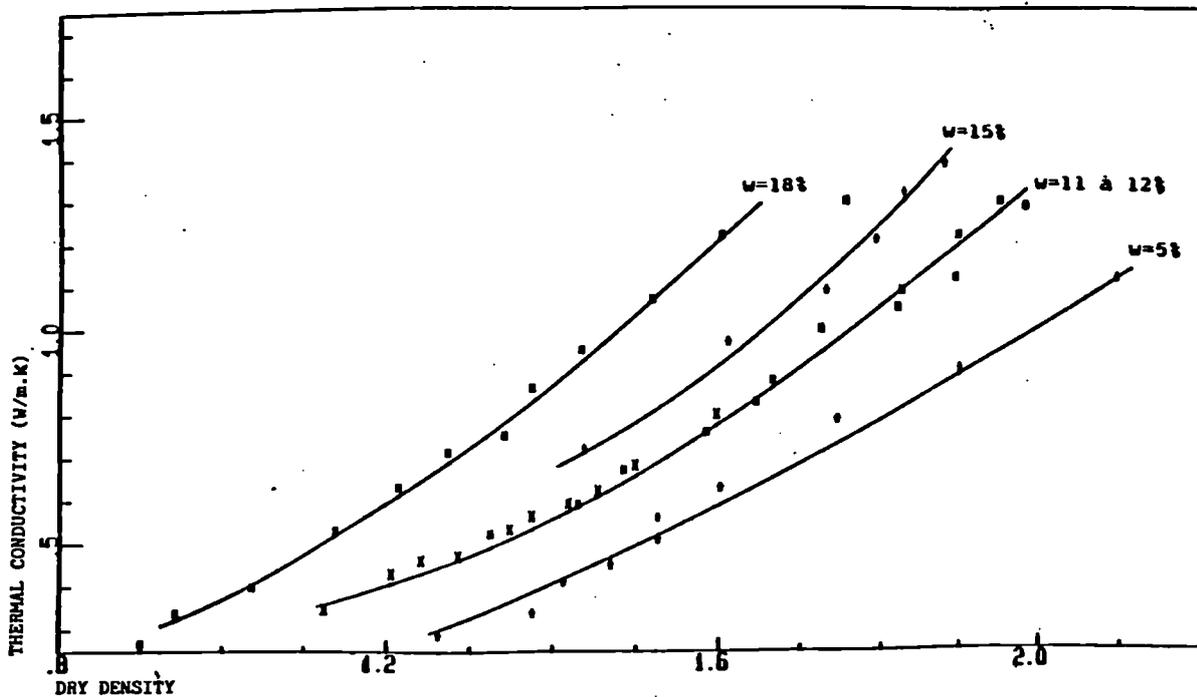
Figure 1 : Thermal conductivity as a function of dry density for reference 4a (20°C) (w = Water content)
