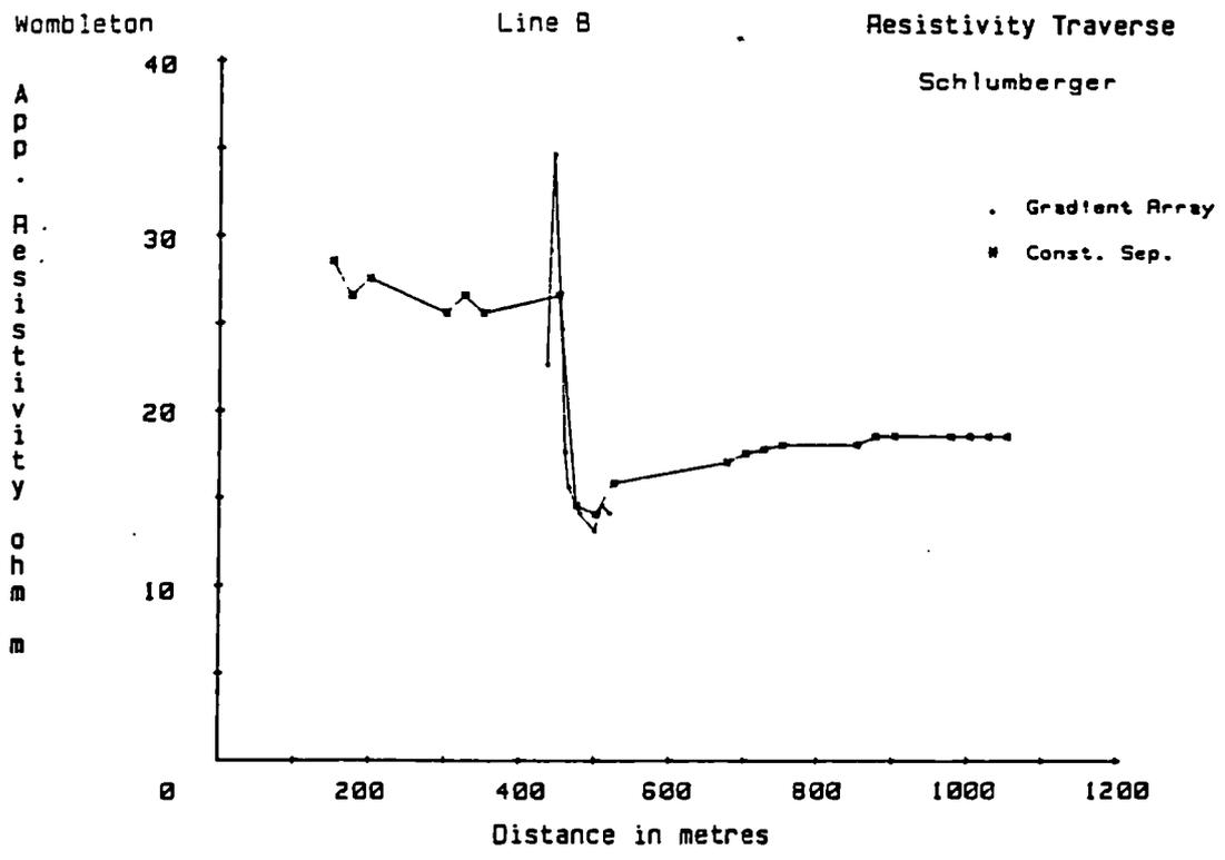
Figure 3 Resistivity traverse along Line B.
