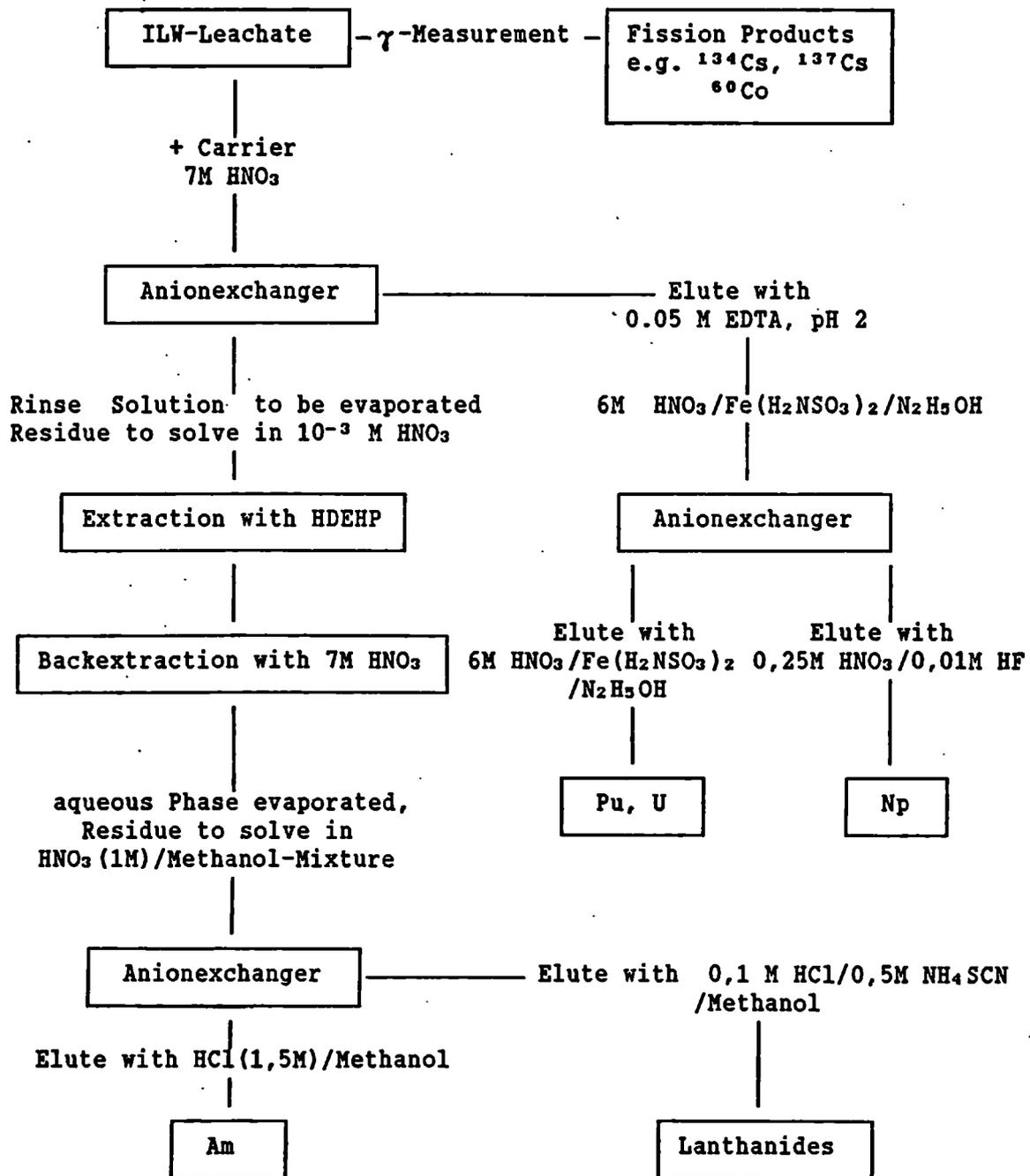
Figure 1. Chemical Procedure for the Separation of Actinides from real waste leachates
