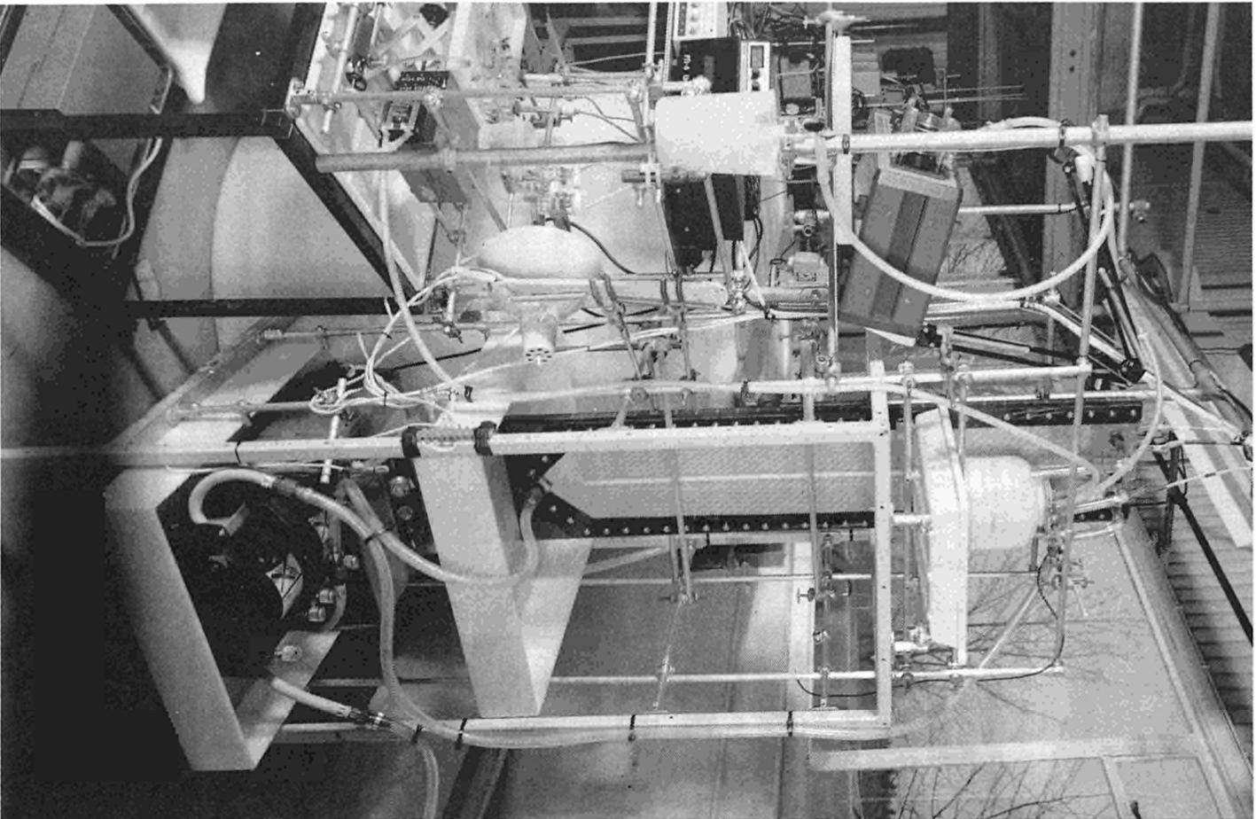
Figure 2 0.1 m<sup>3</sup>/h EIX treatment cell.
