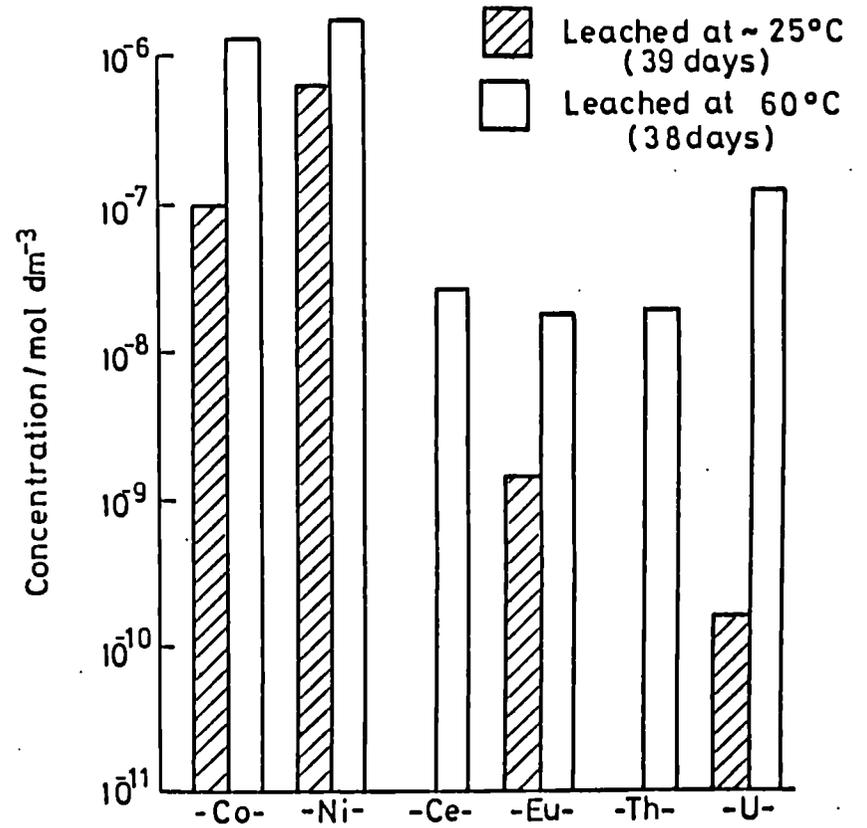
FIGURE 2. CONCENTRATIONS OF SPIKE ELEMENTS LEACHED FROM OPC AT ~25°C AND 60°C AFTER ~38 DAYS AS DETERMINED BY ICP-MS
