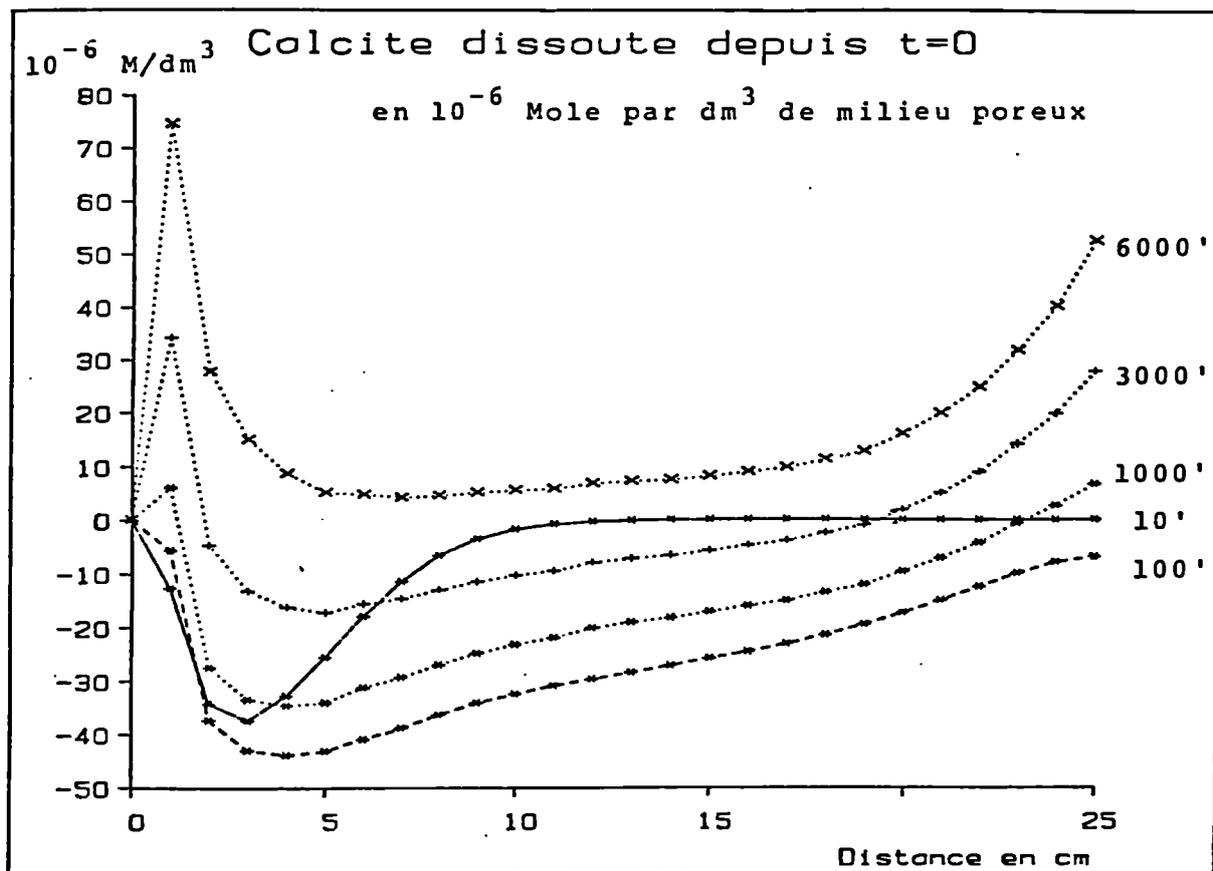
Figure 1 : Balance of dissolved calcite (>0)
