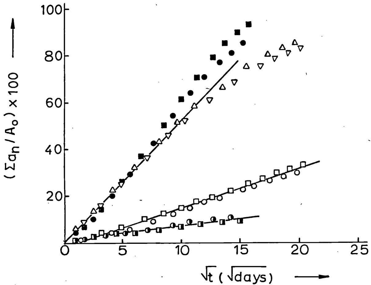
Figure 1. Elution curves of Cs from duplicate cemented specimens containing inactive  $\text{Cs}_2\text{SO}_4$  (3.4% wt) at  $70^\circ$  (Series B; ●, ■) or  $30^\circ\text{C}$  (Series A,C; ○, □, ∇, Δ) or Cs-137 (10  $\mu\text{Ci}/\text{sample}$ ),  $\text{CsNO}_3$  (0.017% wt) and  $\text{NaNO}_3$  (8% wt) at  $30^\circ\text{C}$  (Series D; ○, ■). Sample thicknesses: 1.2 cm (Series C; ∇, Δ) or 4.0 cm (Series A,B,D; ○, □, ●, ■, ○, ■).
