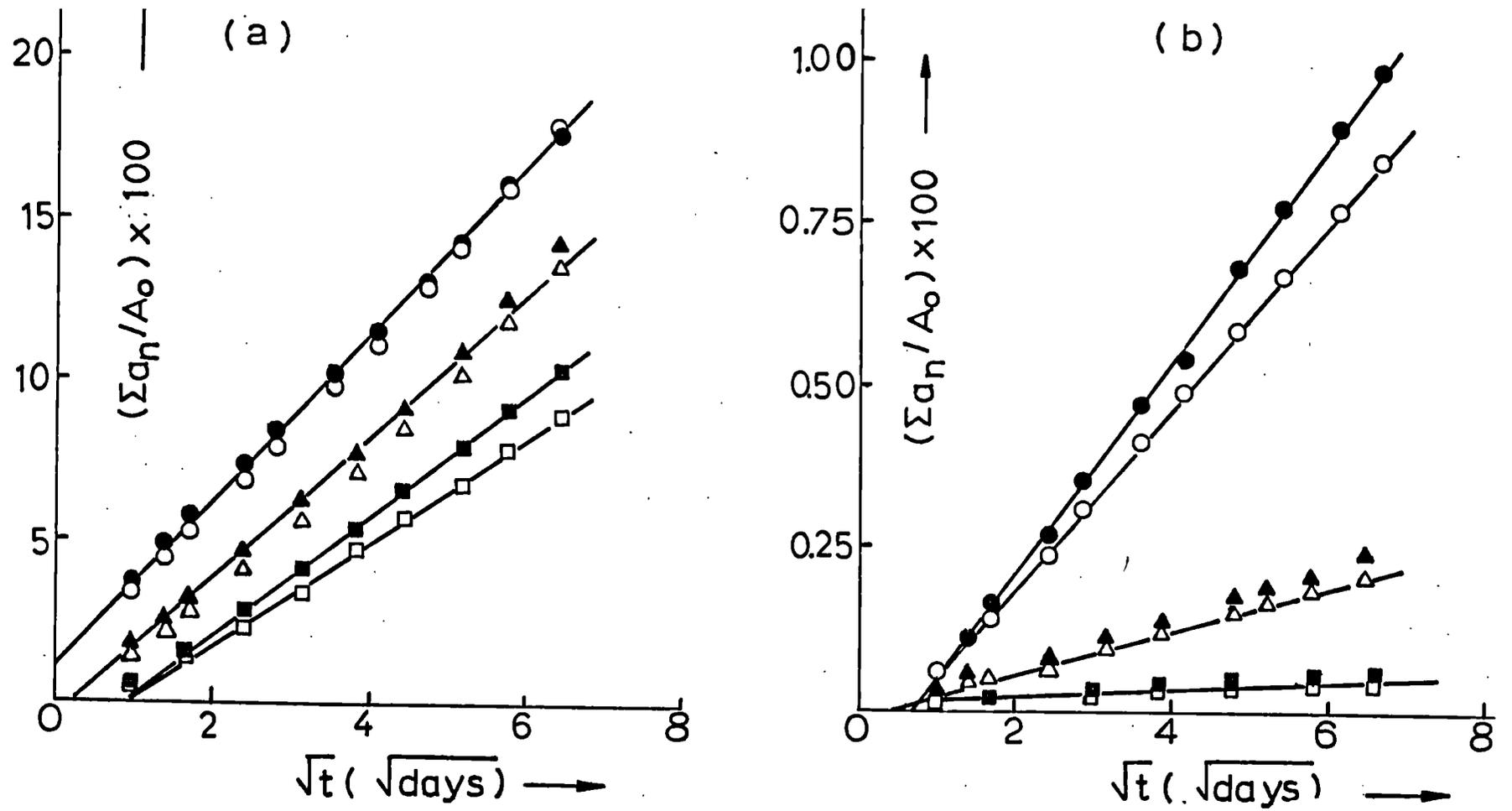
Figure 3. Elution curves at 30°C of (a) NaCl or (b) SrSO<sub>4</sub> from duplicate specimens (~7 mm thick) of salt-loaded epoxy resin. Salt content (% vol): 12 (□, ■), 25 (Δ, ▲), 40 (○, ●).
