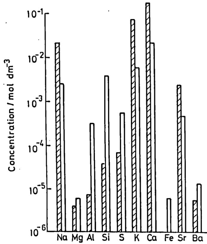
FIGURE 1. CONCENTRATIONS OF ELEMENTS LEACHED FROM OPC AT ~25°C AND 60°C AFTER ~38 DAYS AS DETERMINED BY ICP- OES
