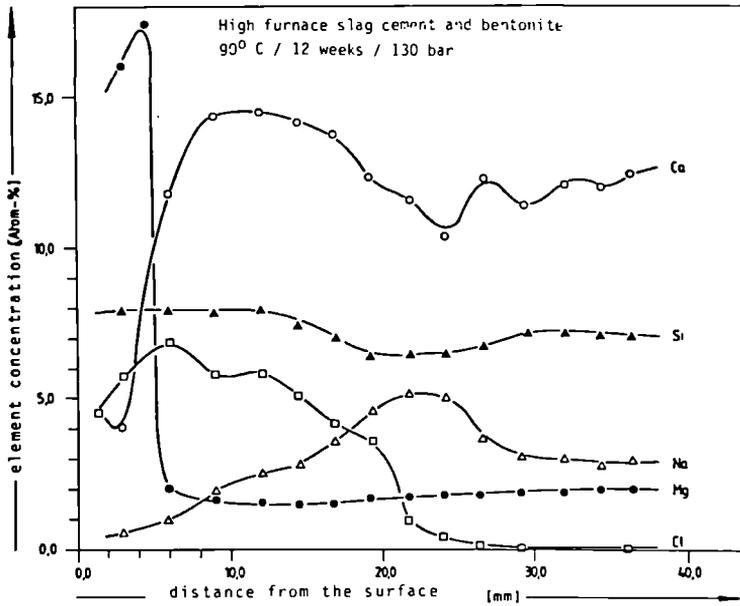
Fig. 7 : Depth-Concentration profiles of selected elements in cement samples from one dimensional corrosion experiments in quinary salt brine at 90° C and 130 bars after 12 weeks duration (high furnace slag cement, w/c-ratio = 0.4, 10 weight %  $\text{NaNO}_3$ , 5 weight % bentonite).
