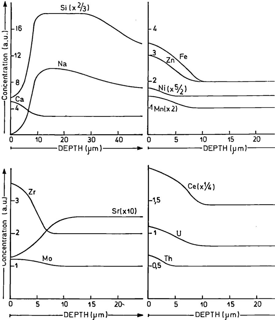
Fig. 26 : Elemental concentration profiles determined in the near surface region of glass sample SON 68 18 17 leached at 90° C during 14 days in deionized water ( $SA/V = 0.5 \text{ cm}^{-1}$ ), using nuclear micro-probe.
