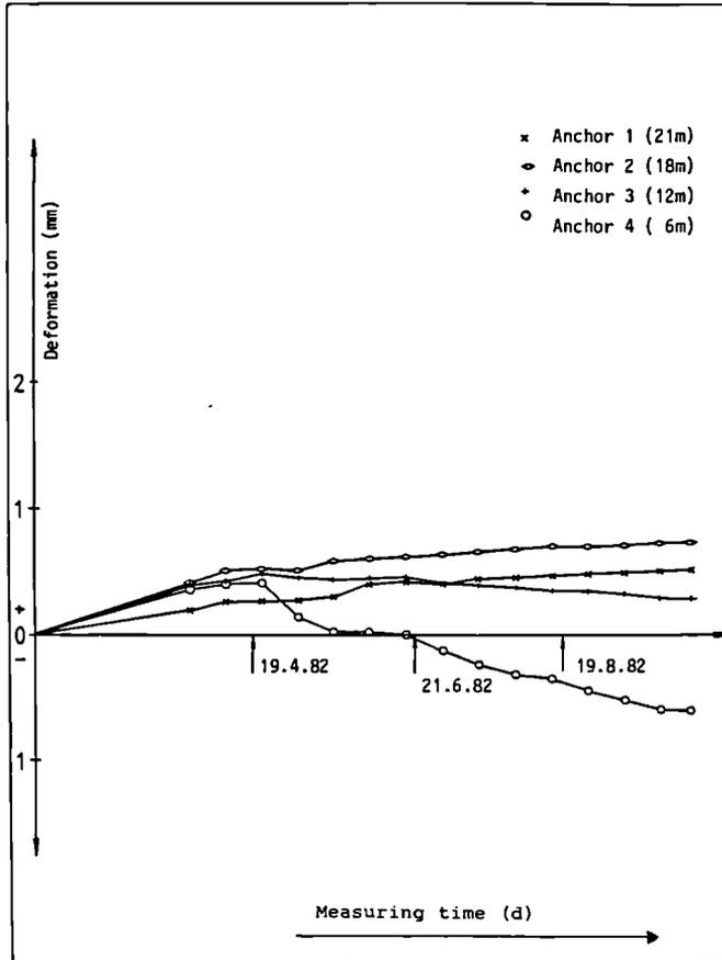
Fig. 54 : Temperature test 5; Deformation/Time diagram of extensometer SE3
