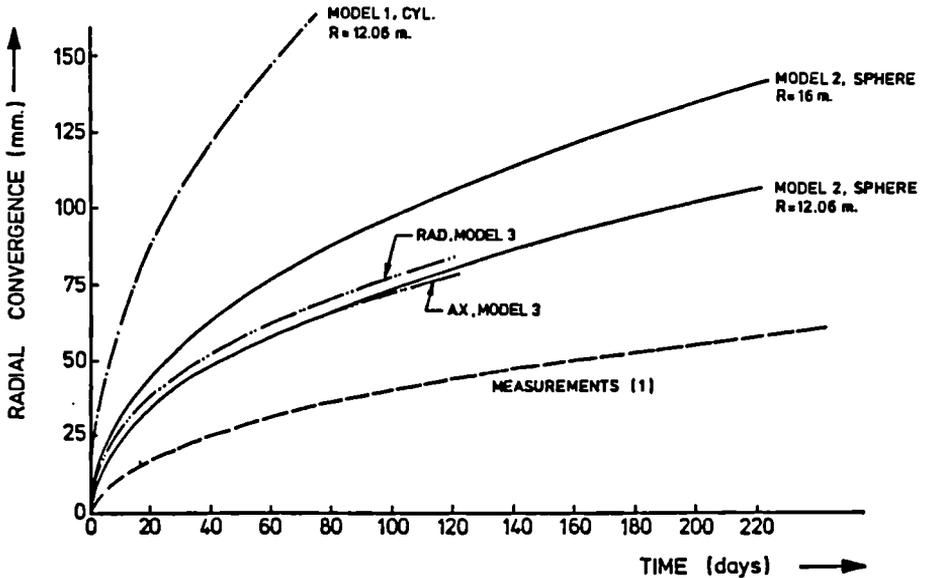
Fig. 90 : Calculated vs. measured radial convergence of the prototype cavern.
