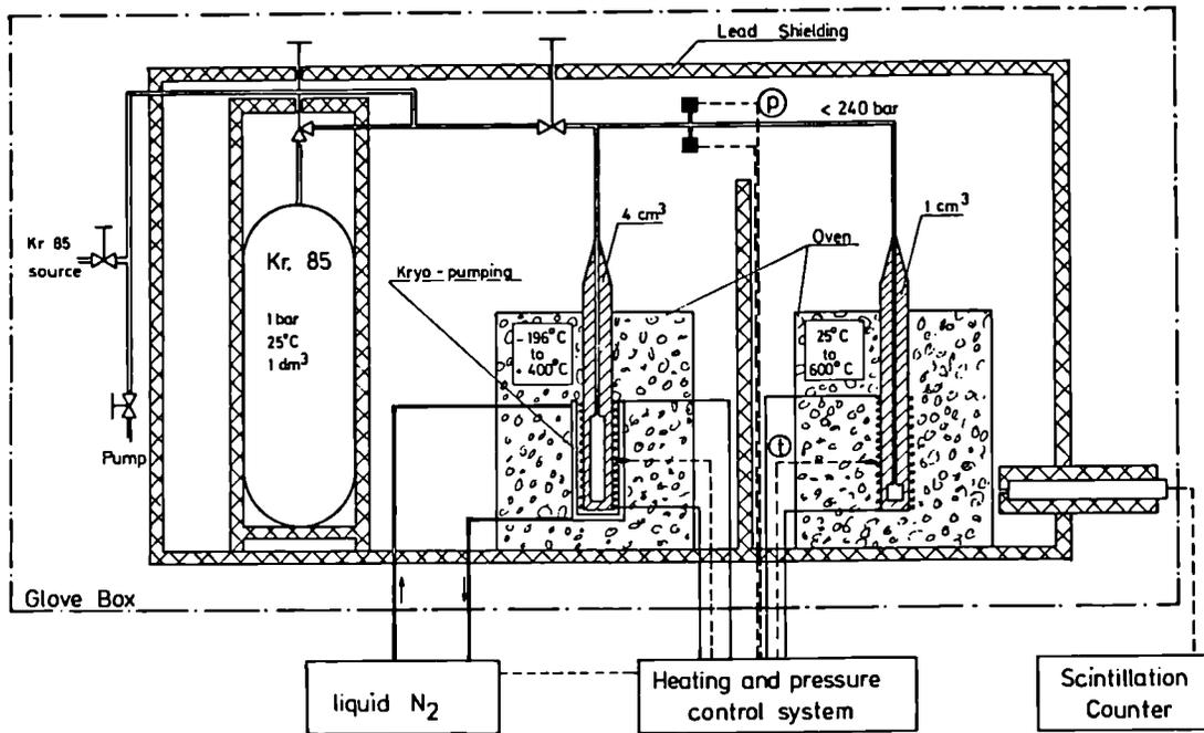
Fig. 37 : Small scale test facility for the fixation of radioactive krypton in zeolite
