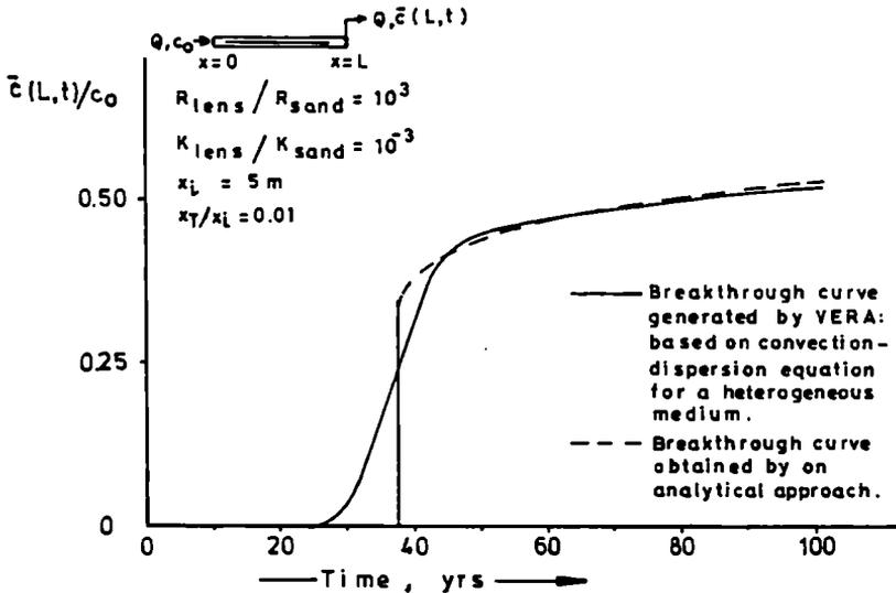
Fig. 47 : Breakthrough curve of one-lens-system
