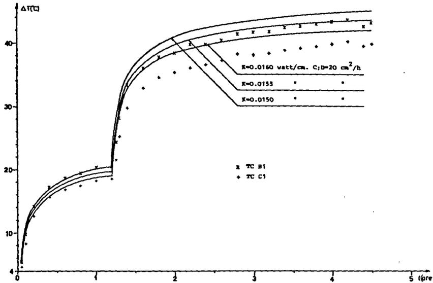
Fig. 76 : Theoretical and experimental temperature increases 50 cm fareway from the heater axis against time. Thermocouple B1 has recorded the maximum temperature increase, while thermocouple C1 has recorded the minimum one.
