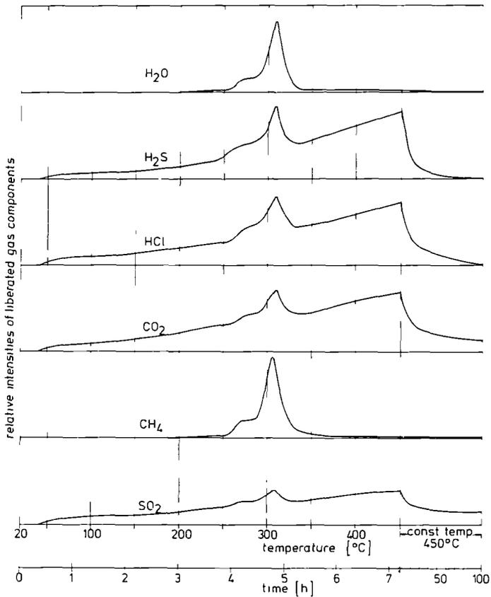
Fig. 53 : Liberation of the gas components H<sub>2</sub>S, HCl, CO<sub>2</sub>, CH<sub>4</sub>, H<sub>2</sub>O and SO<sub>2</sub> versus temperature and time. Mineralogical composition : 73.4 wt% Halite, 20.5 % Polyhalite, 5.2 wt% Anhydrite. Total gas content : 4.3 ppm H<sub>2</sub>S, 20 ppm HCl, 183 ppm CO<sub>2</sub>, 35 ppm Hydrocarbons, 1.26 wt% H<sub>2</sub>O, amount of SO<sub>2</sub> not measurable.
