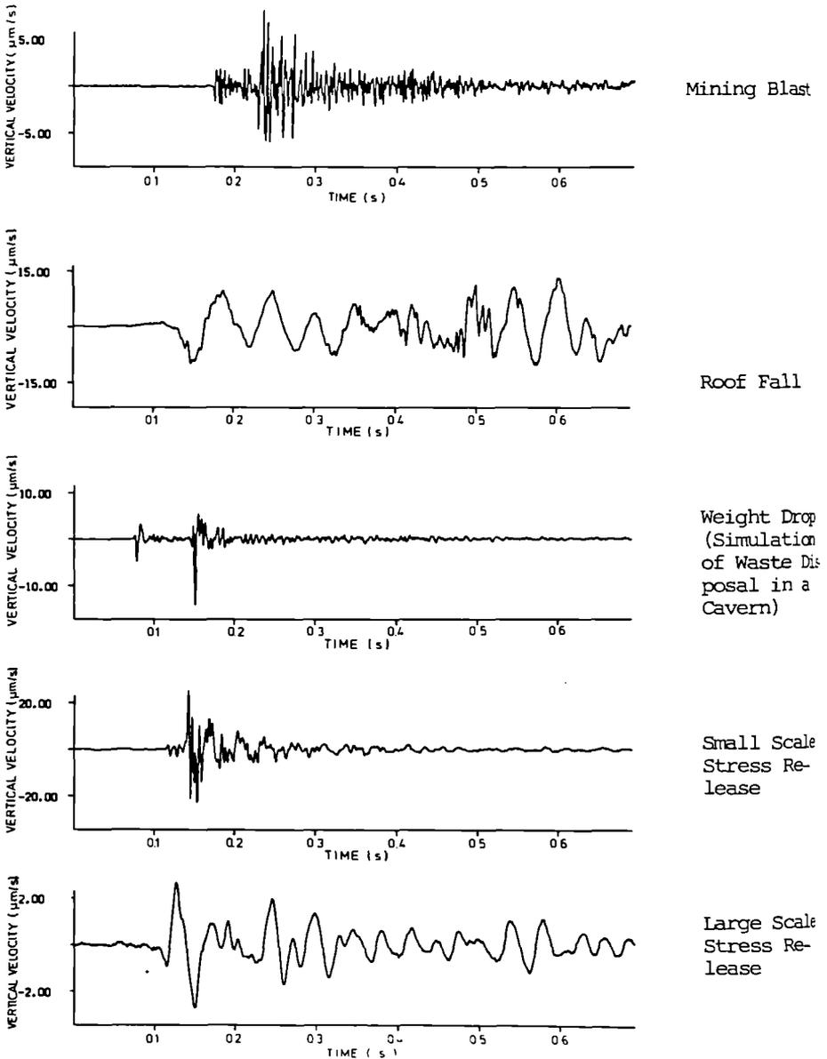
Fig. 57 : Examples of different types of seismic events
