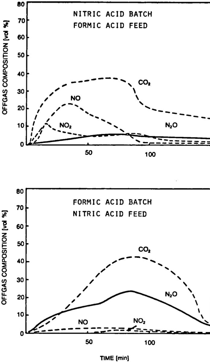
Fig. 19 : Off gas composition for two dinitration procedures of MAW concentrate
