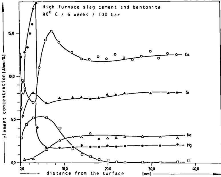
Fig. 6 : Depth-Concentration profiles of selected elements in cement samples from one dimensional corrosion experiments in quinary brine at 90° C and 130 bars after 6 weeks duration (high furnace slag cement, w/c-ratio = 0.4, 10 weight %  $\text{NaNO}_3$ , 5 weight % bentonite).
