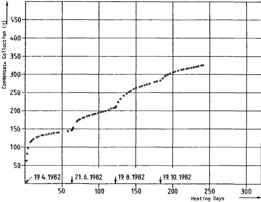
Fig. 52 : Temperature test 5 - Time and temperature dependent water release
