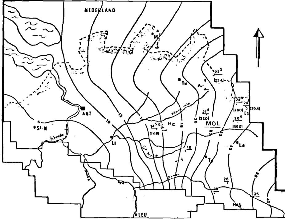
Fig. 50 : Simulation of the Berg sands aquifer
