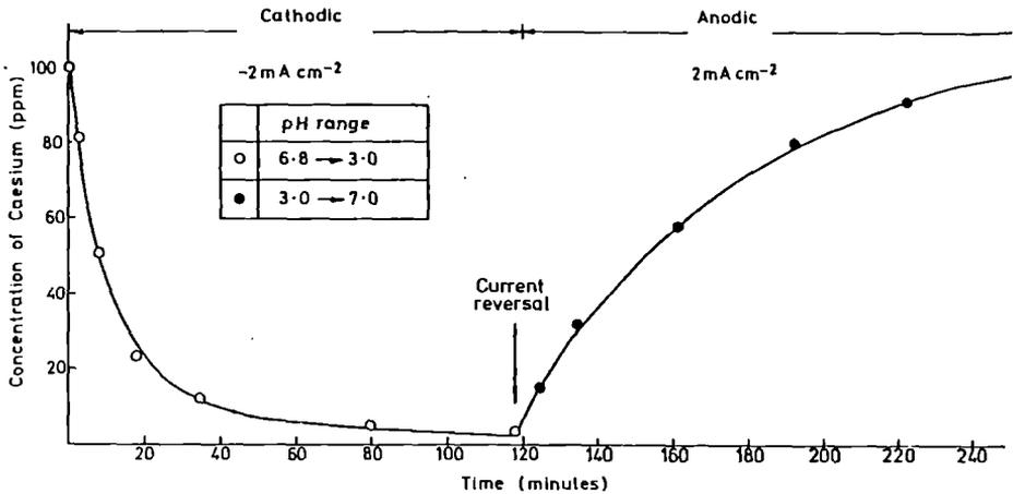
.Fig. 20 : Adsorption of caesium onto an amberlite CG50/Kraton/ Graphite electrode (2nd cycle) from a Cs NO<sub>3</sub> electrolyte
