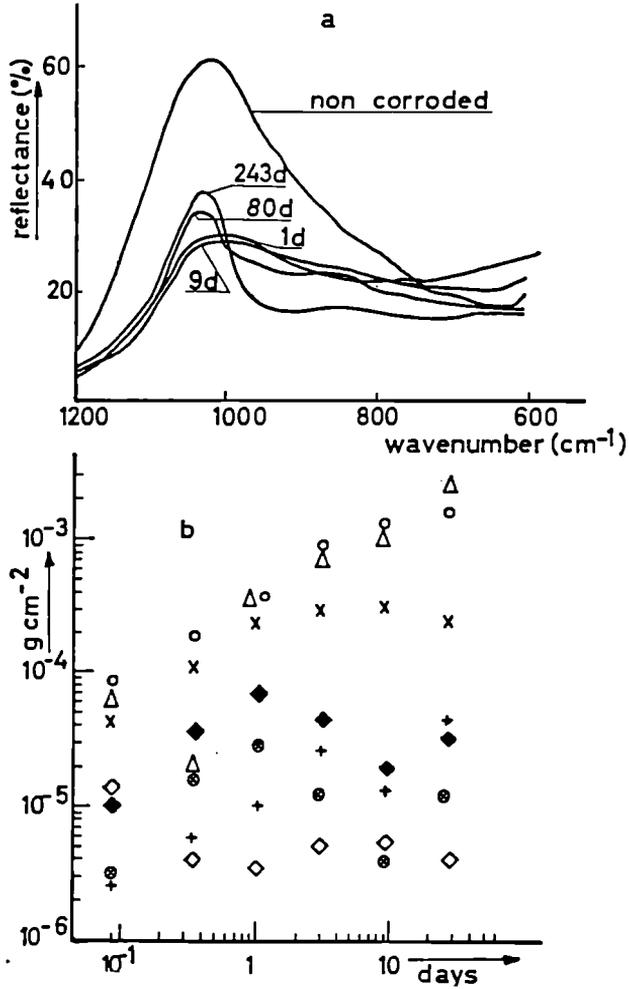
Fig. 27 : SON641920F<sub>3</sub>; IRR spectra (a) and NSWL (b) as a function of the corrosion time ( $\text{H}_2\text{O}$ ,  $90^\circ \text{C}$ ,  $1 \text{ cm}^{-1}$ )
