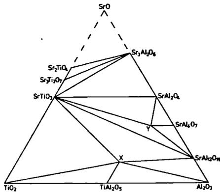
Fig. 32 : Composition diagram of the system SrO-TiO<sub>2</sub>-Al<sub>2</sub>O<sub>3</sub> at 1300° C.
