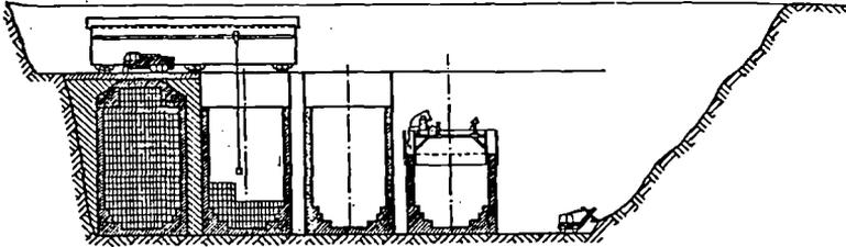
Fig. 46 : Vertical section of burial site with waste units during various stages of manufacture and loading
