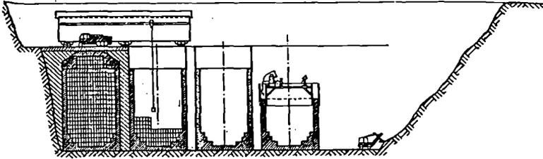
Fig. 46 : Vertical section of burial site with waste units during various stages of manufacture and loading
