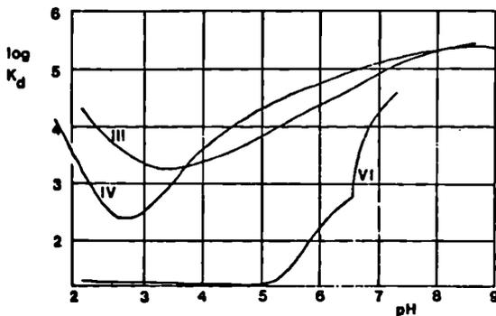
Fig. 87 : Plutonium retention by bentonite versus pH, for valencies III,
