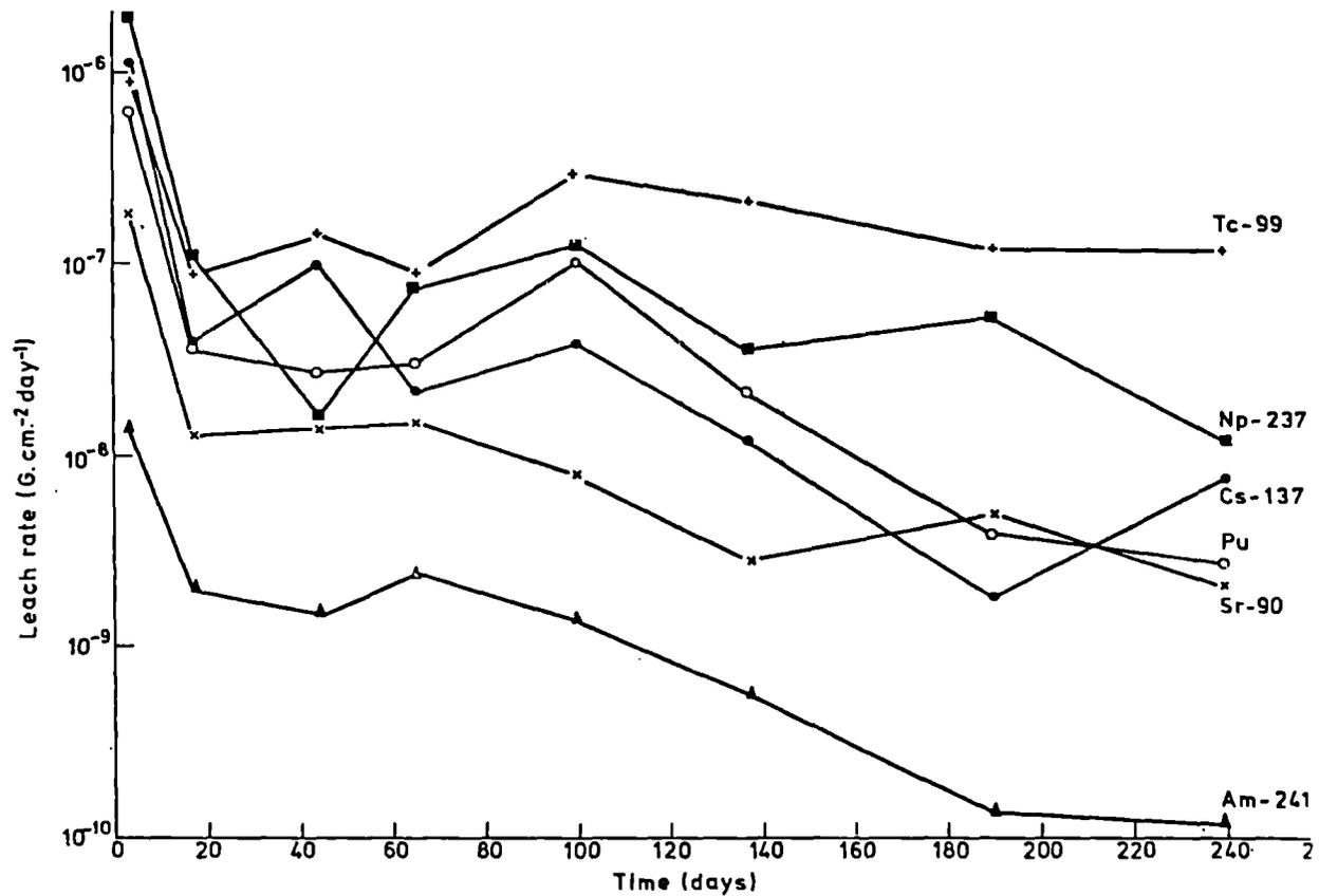
Fig. 30 : Leach rate of UK209 at 60° C in repository simulation
