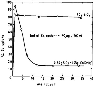
Fig. 9 : The effect of  $\text{Ca}(\text{OH})_2$  on the  $\text{SiO}_2/\text{Cs}$  interaction
