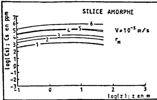
Fig. 83 : Precipitated mass ( $C_g$ ) per unit of fracture volume versus the distance  $z$  from the heat source for the kinetic constant  $r_M$  and the fluid velocity  $V$ .
