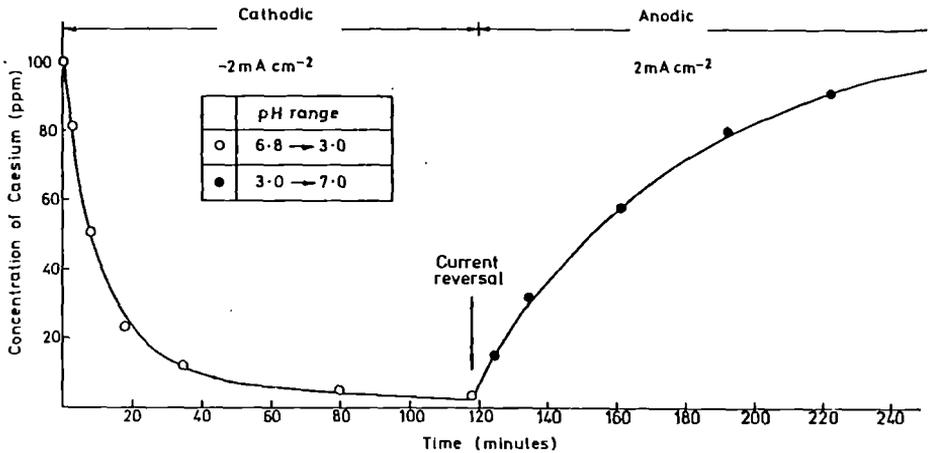
.Fig. 20 : Adsorption of caesium onto an amberlite CG50/Kraton/ Graphite electrode (2nd cycle) from a  $\text{Cs NO}_3$  electrolyte
