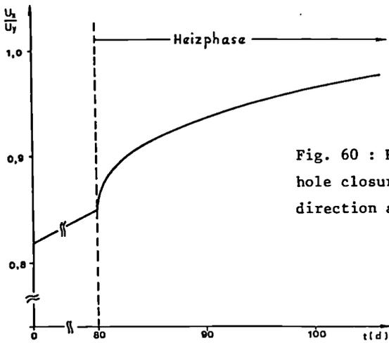
Fig. 60 : Ratio between borehole closure in X- and Y-direction as a function of time
