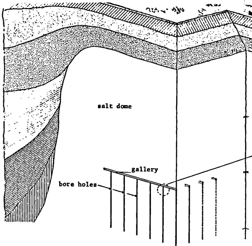
Fig. 91 : Salt dome with disposal holes
