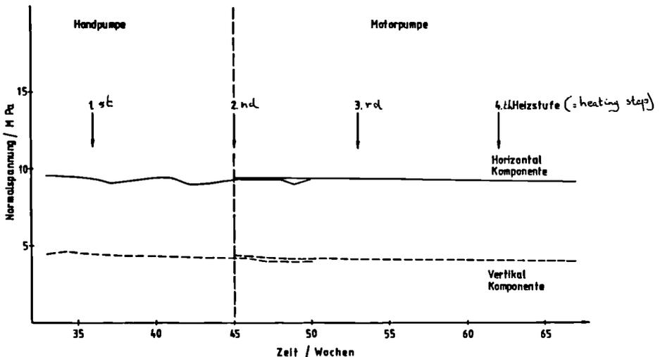
Fig. 55 : Measured stress versus time including the transition from hand pump to motor pump
