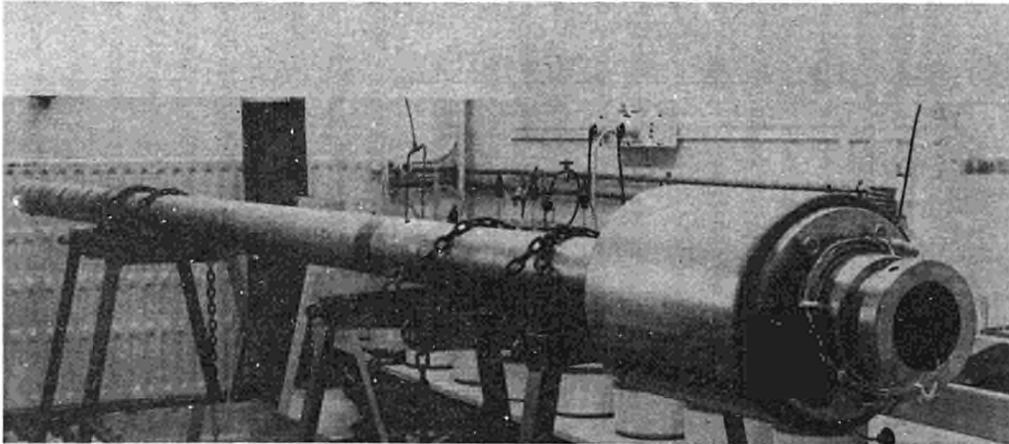
Fig. 66 : Photography of prototype loop system for "in situ" testing of candidate canister materials in direct contact with clay
