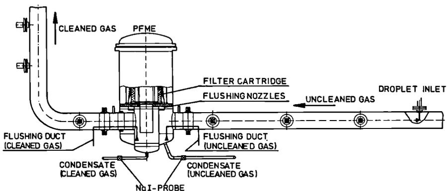
Fig. 40 : Test procedure for the investigation of loading and cleaning
