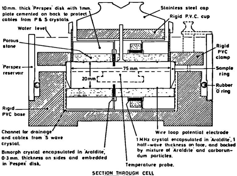
Fig 9. The modified consolidation cell
