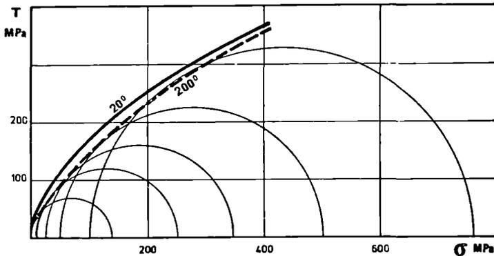
Fig. 80 : Mohr's envelopes of Auriat granite at  $20^{\circ}$  and  $200^{\circ}\text{C}$ .
