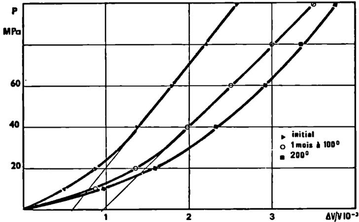
Fig. 79 : Compressibility of Auriat granite under triaxial load
