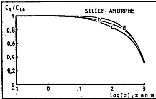
Fig. 82 : Silica concentration  $C_L$  versus the distance  $z$  from the heat source.  $C_{L0}$  : imposed concentration in  $z = 0$ . b,c,d curves for temperature fields of 50, 100 and 1000 years
