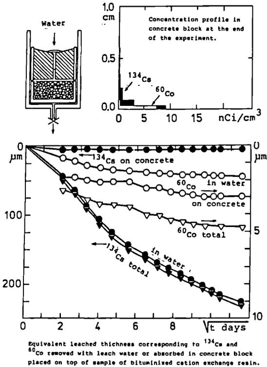
Fig. 10 :  $^{134}\text{Cs}$  and  $^{60}\text{Co}$  removed with leach water or transferred to a concrete block placed on top of a sample of bituminized cation exchange resin.
