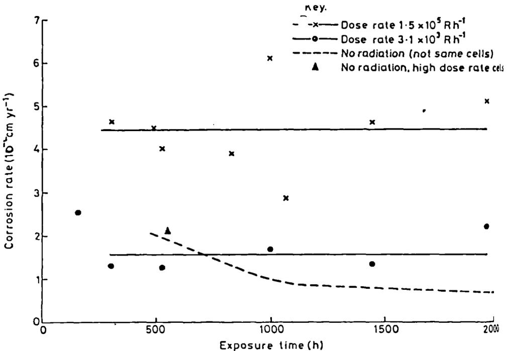
Fig. 67 : Corrosion rate vs exposure time. Influence of radiolysis. Forged steel specimens immersed in de-aerated substitute sea water at 90° C under an argon blanket
