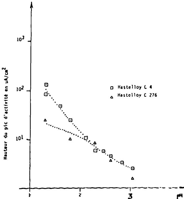
Fig. 71 : Comparison of peak-activity versus pH curves for Hastelloy C4 and C276 (sensitivity to corrosion by crevices)
