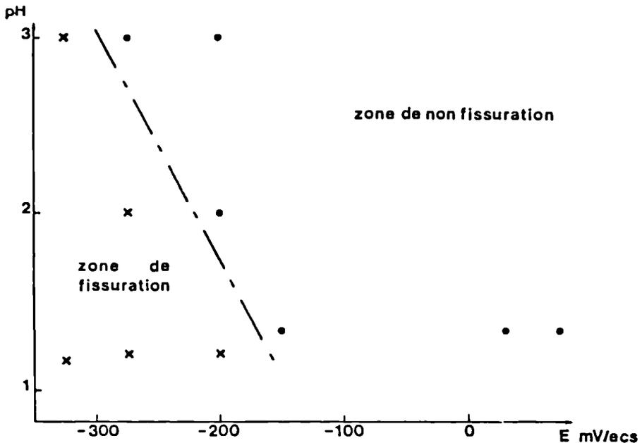
Fig. 70 : Alloy 625, corrosion susceptibility under stress as a function of stress and electrode potential in granitic water nr 1.
