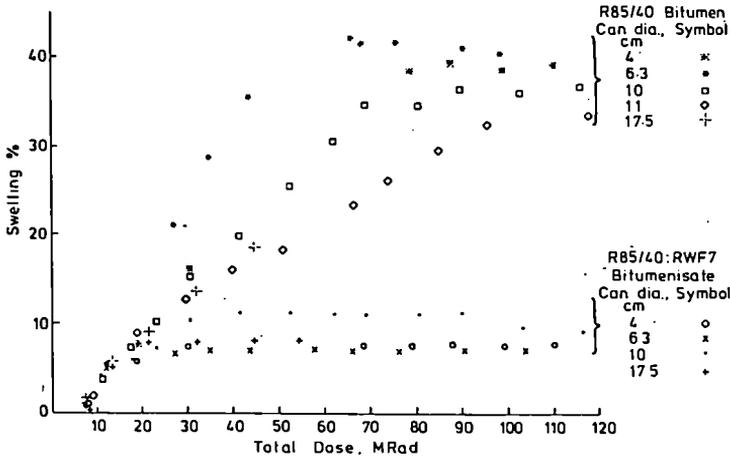
Fig. 4 : Radiation induced swelling of unfilled bitumen R85/40 and bitumenisate simulated waste form RWF7.
