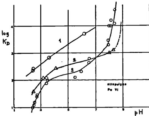
Fig. 86 : Retention of Pu (VI) by attapulgite :
