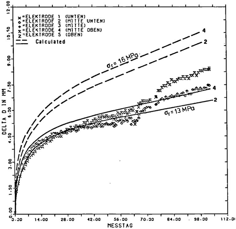
Fig. 59 : Effect of different boundary conditions on borehole closure (experiment II)
