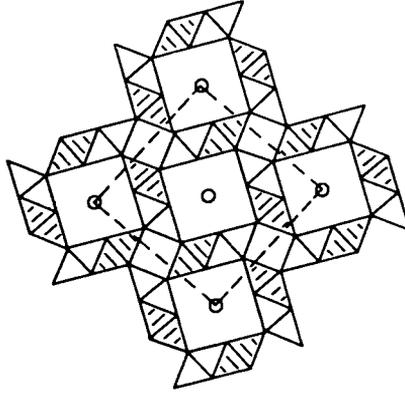
Fig. 31 : Hollandite structure. Double chains of edge-sharing octahedra share corners to produce square tunnels occupied by large A ions. The body centered unit cell is outlined.
