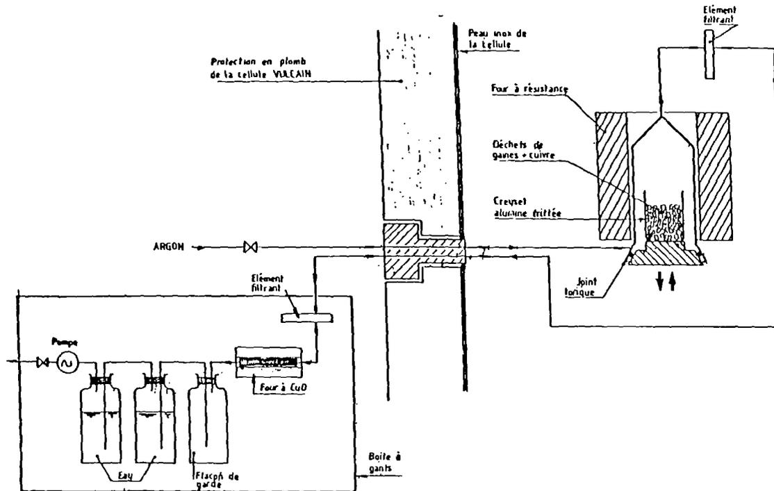
Figure 15 : Principe of the melting and off gas treatment devices
