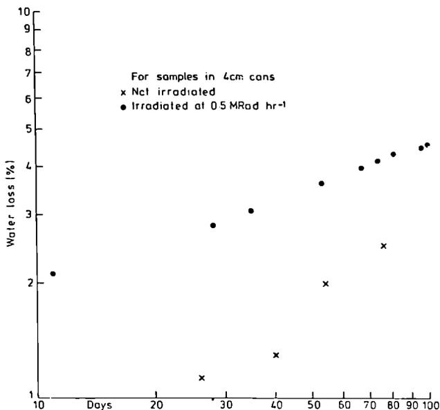
Fig. 5 : Water loss from samples of water extendable polyester resin "A" containing emulsified water droplets.
