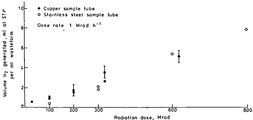
Fig. 3 : Radiolytic hydrogen evolution from magnesium hydroxide/carbonate sludge in OPC - RWF6.
