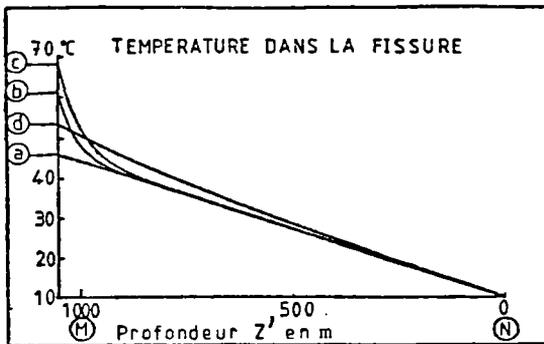
Fig. 81 : Temperature in the fracture between the waste (M) and the surface (N). a,b,c,d : for  $t = 0, 50, 100$  and  $1000$  years.
