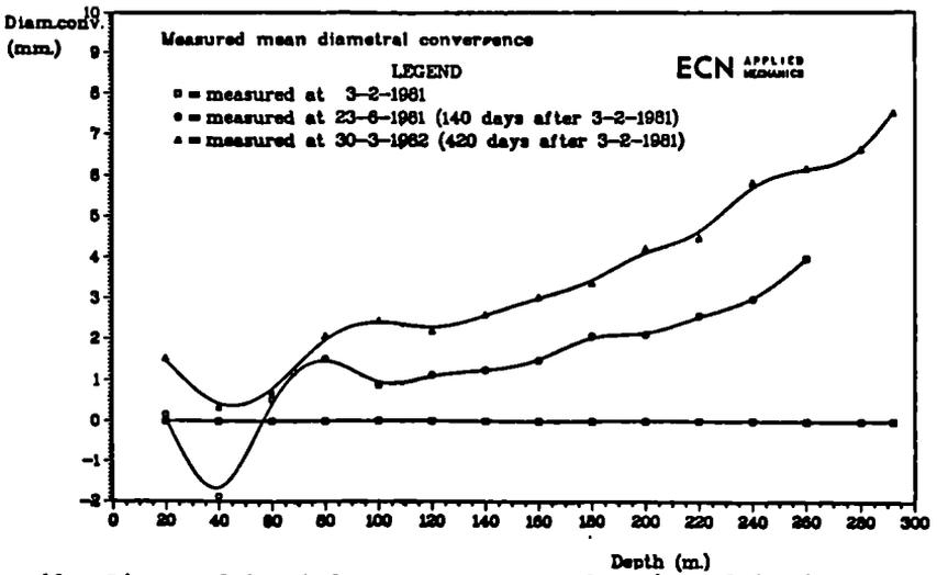
Fig. 62 : Diametral borehole convergence as function of depth
