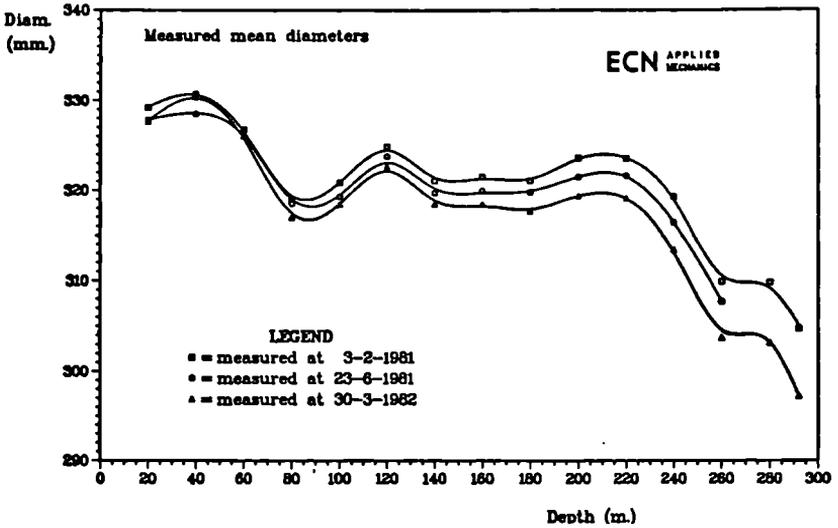
Fig. 61 : Borehole diameter as function of depth
