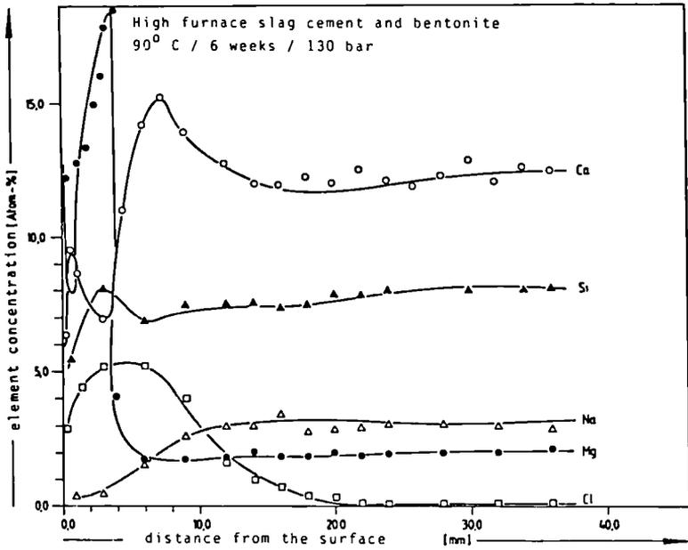
Fig. 6 : Depth-Concentration profiles of selected elements in cement samples from one dimensional corrosion experiments in quinary brine at 90° C and 130 bars after 6 weeks duration (high furnace slag cement, w/c-ratio = 0.4, 10 weight %  $\text{NaNO}_3$ , 5 weight % bentonite).
