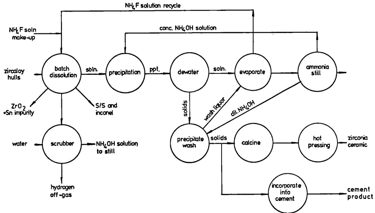
Figure 16 : Zircaloy conversion process flow diagram
