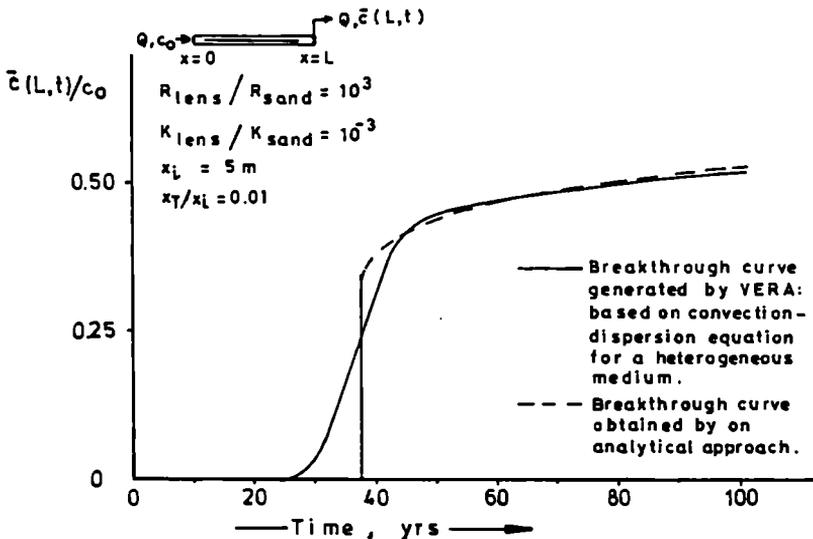
Fig. 47 : Breakthrough curve of one-lens-system
