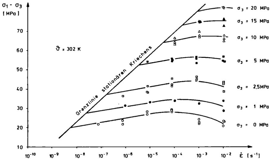
Fig. 56 : Maximum differential stress at failure as a function of axial strain rate, younger halite Na3 $\beta$ , Asse salt mine
