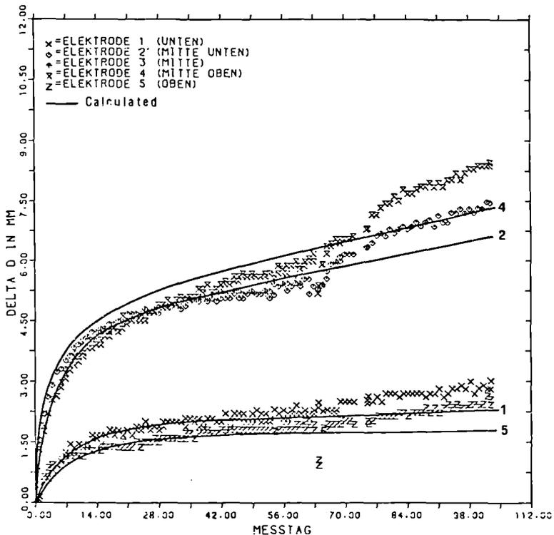
Fig. 58 : Comparison of measured and computed borehole closure for experiment II
