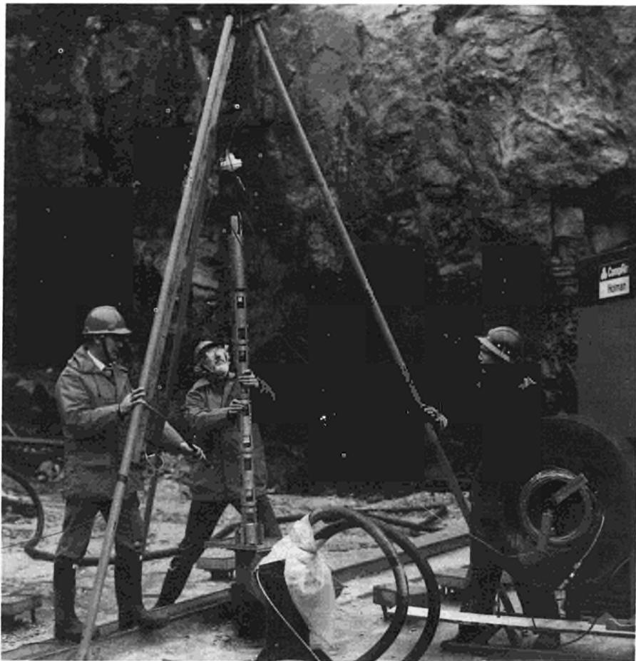
Fig. 36: Field experiment assembly lowered into the borehole at the UKAEA test site at Troon, Cornwall.
