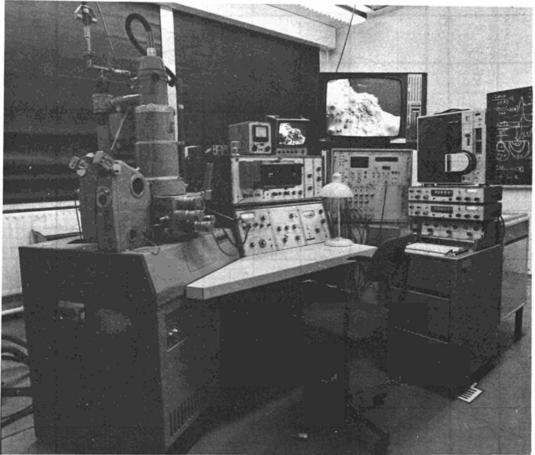
Fig. 5.2.5 Scanning electron microscope JSM U3
