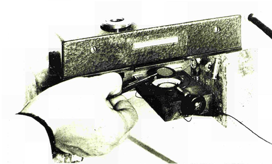
Fig. 2: Overall view of a high-temperature TSEE Counter used at Oak Ridge National Laboratory (ORNL) (24).
