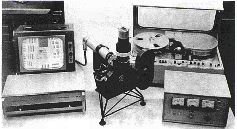
Figure 7: Cine-camera with automatic exposure control. A TV camera is mounted at 90° to the camera in place of the eyepiece. The TV screen shows the image from the transparency placed on top of the camera lens.
