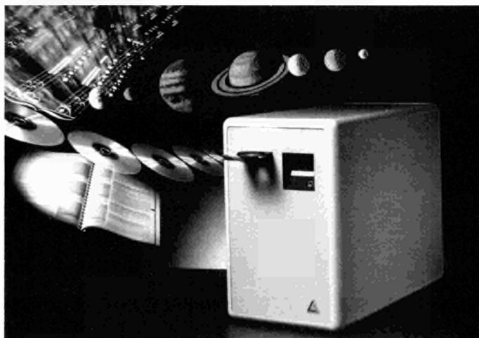
How do you store 250 times 600 megabytes of information in 150 Gigabytes? The answer is a carousel or jukebox slotting in 240 CD-ROMs. Developed by Next Technology Inc of Cambridge with partial funding of the European Commission, the new mass storage system will allow future expansion and increased efficiency for the Adonis project. The contents of some 220 biomedical journals published from 1987 to 1988 already
