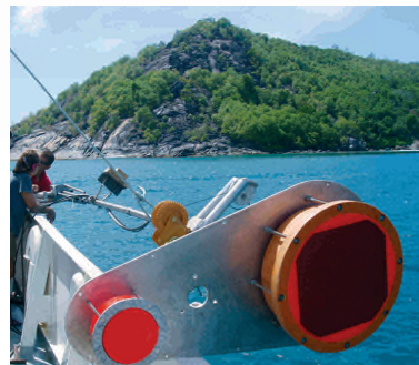
The first mission by the Fadio project to the Seychelles – fitting an echo sounder to the exterior of the vessel.
