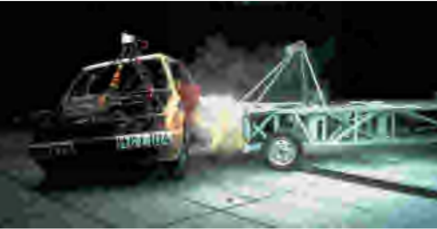
Simulation of a side impact by the INRETS.
