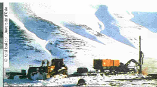
Permafrost drilling at Janssonhaugen (Svalbard – Norway) in May 1998. The borehole is now equipped with thermistors placed at intervals to a depth of 100 metres.
