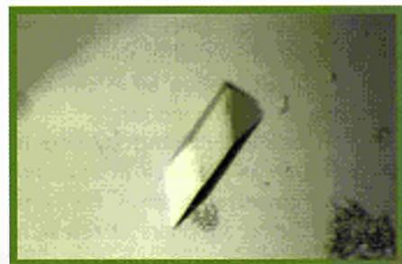
*Crystal of alpha-amylase used for x-ray diffraction to determine 3-D structure.*
