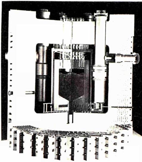
*Model of prototype 300 MWe high-temperature pebble-bed reactor proposed by Brown Boveri/Krupp Reaktorbau GmbH.*
