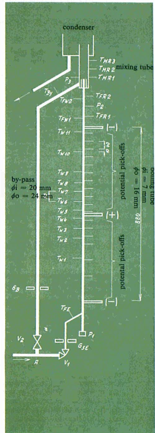
Fig. 3: Experimental loop for boiling tests with liquid metals installed at Ispra. At the various points shown, measurements are made bearing on velocity ( $v_1, v_2$ ), mass flow ( $G_{SE}, G_B$  etc.), pressure ( $P_1, P_2$  etc.) and temperature ( $T_{W1}, T_{FR}$ , etc.).
