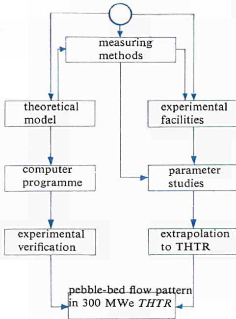
Figure 2: Block diagram of the different stages into which was divided the investigation of the pebble bed flow pattern in the core of the 300 MWe THTR prototype.
