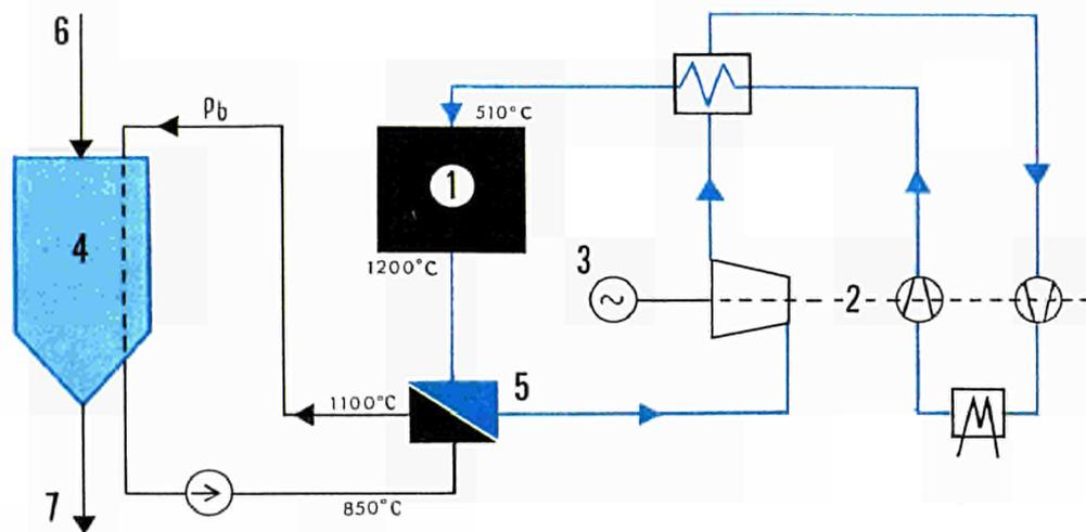
Figure 1: Direct reduction of iron ore with solid reducing agents.
