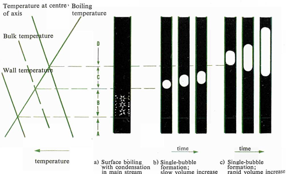
Fig. 2: Liquid metal boiling during forced convection with superheat.
