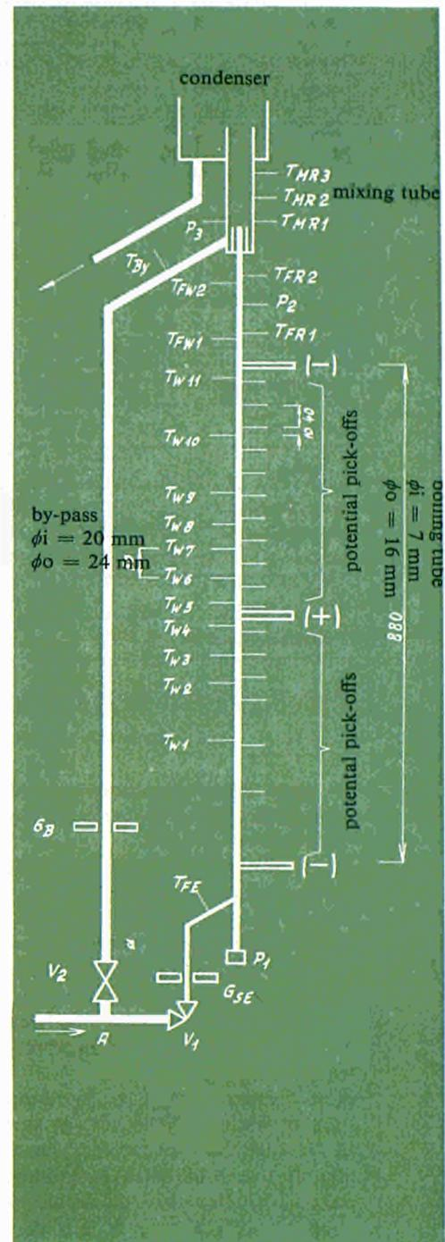
Fig. 3: Experimental loop for boiling tests with liquid metals installed at Ispra. At the various points shown, measurements are made bearing on velocity ( $v_1, v_2$ ), mass flow ( $G_{SE}, G_B$  etc.), pressure ( $P_1, P_2$  etc.) and temperature ( $T_{w1}, T_{FR}$ , etc.).
