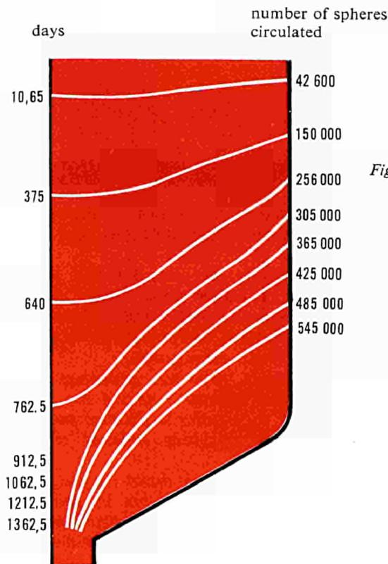
Figure 10: Flow profiles in the THTR core.
