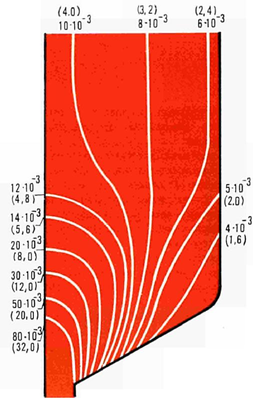
applications of the parametric studies was that the flow pattern in the THTR prototype core could be established by means of the computer programme. Another was that information was obtained with regard to the influence of the core geometry on the flow pattern, particularly with respect to higher power units.
