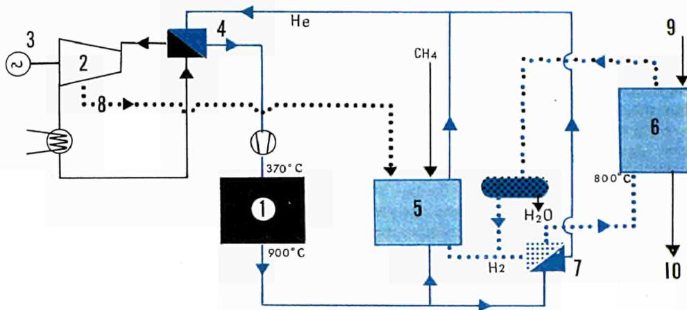
Figure 2: Direct reduction of iron ore with gaseous reducing agents.
