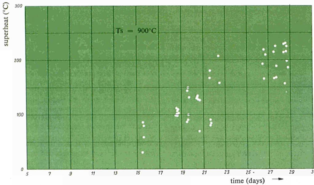
Fig. 7: Rise of superheat measured in sodium with time.
