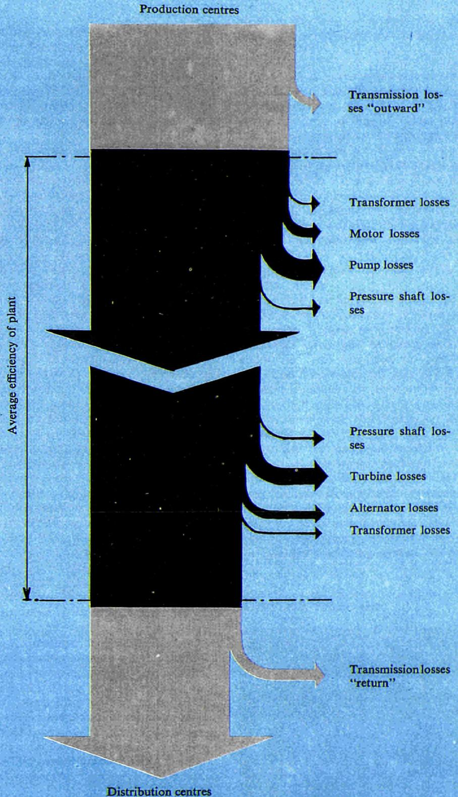
Figure 5: Breakdown of the losses for the Coö pumped storage scheme (according to the Syndicat d'étude de centrales de pompage en Belgique, July 1964).
