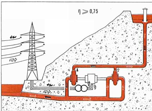
Figure 1: Principle of operation of a pumped storage scheme. Cheap energy available at certain hours is used to pump water into the upper reservoir (white arrows). At peak hours the energy is restored by the turbines (black arrows).
