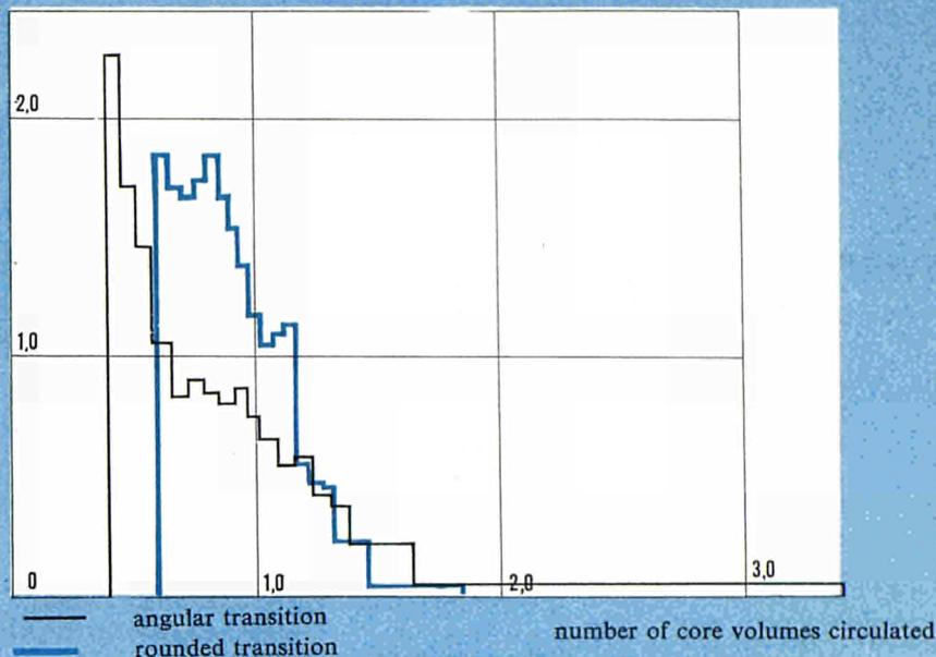
Figure 6: Residence spectra, measured on a 1 : 15 model of the THTR core; the effect of the transition between the cylindrical wall and the conical base is shown. The frequency distribution in accordance with which test balls initially on the top surface leave the core is plotted.
