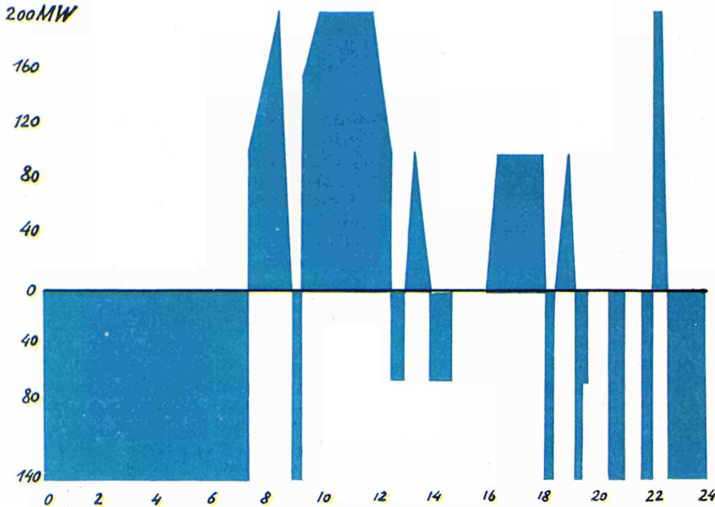
Figure 3: Typical daily load diagram of the Vianden pumped storage station after the commissioning of the first two groups.
