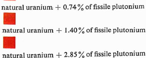
*Enrichment distribution in the rods of three types of fuel element used in the plutonium recycling experiments at Garigliano nuclear power plant.*
