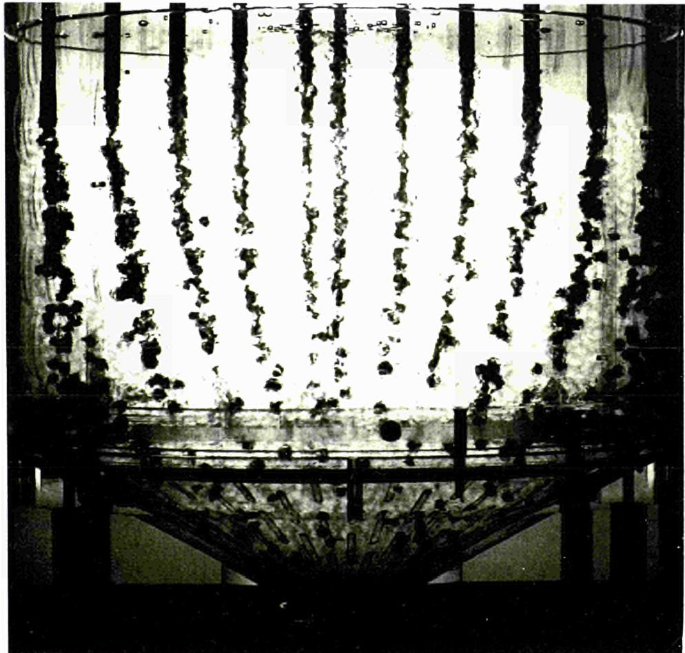
*Figure 5: Sphere paths as photographed in a glass sphere model.*
