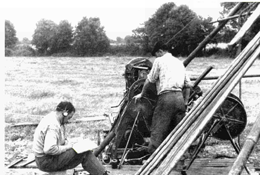
Radio-core-sampling by means of a Geiger-Müller counter (CEA, France)
