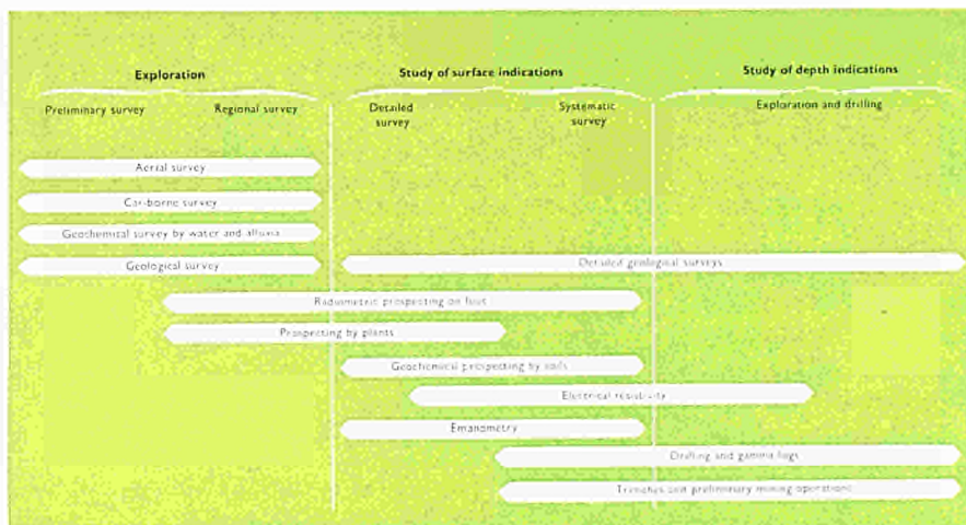
Fig. 5: The methods employed in the various stages of prospecting for uranium
