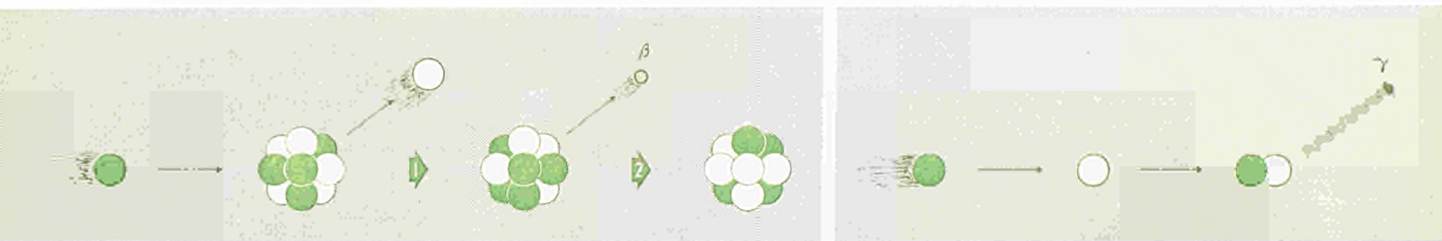
Figure 6: Interaction of a slow neutron with the nucleus of an element. Two examples are given of the interaction of a slow neutron with a nucleus. In both cases the neutron is absorbed. Left: A neutron interacts with a (stable) nitrogen-14 nucleus, which releases a proton to give a (radioactive) carbon-14 nucleus. The carbon-14 nucleus emits a \beta -particle and disintegrates into a stable nitrogen-14 nucleus. Right: A neutron interacts with a proton (hydrogen nucleus) to give a deuteron. \gamma -radiation is released.
