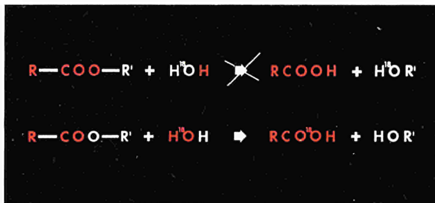
Figure 2. Determination of the hydrolysis mechanism of esters. Thanks to the use of water marked with oxygen-18 ( H^{18}OH ) we can determine that the hydrolysis reaction follows the second pattern.
