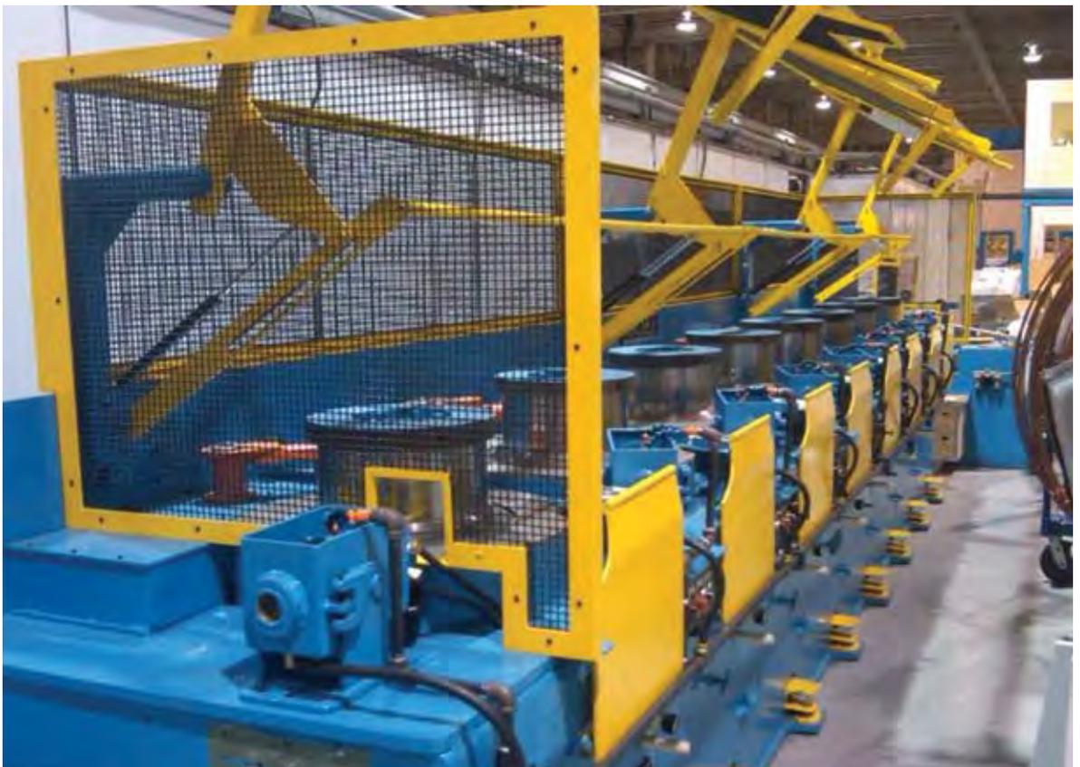
Fig. 7: Manufacturing facility for Nb<sub>3</sub>Sn strand drawing (courtesy of OST)
