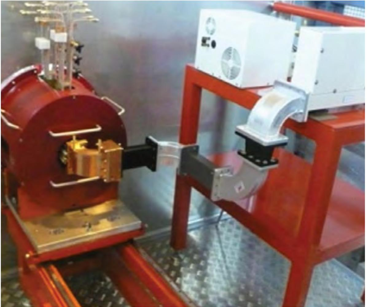
Fig. 28: Ion source and RF chain on HV platform
