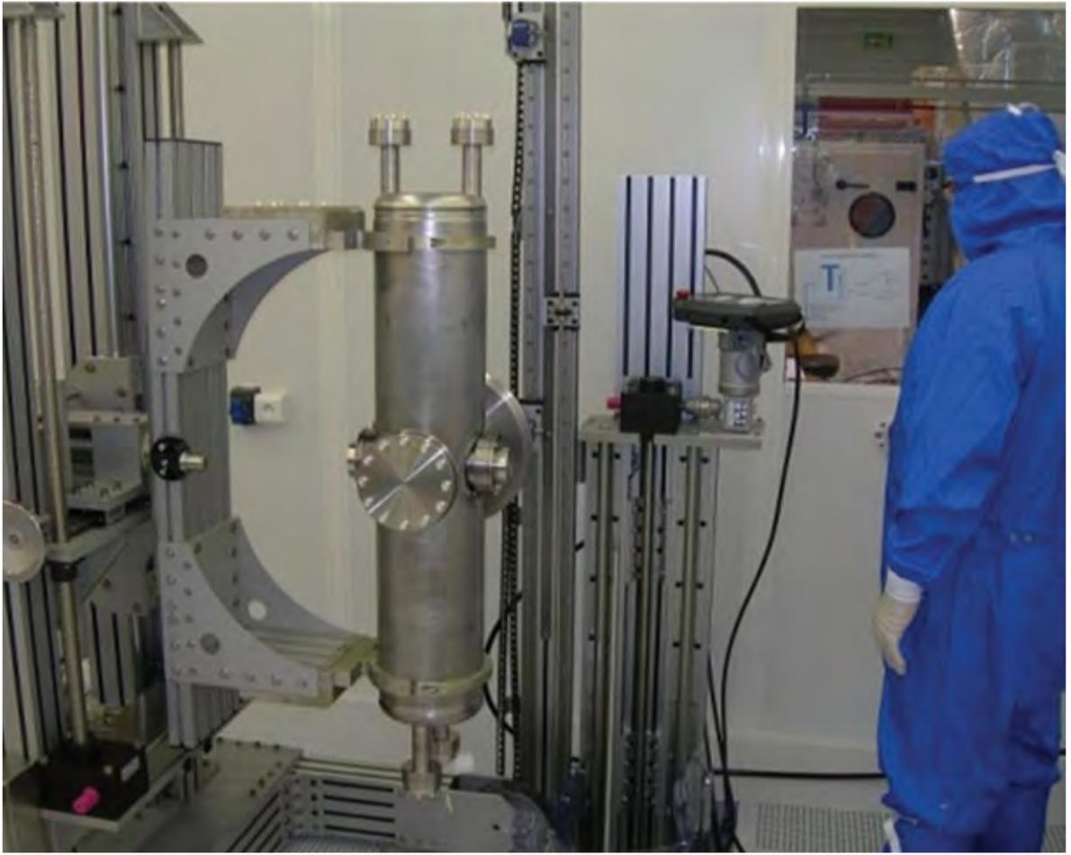
Fig. 30: High pressure rinsing of the Half-Wave Resonator prototype (P01) manufactured for the Superconducting RF Linac
