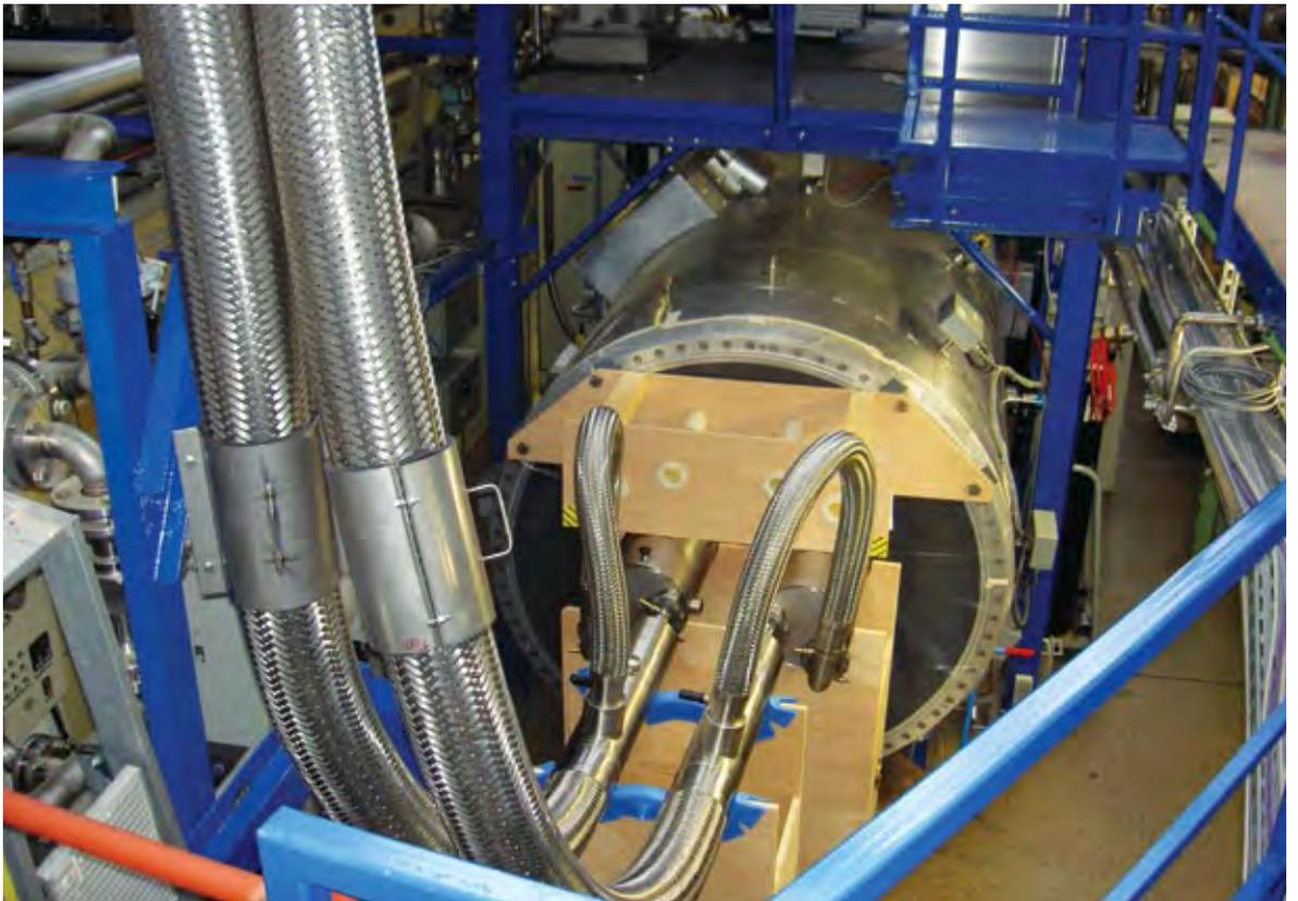
Fig. 13: View of TIMO-2 Facility at KIT being upgraded to provide 4.35 K supercritical He for testing the ITER Torus Cryopumps (courtesy of KIT)
