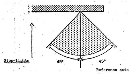
(\*) The angles shown in these diagrams are correct for devices to be mounted on the right side of the vehicle. The arrows point to the front of the vehicles.
