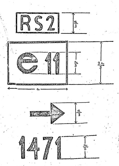
The device bearing the EEC type-approval mark shown above is a device comprising both a rear light and a stop light, with two levels of illumination, approved in the United Kingdom (e 11) under the number 1471. The arrow means that, on the side to which it points, the photometric specifications are satisfied up to an angle of 80°H.
