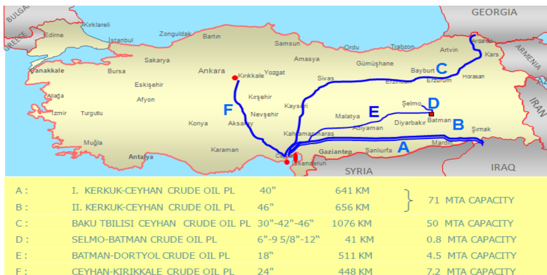
Figure 50. Turkey – Crude oil pipelines
