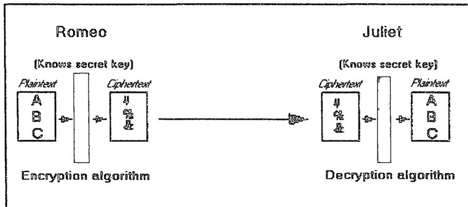
Fig. 3 Symmetric encryption
