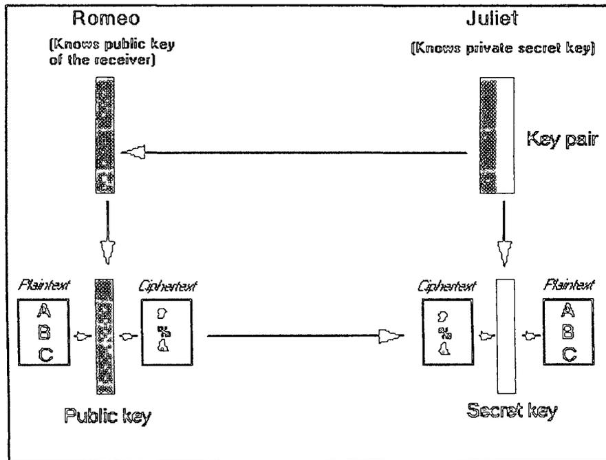
Fig. 4 Asymmetric encryption
