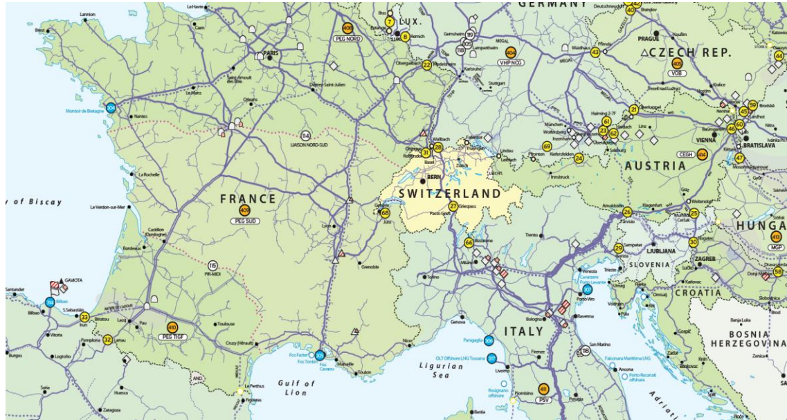
Figure 3. Natural gas pipelines and entry/exit points in continental Europe (detail)
