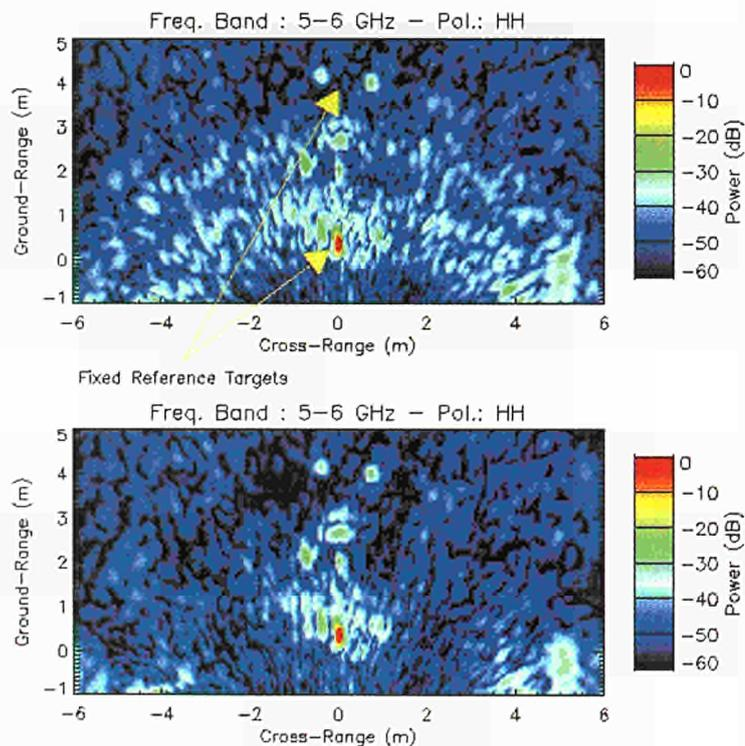
Figure 6.4: Diagram illustrating how the coherent signal averaging technique removes artifacts due to unfocused images of moving parts in vegetation cover. SAR image of a group of trees including ‘wind’ effect (above). The same image where the artifacts have been removed by temporal coherent averaging (below)
