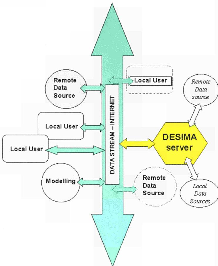
Figure 5.4: DESIMA distributed client/server architecture
