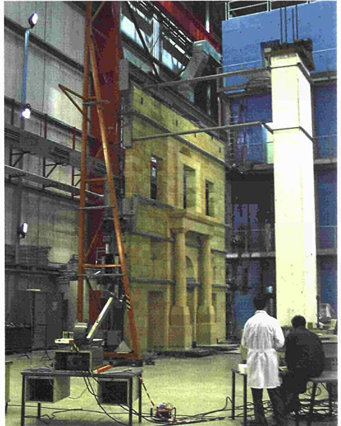
*Figure 12.1: The facade of Palazzo Geraci undergoing deformation tests at ELSA while the LISA SAR system acquires radar data to assess the deformation behaviour by means of 3-D SAR Interferometry*
