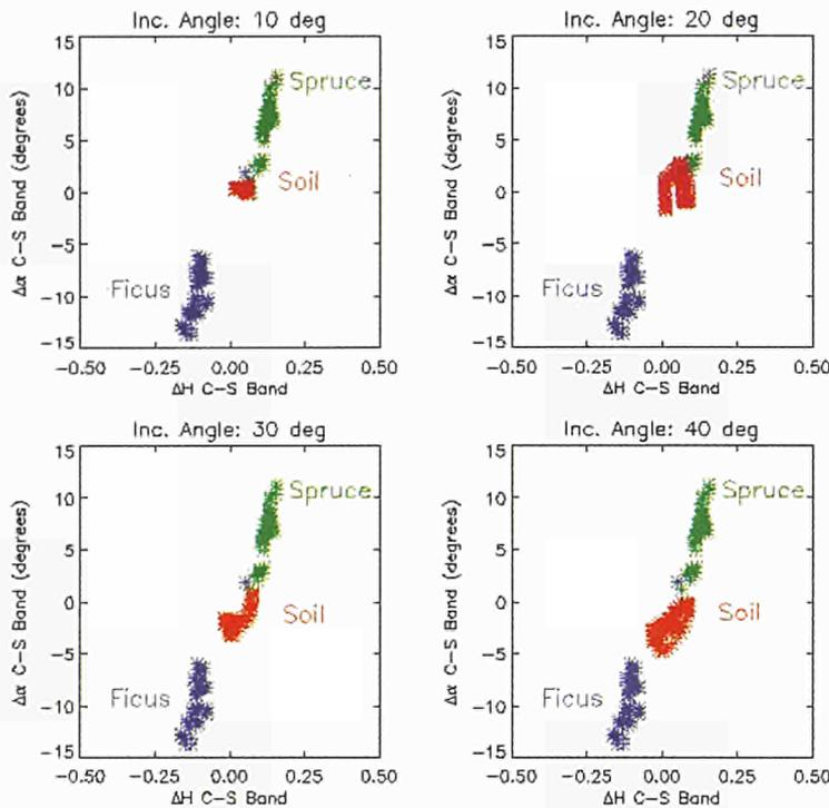
Figure 6.3: Scatterplot showing the separability of two tree species and a smooth soil surface by means of their polarimetric radar signatures
