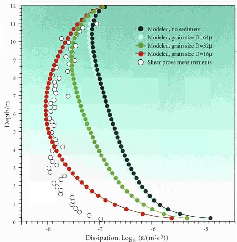
Figure 5.2: Comparison of measured and modelled (using the K-e model) dissipation rates for the Oosterschelde experiment
