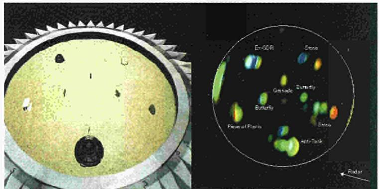
Figure 7.1: Anti-personnel mines identification using high resolution polarimetric microwave imaging. The colour-coded image (right) shows the dominant scattering mechanism for each target in the test scenario (left) which includes different types of mines and non-dangerous objects
