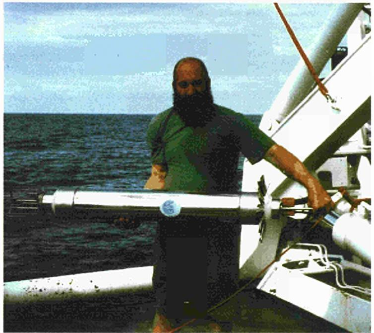
Figure 5.1: Micro-structure profiler prepared for measurements in the falling mode of operation
