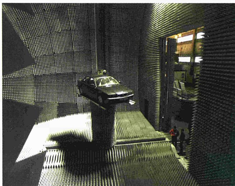
Figure 12.2: A BMW car is transported inside the measurement chamber. The radiation patterns of different types of telecommunication antennas located inside the car are measured by performing a full rotation of the target positioner about the vertical axis
