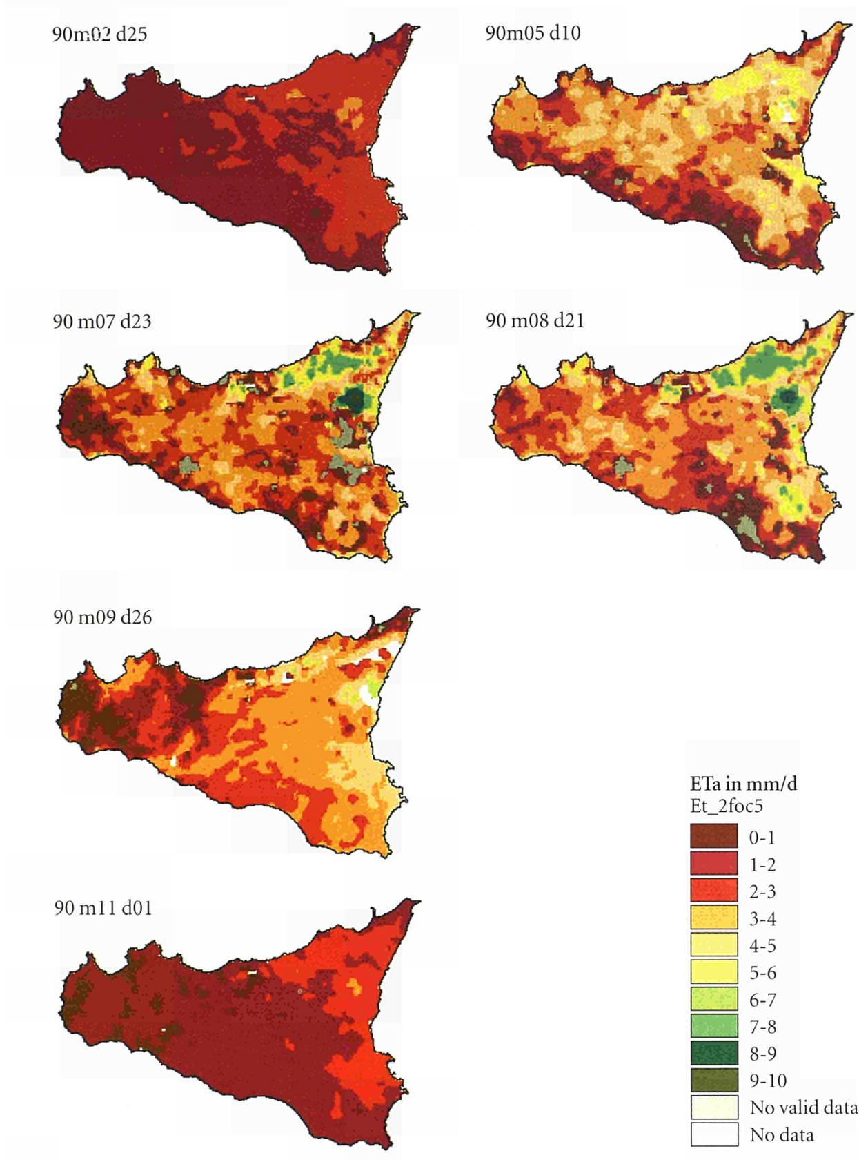
Fig. 4.2: Estimated actual evapotranspiration for selected days in 1990 for Sicily. Model outputs are based on meteorological data, land cover data, digital elevation data, and remote sensing data (surface temperature, surface albedo, vegetation index). The model resolution is 1x1 km. The presented data have been smoothed by a 5x5 pixel moving window filter.
