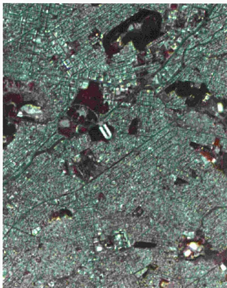
Figure 3.2: Fusion of multi-spectral and panchromatic IRS-1C imagery for the city of Athens, Greece. Spatial resolution is 5 m. (Based on IRS-1C data, copyright by ‘ANTRIX SIE’, Euromap Neustrelitz)
