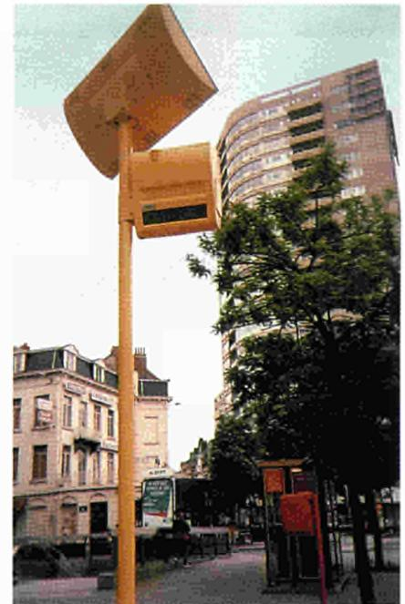
**User information post on trial in Brussels. Installed as part of the PHOEBUS project, the display gives waiting passengers travel information such as the number and destination of the next bus as well as the likely waiting time.**
