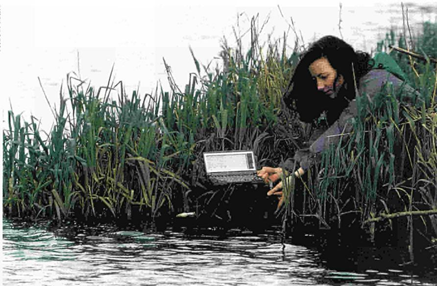
**A water analysis system based on a disposable sensor incorporating sensing and calibration electronics has been developed in B-ASICS (project 6240). The system can rapidly measure concentrations of heavy metals in a few drops of water, enabling real-time on-site pollution monitoring.**
