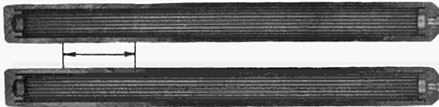
Fig. 4: W-26 Re/Li heat pipe (116 mm long) after 10,000 hours of horizontal operation at 1600°C, average heating rate 120 w/cm 2 . The flash indicates the heating zone. Vertical cut, Li removed.
