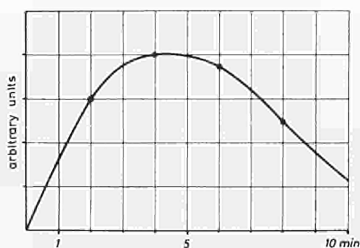
Fig. 3: Typical build up of the dynamic polarization with time. Ordinate arbitrary units.
