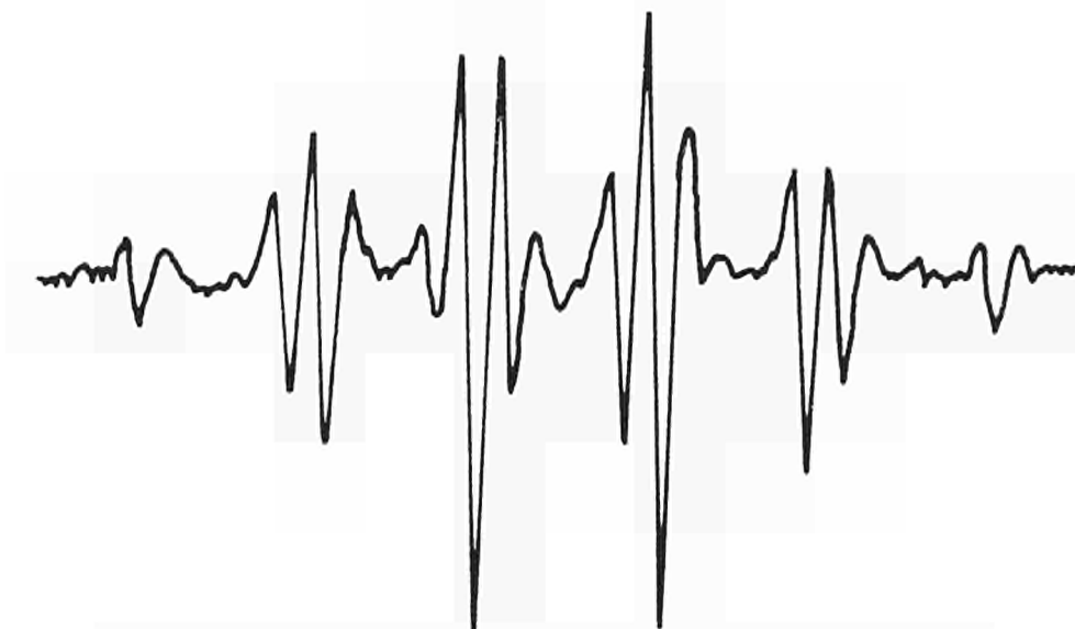
Fig. 1: An experimental E.S.R. spectrum of Ethyl Radical (second derivative).
