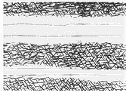
Fig. 2: Longitudinal section of unidirectionally Ni-Ni 3 Ta eutectic exhibiting fine precipitates in the matrix interlamellae space. (865 x)
