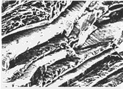
Fig. 9: Scanning electron microscope picture of the rupture zone Ta specimen with the broken lamellae of intermetallic Ni_3Ta . (450 x)
