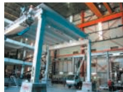
Precast Industrial Building model tested at the ELSA Laboratory in the framework of the competitive project PRECAST-EC8
