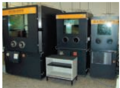
Climatic chambers used in the EID laboratory for the device certification
