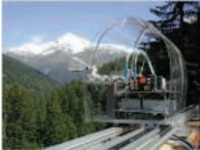
LISA (Linear Synthetic Aperture Radar) is a system developed by JRC-IPSC which is able to monitor in real time ground displacements and avalanches in high risk areas
