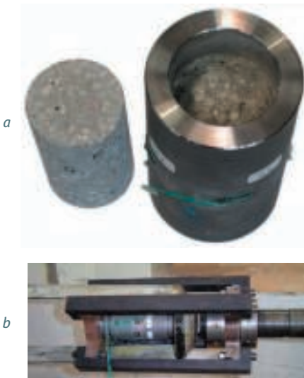
Dynamic axial compression of concrete with lateral confinement:
