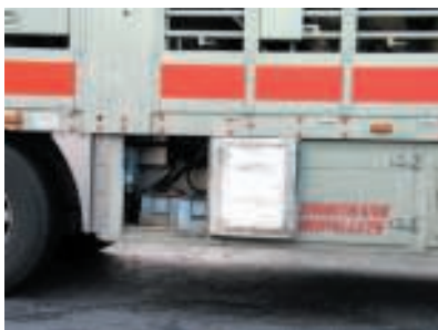
On Board Unit installed in a truck dedicated to animal transportation
