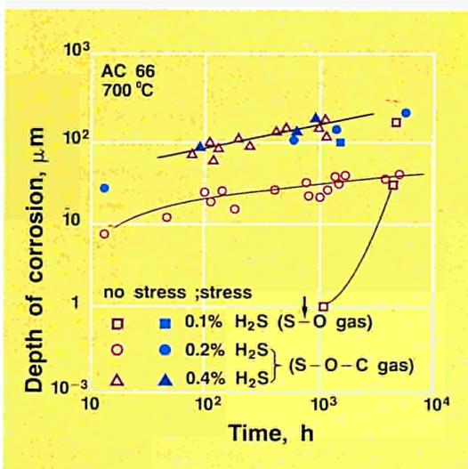
**Left:** Depth of internal corrosion versus exposure time for stress free and stressed AC 66 at 700°C in various S-O-C bearing gases
