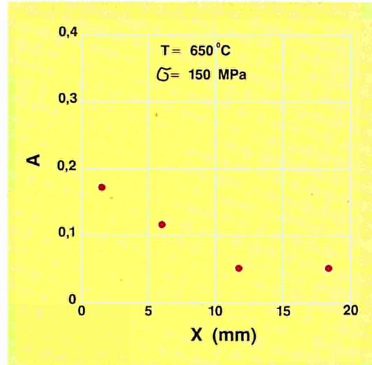
Above: A-parameter determined in the ruptured specimen  $t_r = 167$  h
