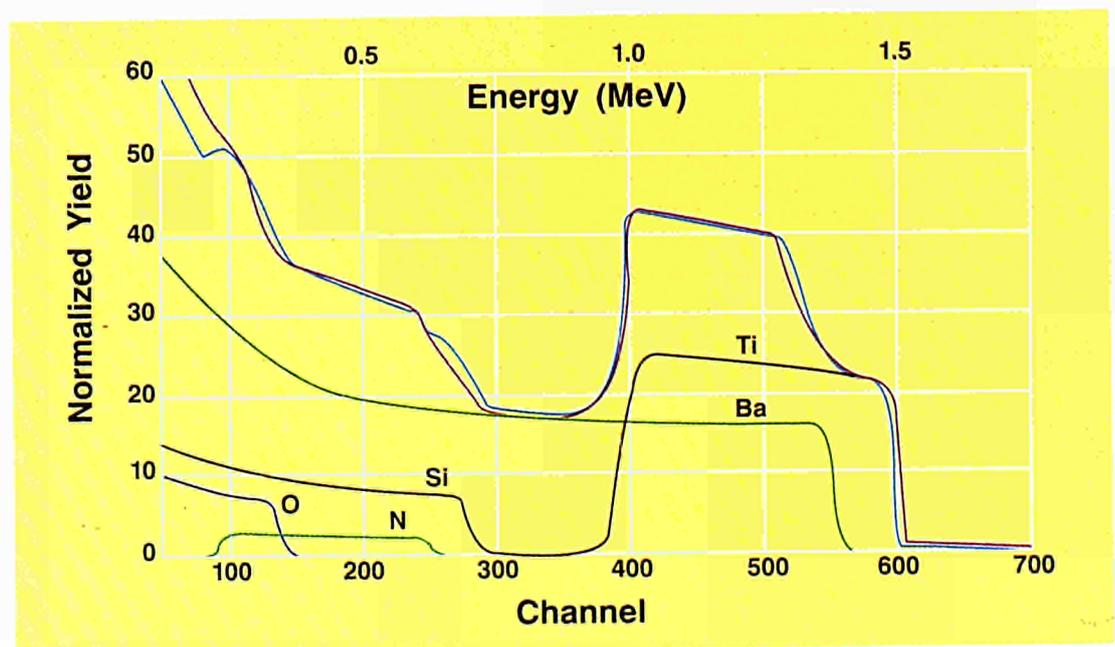
The chemical composition of the film (and substrate) has been obtained by modelling a spectrum from single element contributions.
