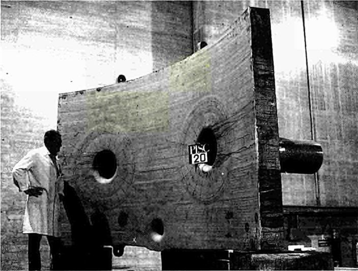
**Above:** PISC III Action 3 (NDW). Assembly with three nozzles and safe-ends of the BWR type. This assembly is also a key element for any evaluation of new inspection possibilities of old plants considered for life-extension
