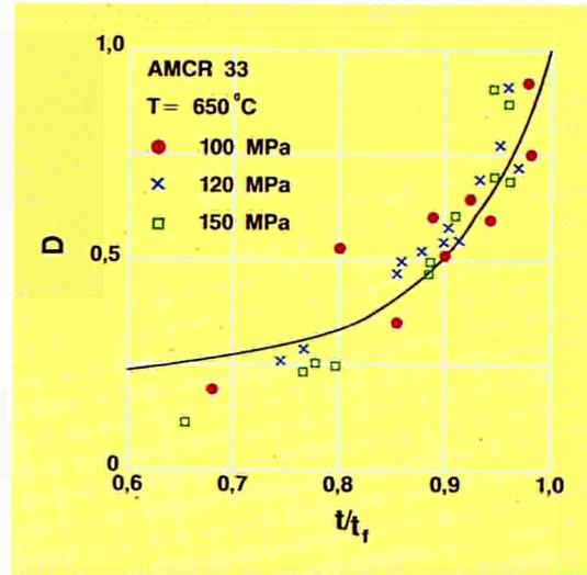
**Above:** Damage-parameter D determined from the creep curve. Dashed line calculated with the Hutchinson-Riedel model
