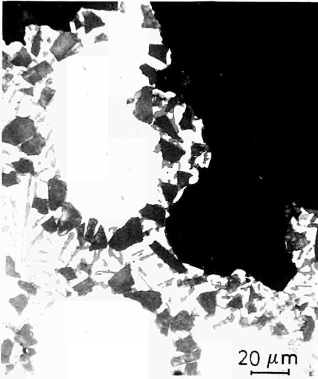
**Above:** Fracture surface profile of the A356 + 20% SiC composite (F temper) broken at room temperature ( $\epsilon = 1 \times 10^{-4} s^{-1}$ ).
