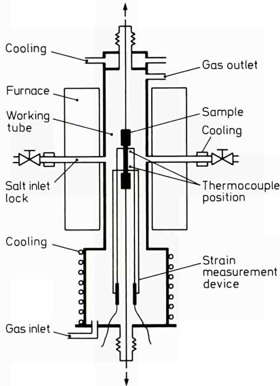
**Above:** Equipment for creep testing in controlled atmospheres with independent salt addition
