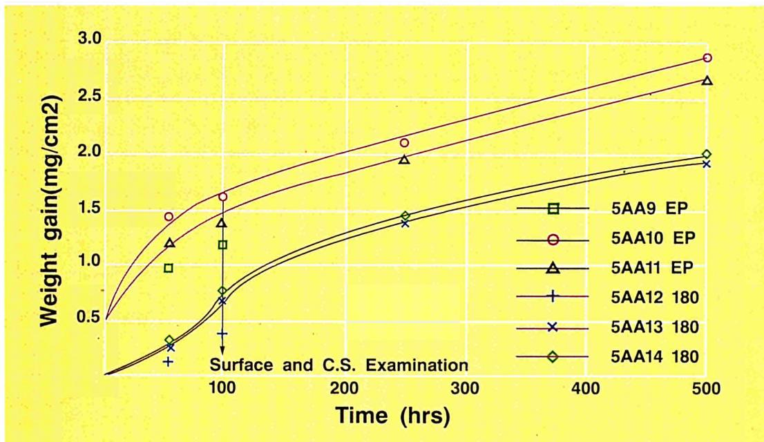
Corrosion kinetics at 600°C/0.6% $H_2S$  - M.A. 956
