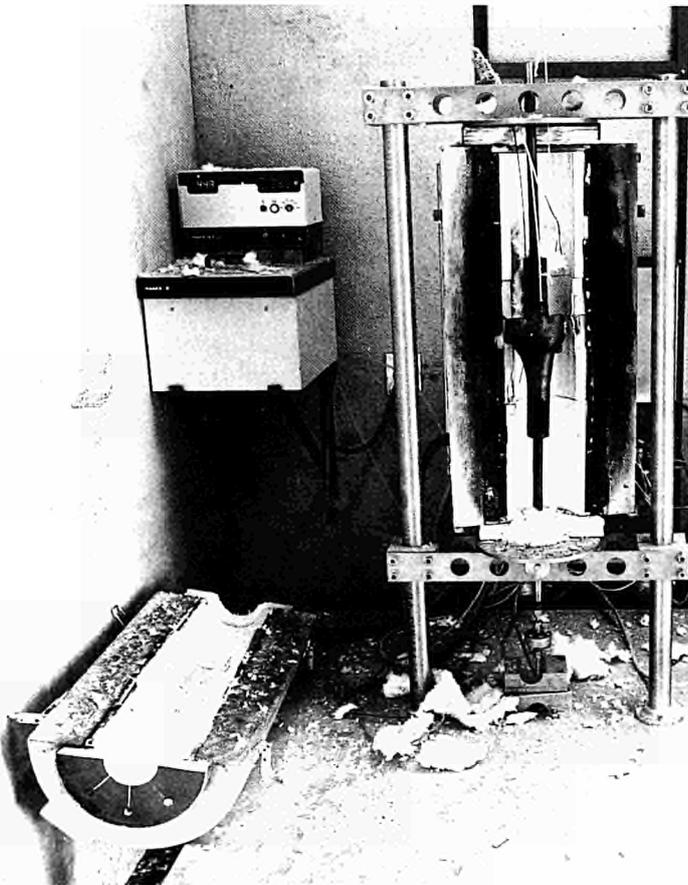
**Above:** PD instrumented longitudinal notch ( $2\frac{1}{4}$ Cr1Mo).
