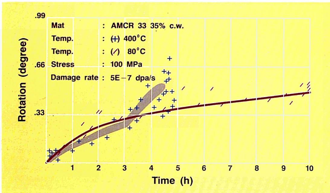
In order to give an explanation for this unexpected irradiation creep behaviour at low temperatures, two types of experiments have been performed. In a first series of tests the irradiation creep rate of a 20% cold-worked 316 L stainless steel specimens has been determined as a function of the deuteron flux for a specimen temperature of 85°C. The damage rates ranged from 2E-7 to 8E-7 dpa/s. The results are given in figure below.
