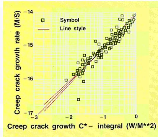
**Above:** Creep crack growth rate VS.  $C^*$ -integral, alloy 800H at 550°C
