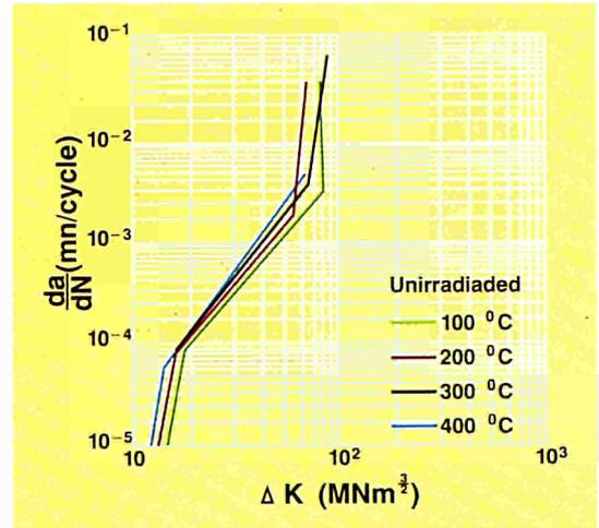
**Above:** Crack growth per cycle versus stress intensity factor for unirradiated AISI type 316 steel
