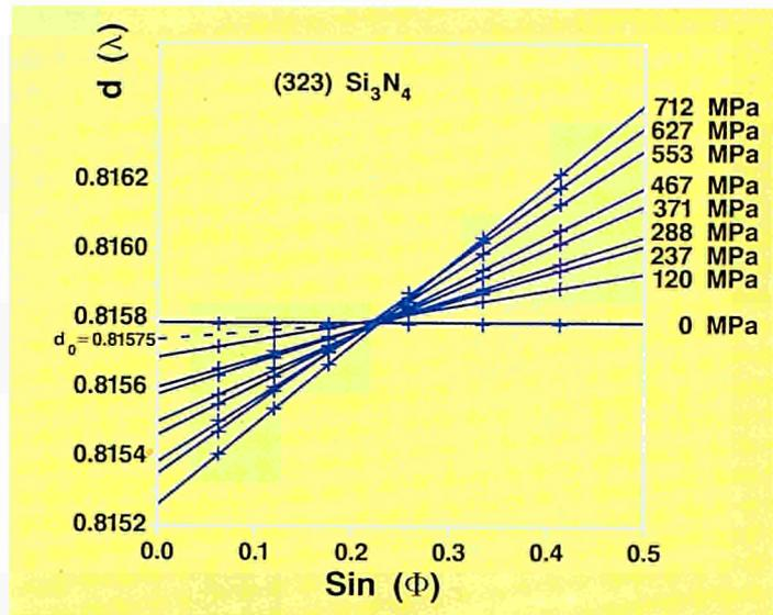
Above: Lattice Spacing vs.  $\sin^2 \phi$  as a function of applied stress
