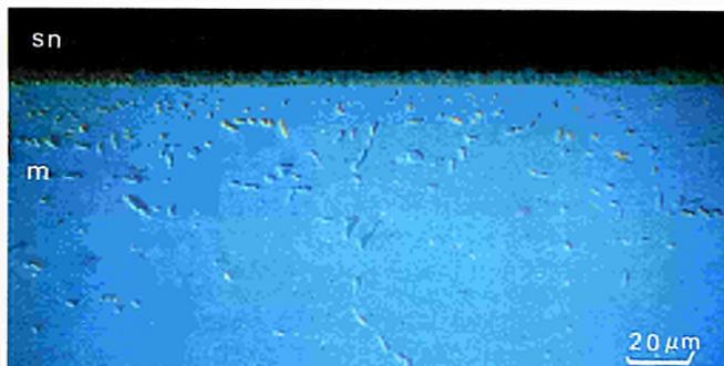
**Above:** Microstructure of a joint interface; joining conditions: 1200°C, 100 MPa, 1h, Argon (sn: silicon nitride, m: filler metal).
