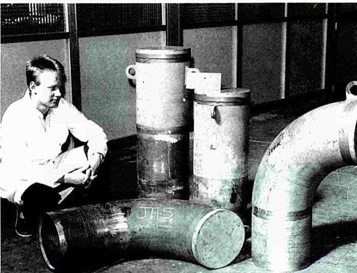
An American BWR assembly with two nozzles and safe ends and a Spanish PWR nozzle and safe end began their circulation mid 1989 (Figures above). These round robin tests are planned to continue until January 1991.
