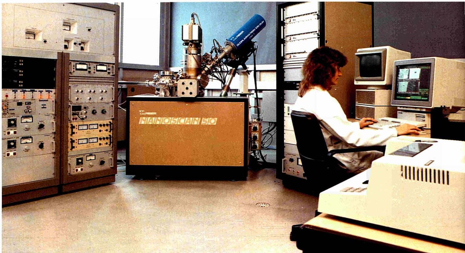
b) RIBER Scanning Auger Microscope:
