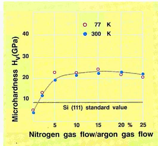
**Above:** Microhardness of TiN films, which have been sputter deposited at different gas flow ratios of nitrogen and argon, respectively
