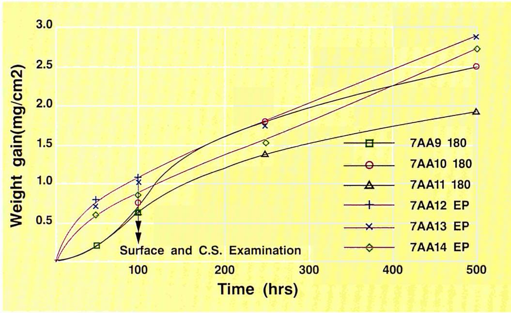
Corrosion kinetics at 600°C/0.6% $H_2S$  - FeCr alloy
