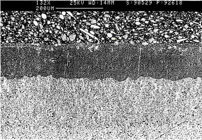
**Corrosion of Cr-Mn based Austenitic Stainless Steels by Pb-17Li**
