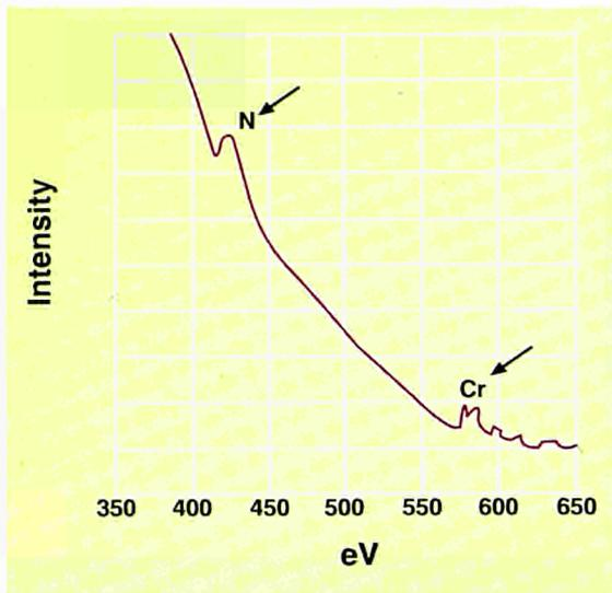
**Above:** EELS spectrum intragranular He bubbles shown in the figure on page 96 above indicating enrichment of Cr and N near their surface
