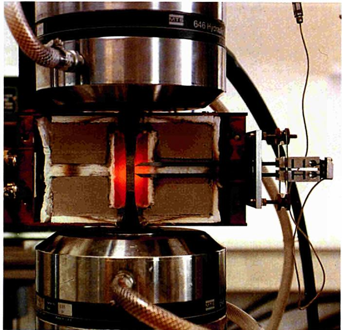
**Above:** View on half of the split furnace used in cyclic fatigue testing of ceramics
