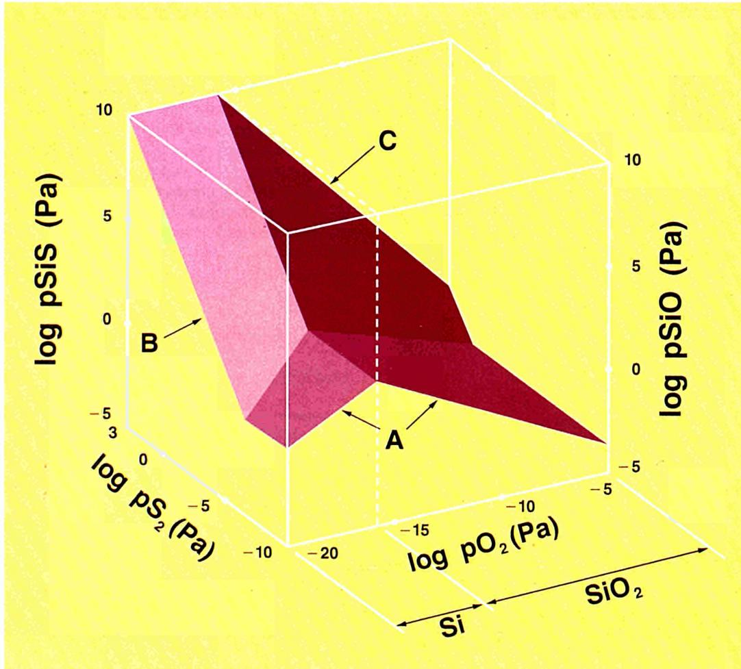
This thermodynamic model has been confirmed by the experimental data which show that the catastrophic corrosion rates observed in region B (mass losses up to  $850\mu\text{g cm}^{-2}\text{h}^{-1}$ ) may be reduced by two orders of magnitude by small additions of water vapour to the environment, thus shifting the thermodynamic activities into region C.
