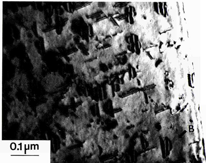
**Above:** Formation of large Frank interstitial dislocation loops due to the interaction of interstitial Cr with N together with very small He bubbles (B) in AMCR 0033 steel implanted with 1000 atppm at 773 K.
