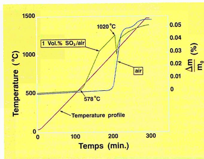
Above: Thermogravimetric comparison of the behaviour of a HPSN(Y) ceramic in air and 1 vol% SO<sub>2</sub>-air
