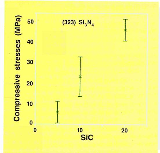
The determination of interphase stresses in ceramic composites in contrast show significant differences of residual stress values. For a silicon nitride-silicon carbide (whisker) composite, stresses generated by thermal expansion mismatch are compressive in the matrix and tensile in the whiskers. Variation of matrix stress with whisker content shows a significant increase (figure right).
