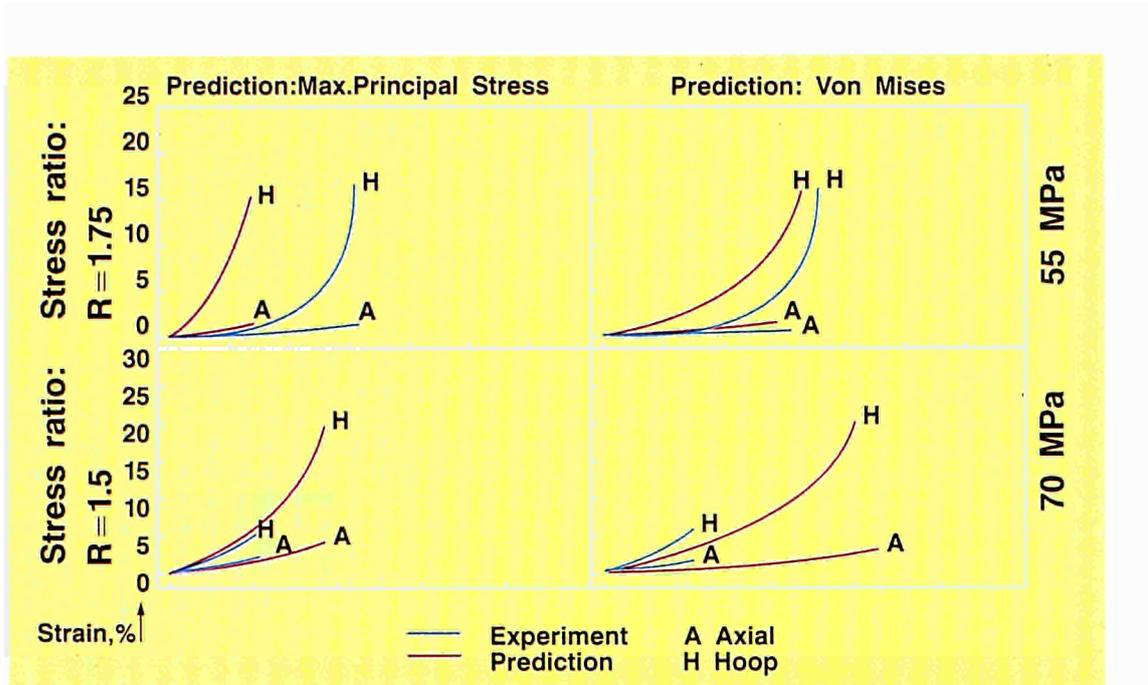
The stress rupture behaviour under multiaxial stresses better reflects the predictive ability of the model.
