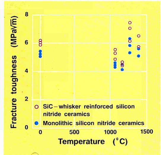
Above: Variation of fracture toughness with temperature
