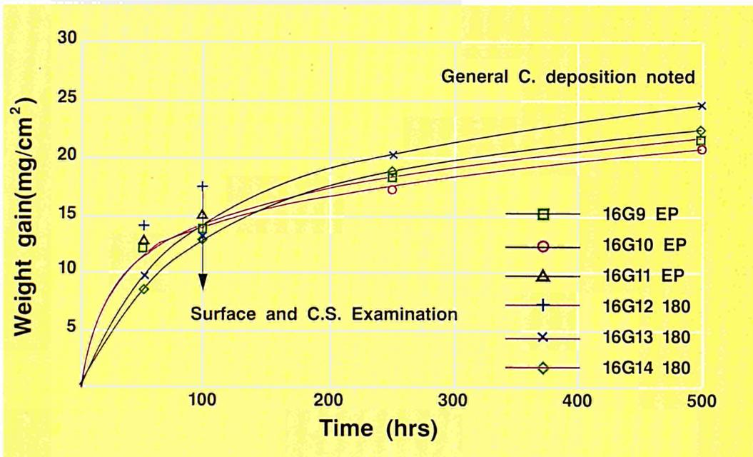
Corrosion kinetics at 600°C/0.6% $H_2S$  - Alloy 800H
