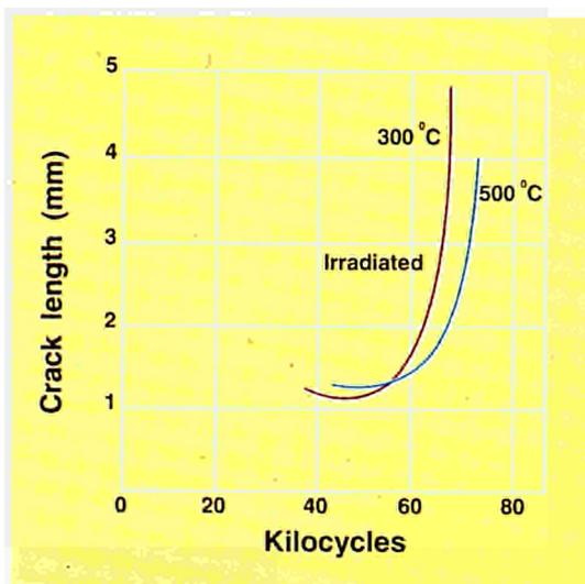
**Above:** Fatigue life under irradiation at 300°C and 500°C
