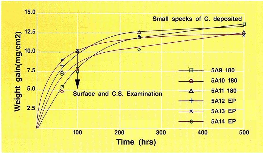
Corrosion kinetics at 600°C/0.6% $H_2S$  - A.I.S.I. 310
