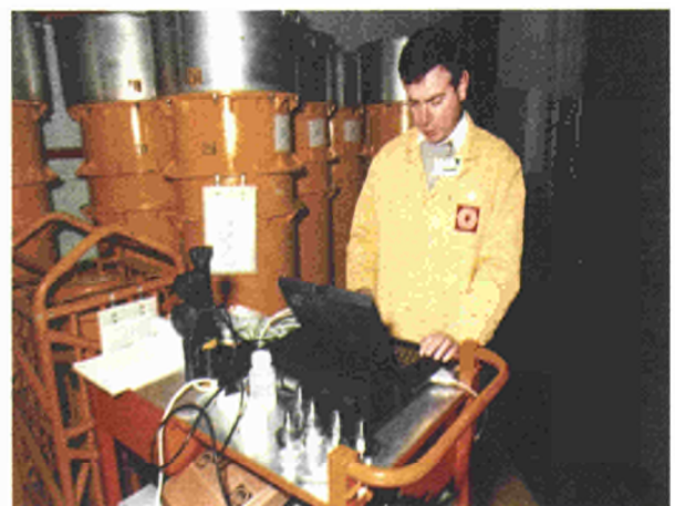
Fig. 3.9 Preparation of a transport test with on FS-47 casks from COGEMA facility in Cadarache (F)
