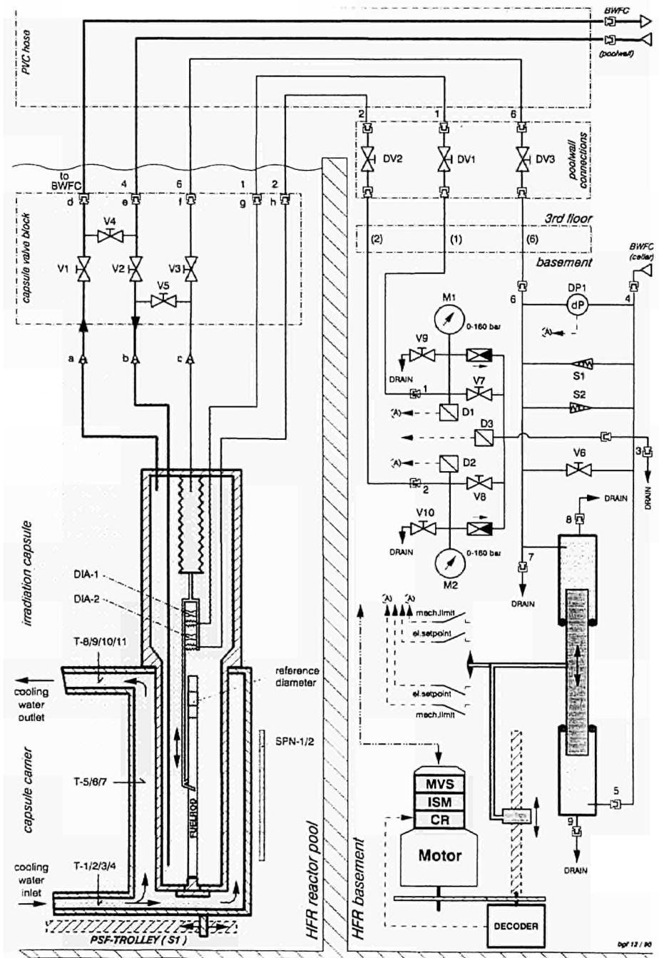
irradiation device was performed and yielded feasibility for application of both coolant media, light water and heavy water. The irradiation device is reloadable and provides intermediate inspection capabilities of the irradiated samples. During this period an additional study was performed and confirmed for the light water system feasibility of accommodation of two independent loop systems in a TRIO-type irradiation rig.
