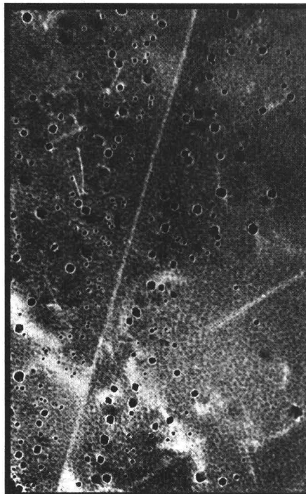
Petten Basic research on materials. Transmission electron micrographs of vanadium, neutron irradiated at 600°C to a dose of about 3 \times 10^{21} n/cm 2 (energy of neutrons over 0.1 MeV). On the left, high purity vanadium; on the right, high purity vanadium pre-injected with 10 atomic parts per million of helium (50,000 x)
