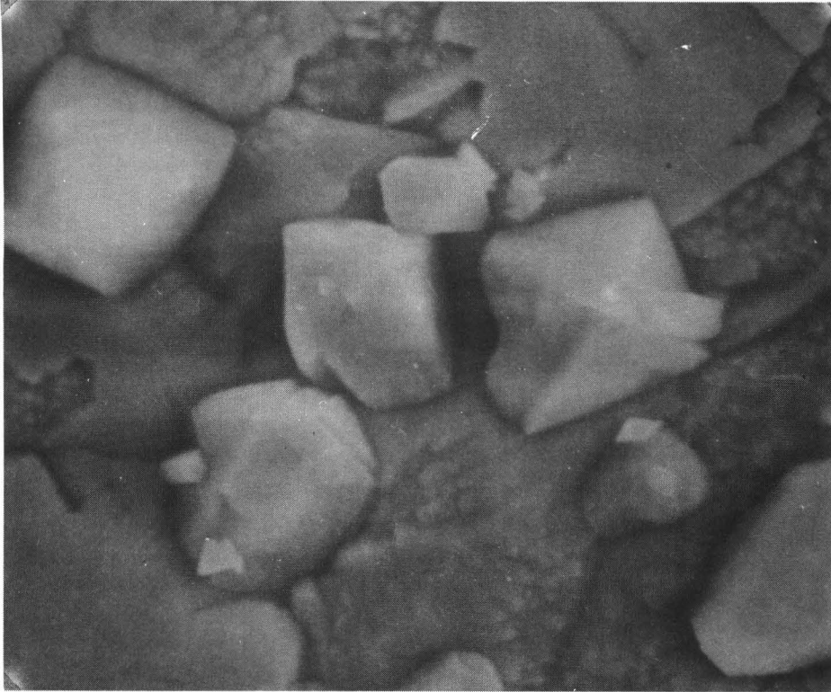
Ispra Basic research on materials. Scanning electron micrograph of Ni-foil containing octahedral-shaped precipitates of NiO.
