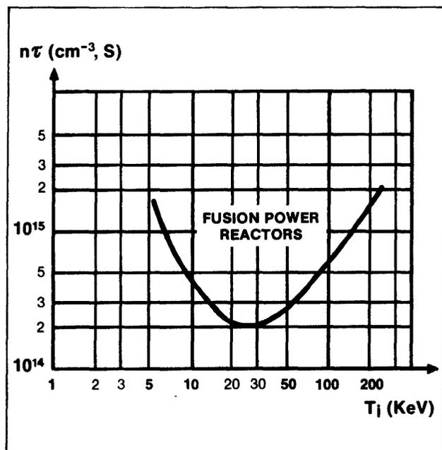
Fig. 2. Ignition curve for the D-T reaction
