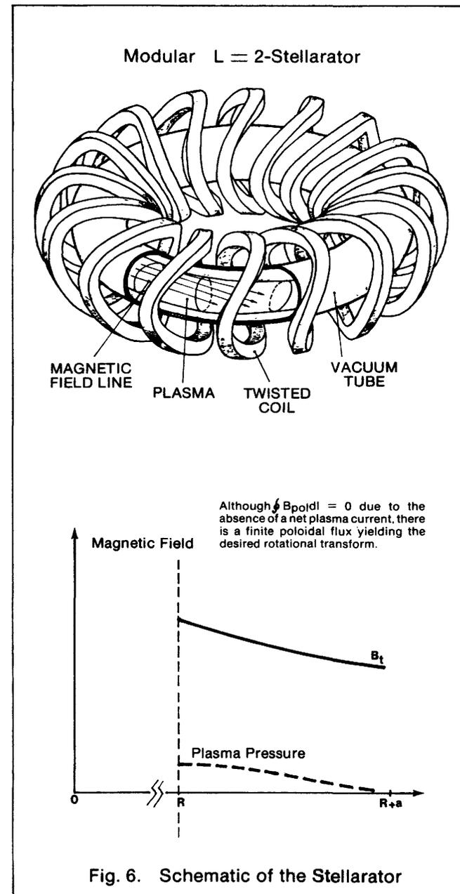
Fig. 6. Schematic of the Stellarator
