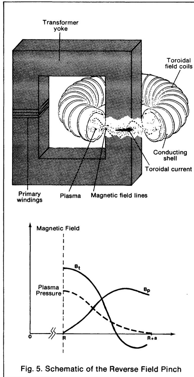
Fig. 5. Schematic of the Reverse Field Pinch
