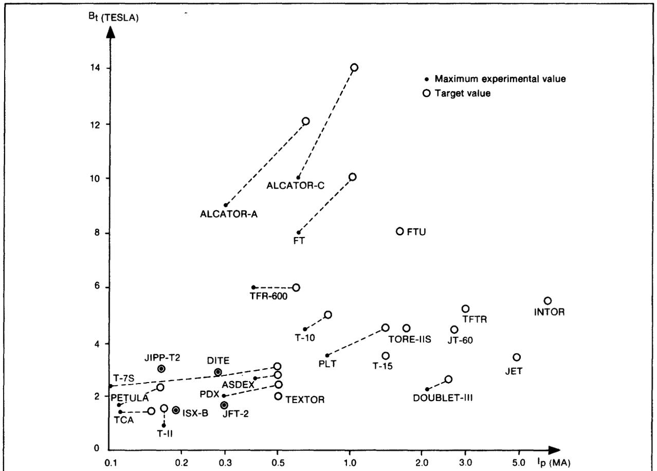
Fig. 10. Planned Performance of Tokamaks compared with actual performances. (Toroidal magnetic field  $B_t$  and plasma current  $I_p$ )
