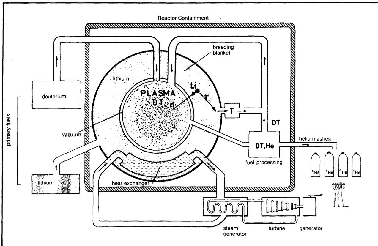
Fig. 1. Principle of a Fusion Reactor
