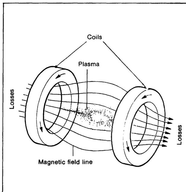
Fig. 3. Schematic of the magnetic mirror
