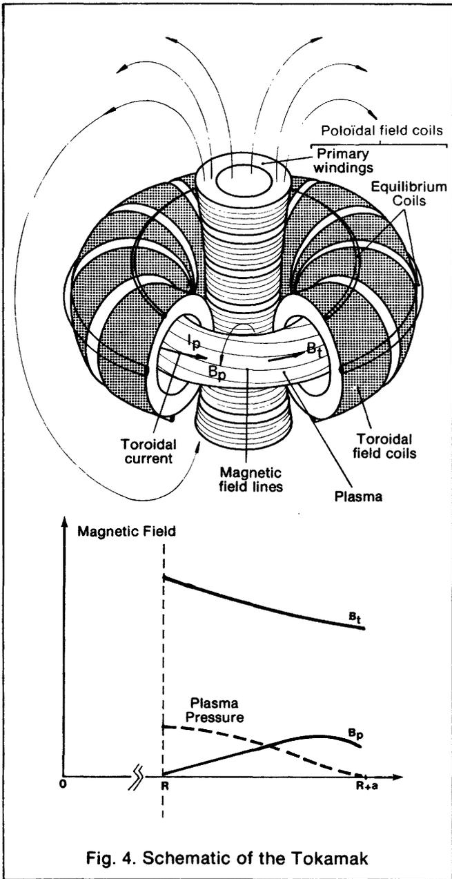
Fig. 4. Schematic of the Tokamak
