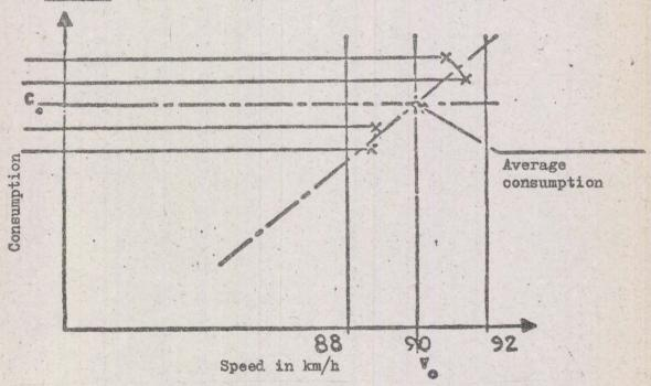
The four crosses correspond to the calculated values for each test run. Co is the value calculated for the consumption, at the reference speed. Vo over the test distance.
