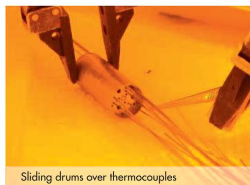
Sliding drums over thermocouples
