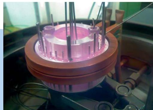
Brazing test in an induction furnace
