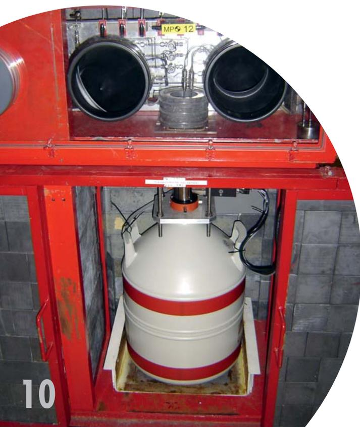
Figure 9 - Gamma spectrometer in HFR
