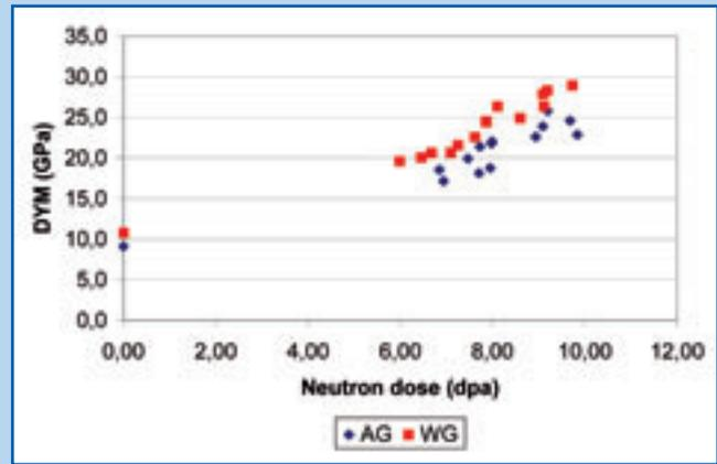
Figure 37 - The Dynamic Young's Modulus (DYM) of a typical isomoulded graphite, before and after irradiation to 9 dpa\_g at 750°C. (It is assumed that the specific heat of graphite is not changed during irradiation)
