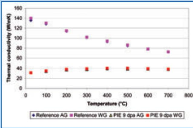
Figure 36 - The coefficient of thermal conductivity as a function of temperature of a typical extruded graphite, before and after irradiation to 9 dpa\_g at 750°C. (It is assumed the specific heat of graphite is not changed during irradiation)
