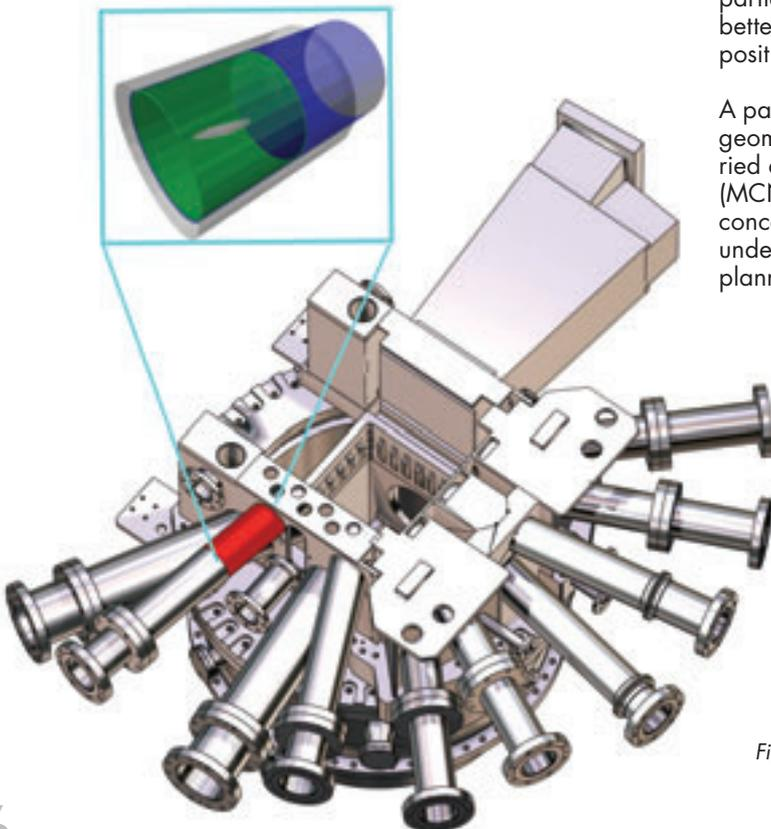
Figure 21 - Position of positron generator at HFR-HB9
