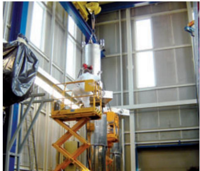
Figure 4 - Loading of a cask for shipment to the US
