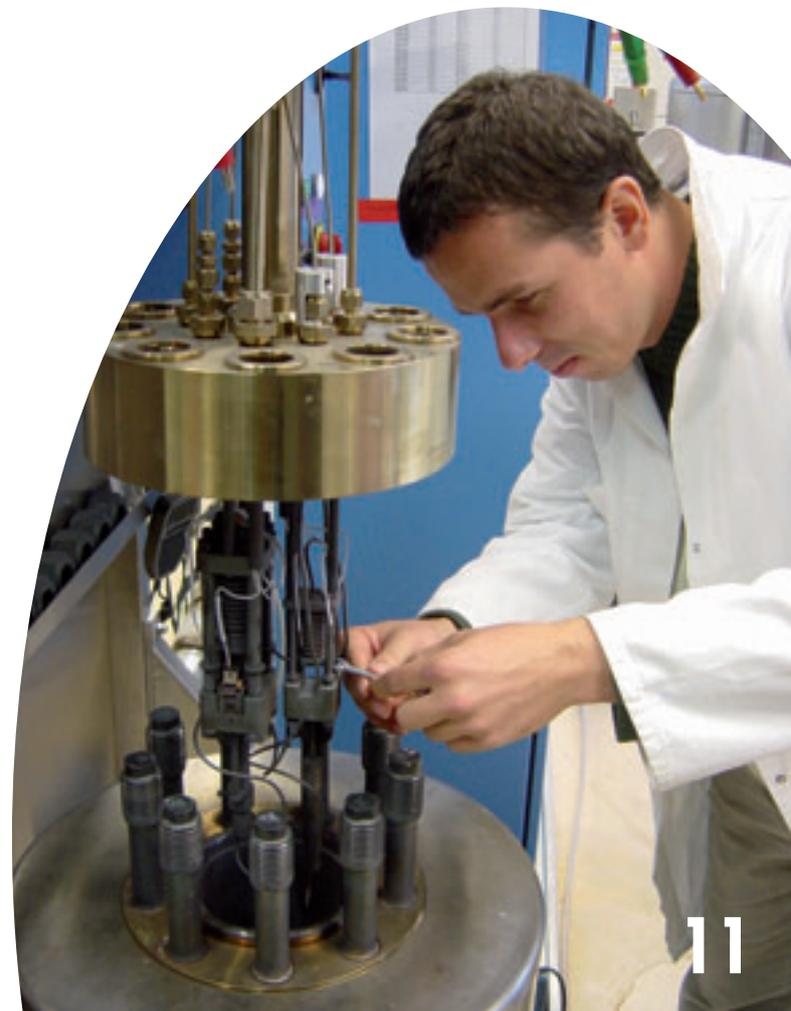
Figure 11 - Autoclave for Stress Corrosion Cracking (SCC)
