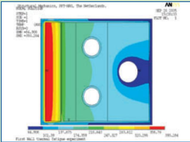
Figure 41 - Temperature analysis for PWM in-pile test
