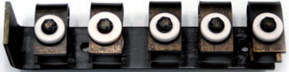
Figure 8 - Typical U-band samples for Stress Corrosion Cracking (SCC)
