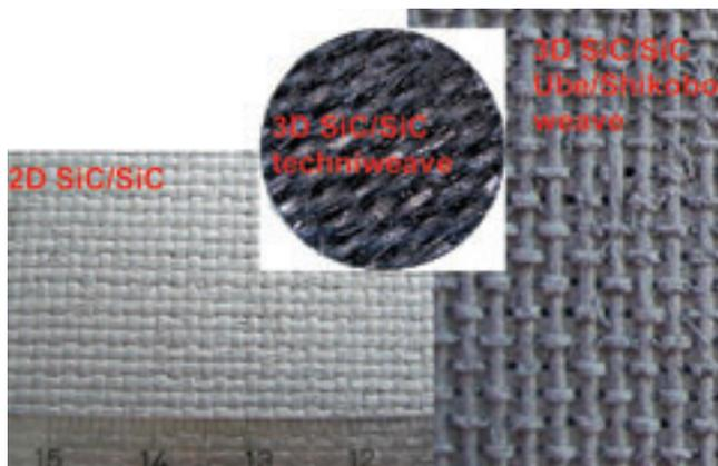
Figure 47 - Pictures of 2D and 3D SiCSiC composite produced by European industry
