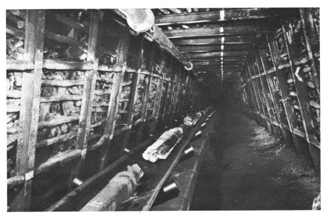
Fig. III-7: Belt conveyor for carrying material in a supply gate
