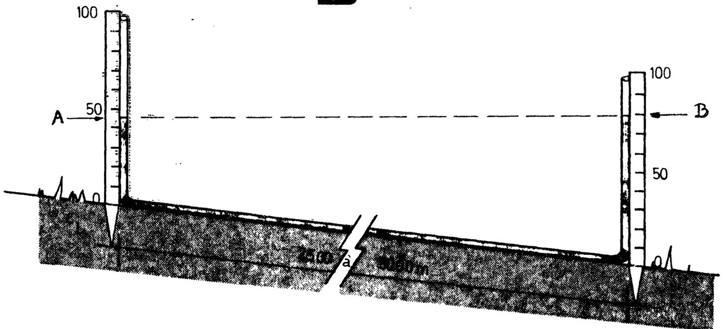
Considering the limited length of the tube, it is recommended to repeat the exercise several times at different sites along a 1 km stretch of the watercourse and to average the obtained measurements.
