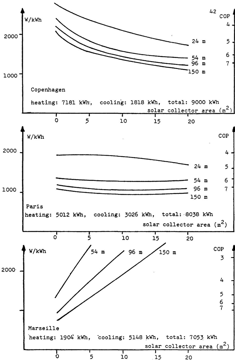
Fig. 13 Energy consumption and COP of the heat pump for the three destinations.
