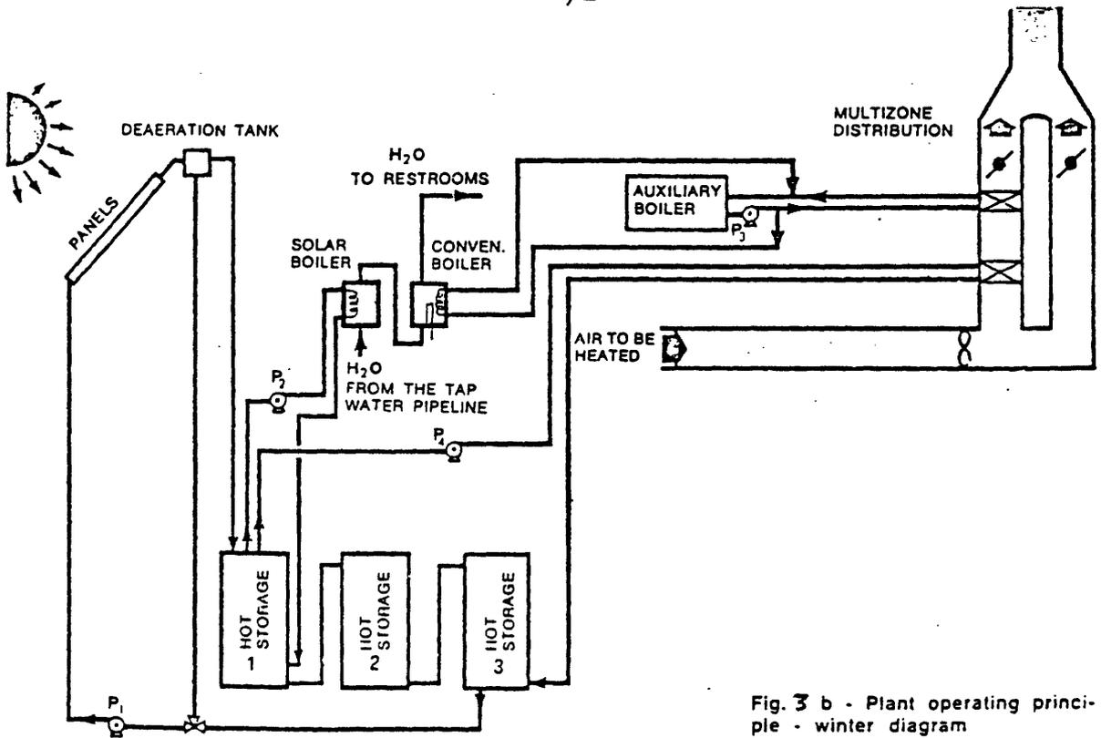
Fig. 3 b - Plant operating principle - winter diagram
