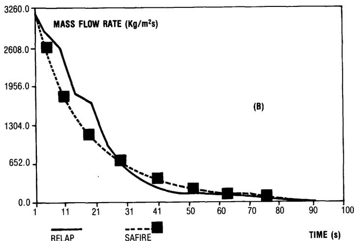
Fig. 13 - Comparison between SAFIRE and RELAP5 concerning the water blowdown test "3"
