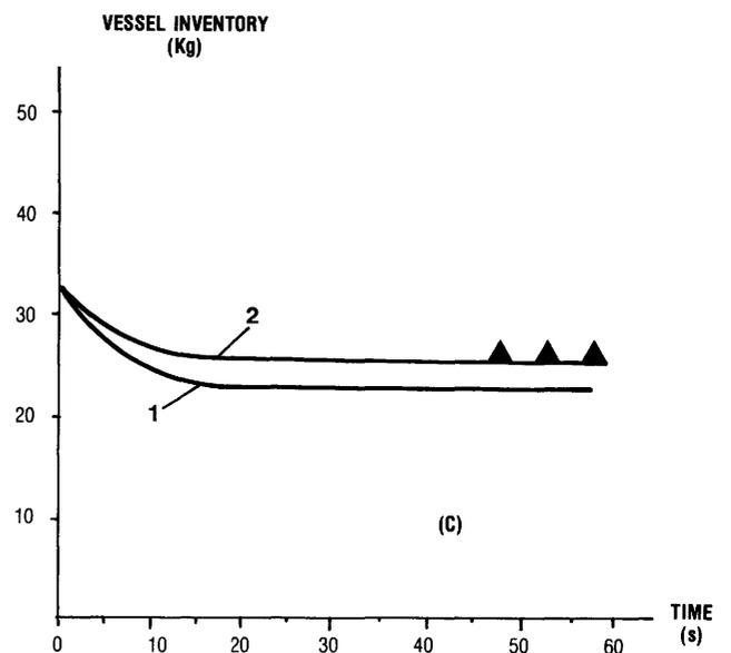
Fig. 10 - Comparison between SAFIRE calculations and measured data concerning the water blowdown test "1" performed with the MPMC-TF
