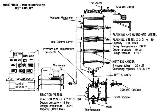
Fig. 6 - Multiphase - Multicomponent Test Facility
