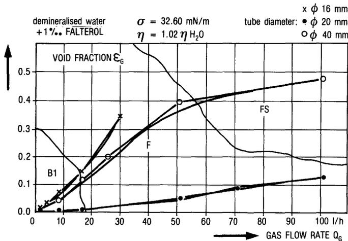
Fig. 3 - Void Fraction Versus Gas Flow Rate
