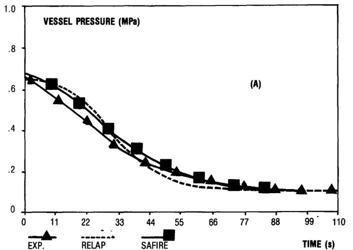
Fig. 12 - Comparison between SAFIRE, RELAP5 and experimental data concerning the water blowdown test "3" performed with the MPMC-TF
