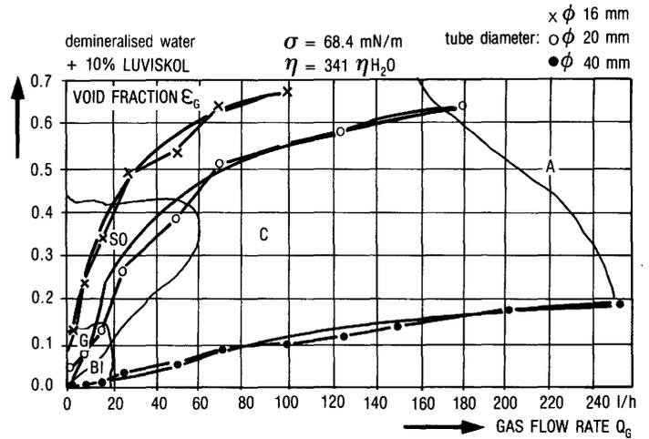
Fig. 5 - Void Fraction Versus Gas Flow Rate
