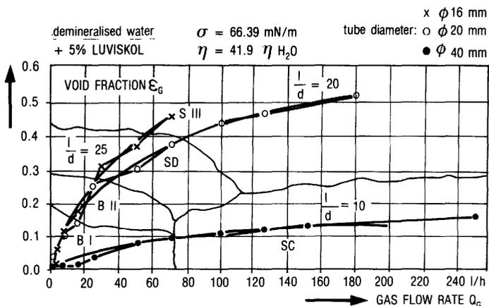
Fig. 4 - Void Fraction Versus Gas Flow Rate
