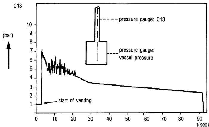
Fig. 8 - Depressurisation history (pressure in the test section, pressure gauge C13)
