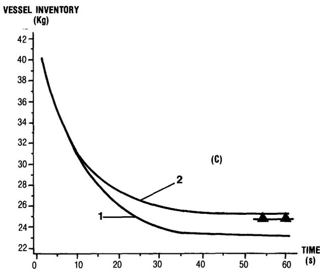
Fig. 11 - Comparison between SAFIRE calculations and measured data concerning the water blowdown test "2" performed with the MPMC-TF
