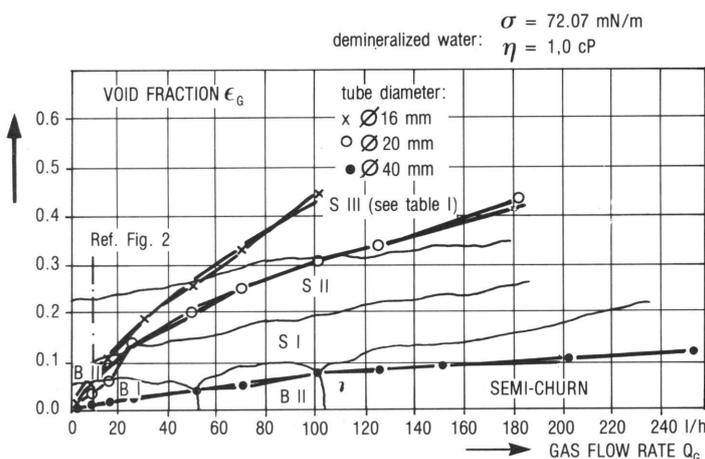
Fig. 1 - Void Fraction Versus Gas Flow Rate
