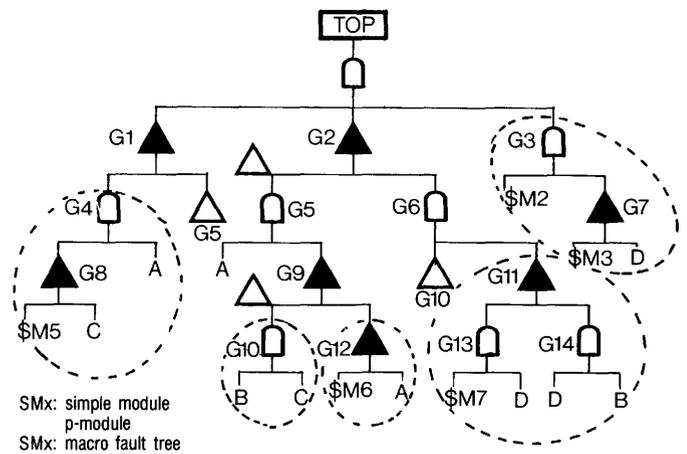
Fig. 1 - Example of pseudo module and macro fault tree generation
