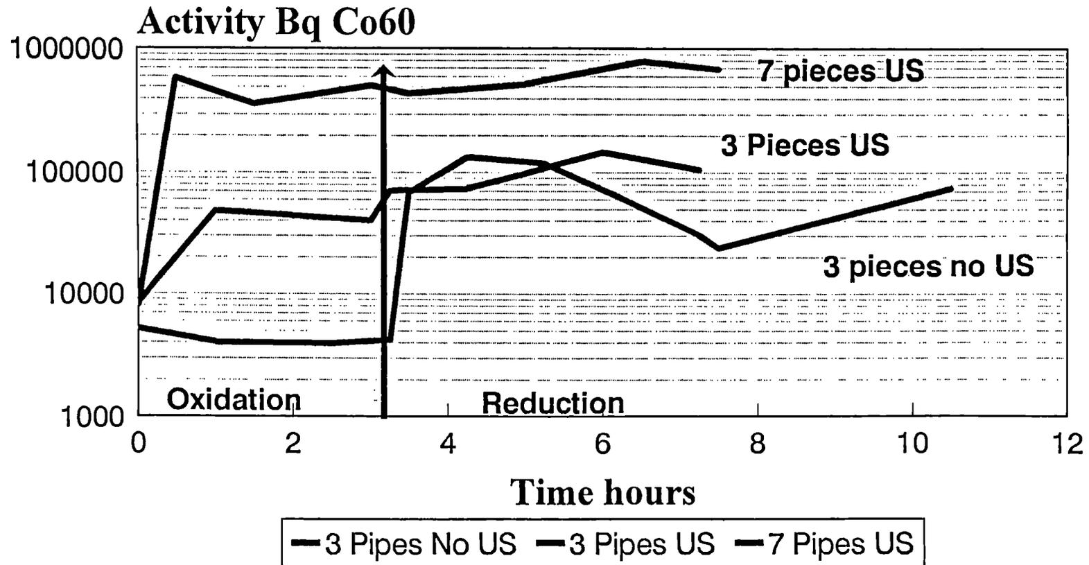
Fig. 4: Decontamination of 3 pieces 1" - 50 cm length
