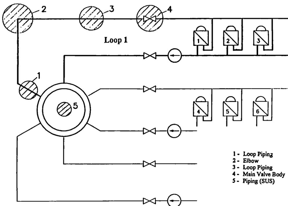
Fig. 1: Location of the Decontaminated Parts during Operation of VVER 70
