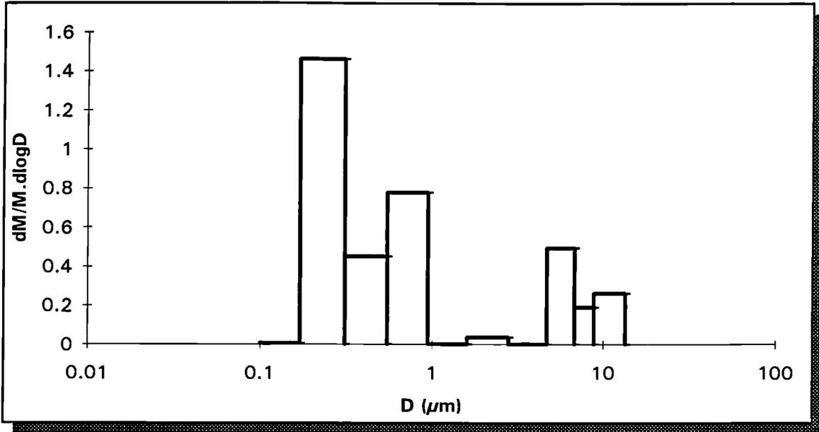
FIGURE 3: S.D.I. sampling - particle size distribution carbon steel experiments
