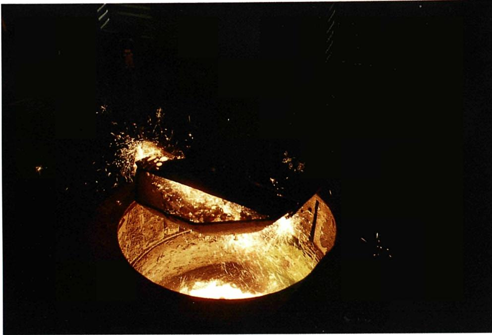
Picture 5. Slag removal sequence (2)
