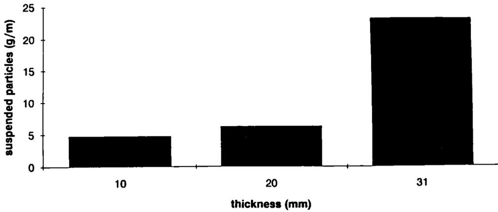
Figure 4 : Variation of the suspended particles v.s. sample thickness
