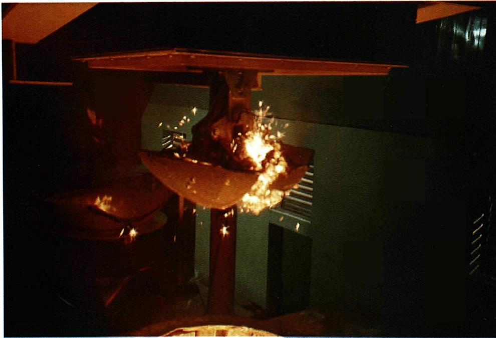
Picture 6. Slag removal sequence (3)
