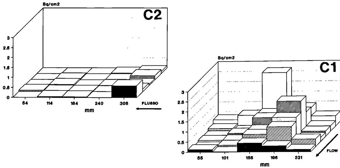
Fig. 5 Residual activity distribution on pipe C-1 and C-2.
