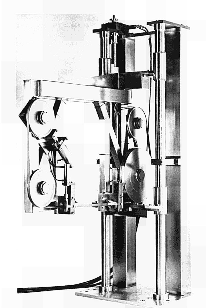
Figure 3 - Underwater band saw machine
