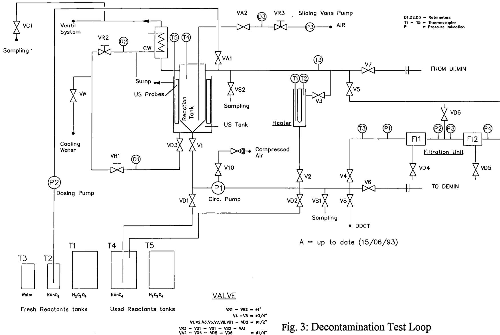
Fig. 3: Decontamination Test Loop
