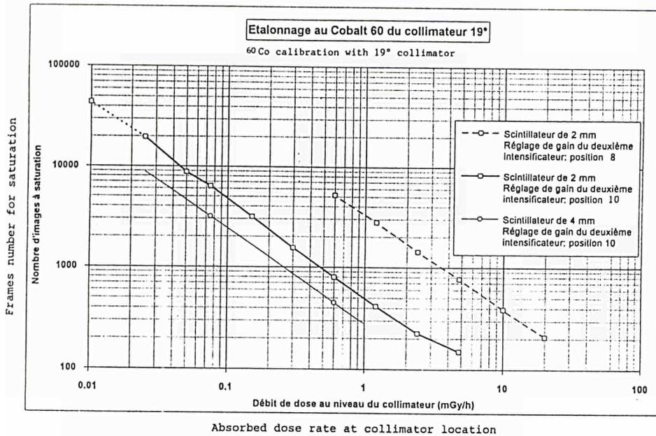
Figure 4 : Experimental results of linearity tests with <sup>60</sup>Co
