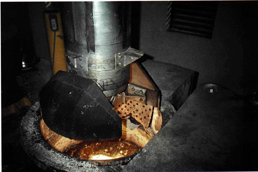
Picture 4. Slag removal sequence (1)
