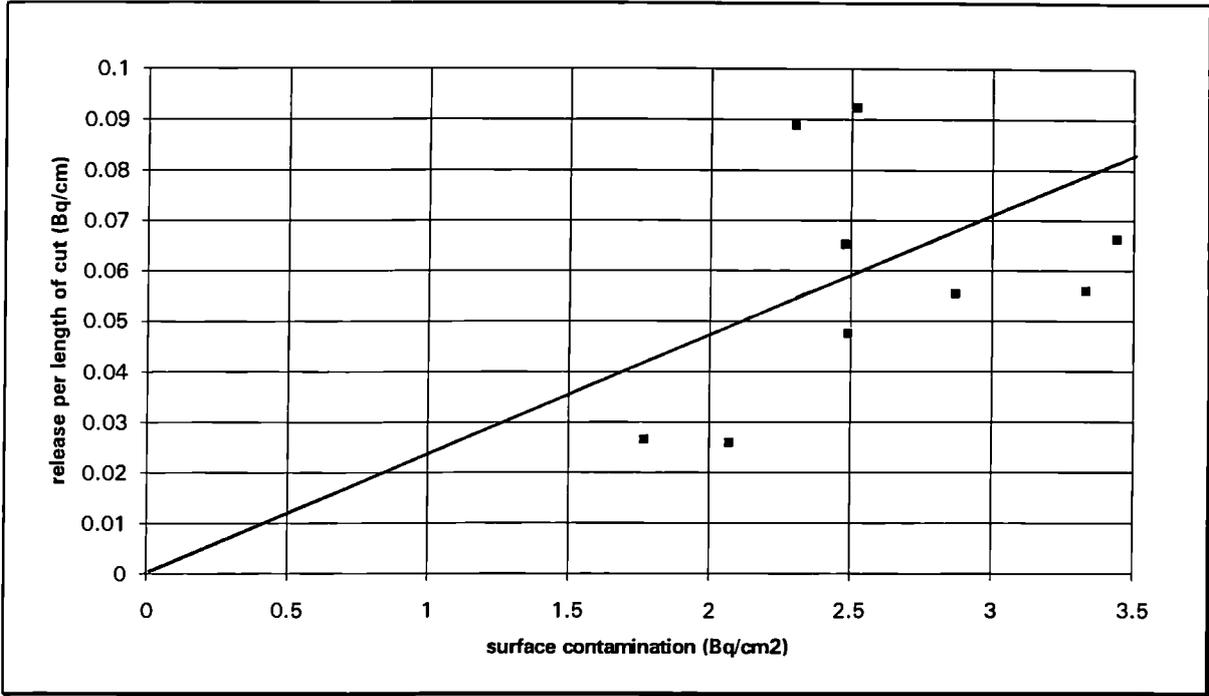
FIGURE 5 : Radioactivity release during thermal cutting of austenitic material contaminated with  $UO_2$  powder
