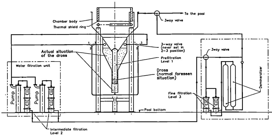
Figure 1 - Flooded chamber for plasma cutting (lower part only)
