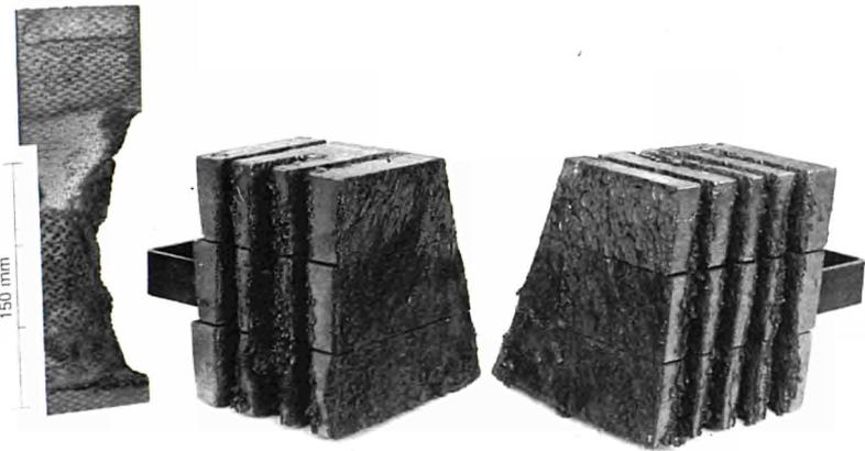
**Figure 2 : Result of cutting 150mm of stainless steel plate with the CAMC tool**
