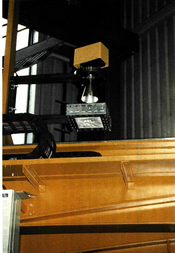
Picture 2. Bath level measuring device
