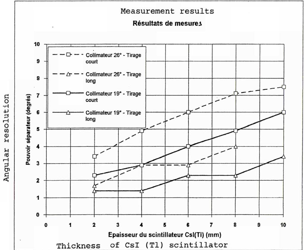
Figure 3 : Measurement results of angular resolution
