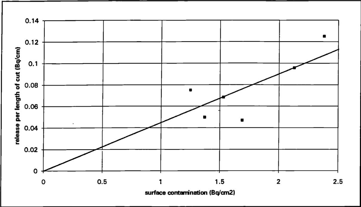
FIGURE 7 : Radioactivity release during thermal cutting of ferritic material contaminated with UO<sub>2</sub> powder
