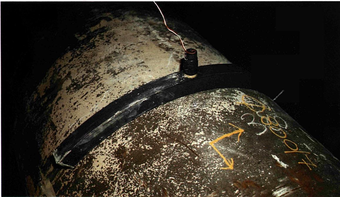
Figure 3 : Cutting tests with Nitroroc explosive
