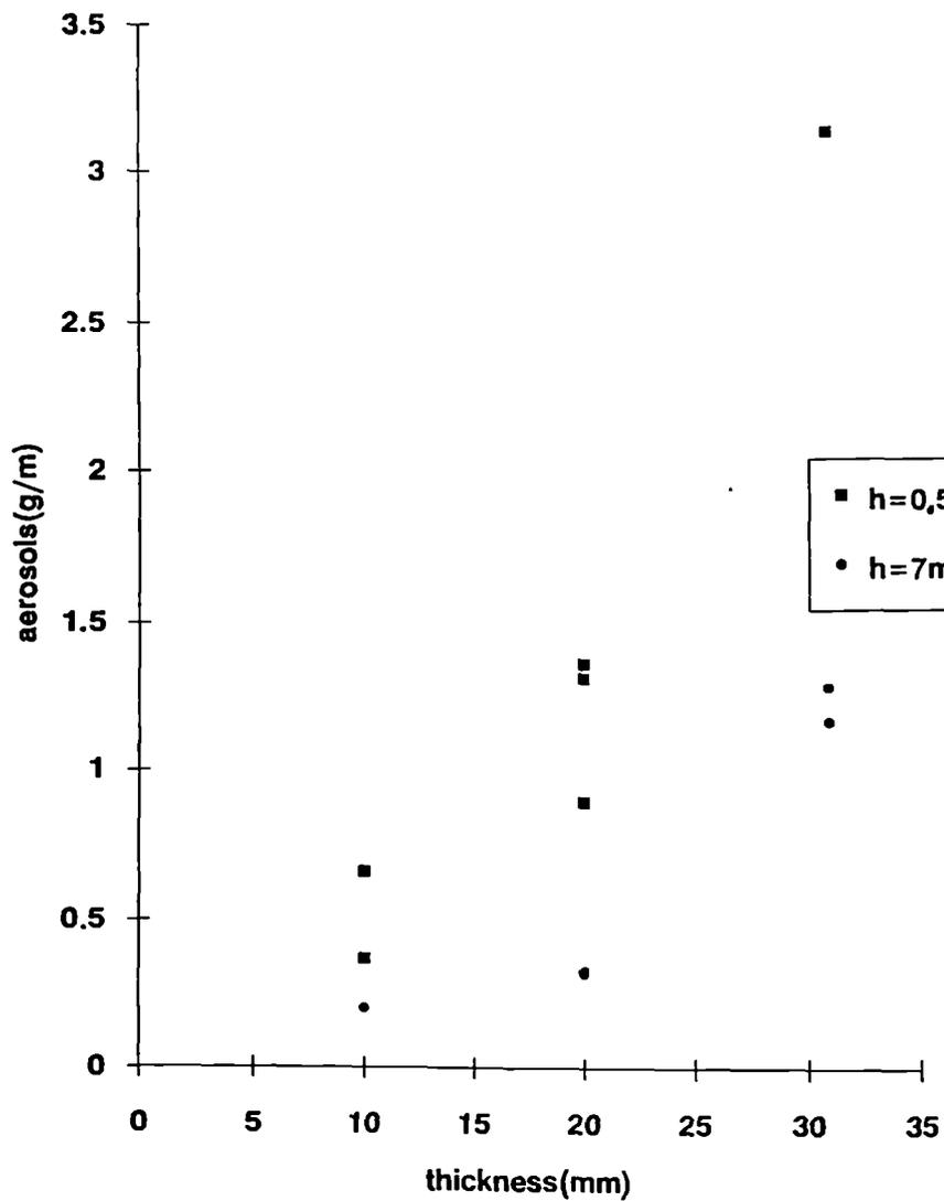
Figure 3 : Variation of the aerosols mass v.s. plate thickness
