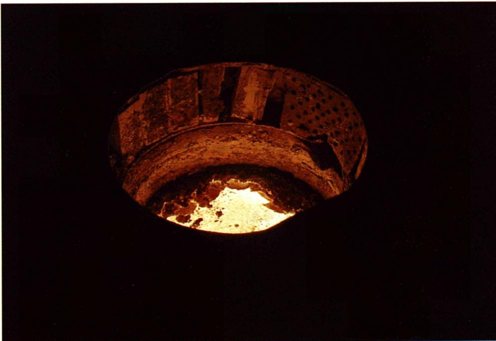
Picture 8. Slag ring formed on the crucible edge
