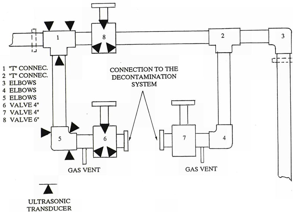
Fig. 2 Scheme of the system selected for the field test at the Garigliano BWR plant
