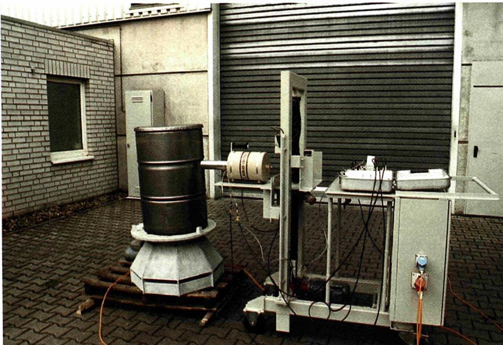
Picture 4. Barrel scanner for drum activity level determination
