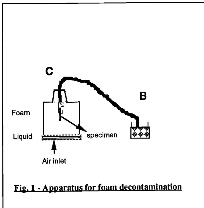
**Fig. 1 - Apparatus for foam decontamination**
