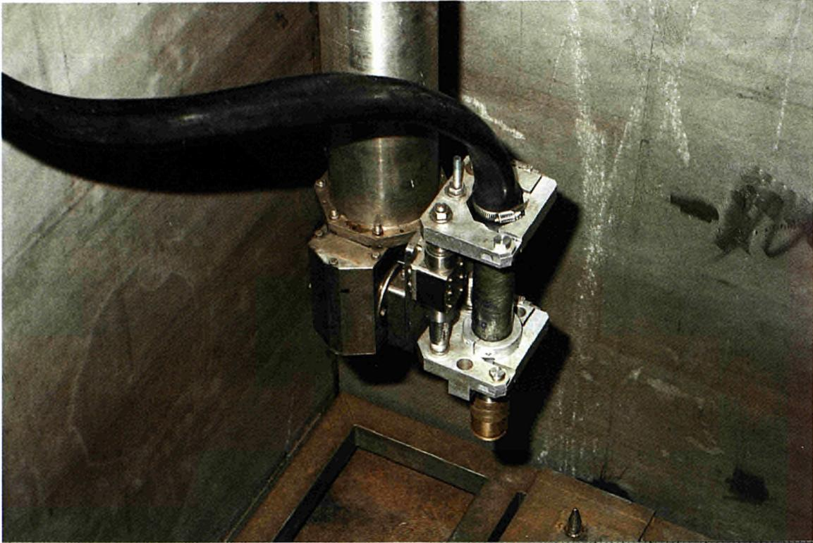
**Figure 1 : The L'TEC plasma torch in the empty tank**
