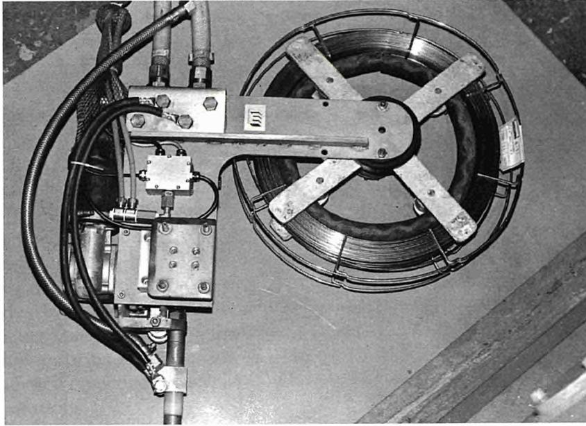
**Figure 3 : Consumable electrode tool ready for use in the Pegase facility**
