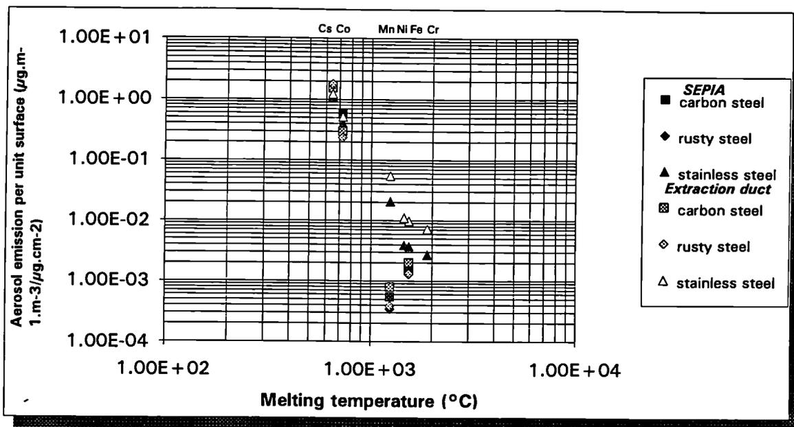
FIGURE 1 : Aerosol emission against melting temperatures (SEPIA sampling inside the test cubicle and extraction duct filter sampling)
