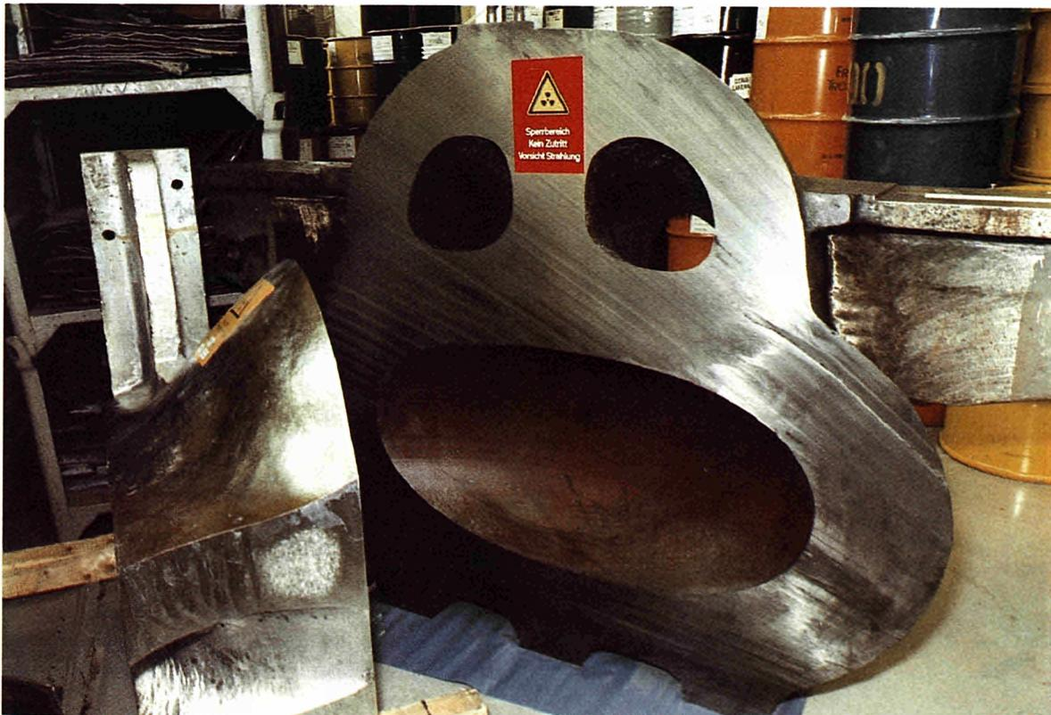
Figure 3: Post-segmenting of the recirculation pump by sawing
