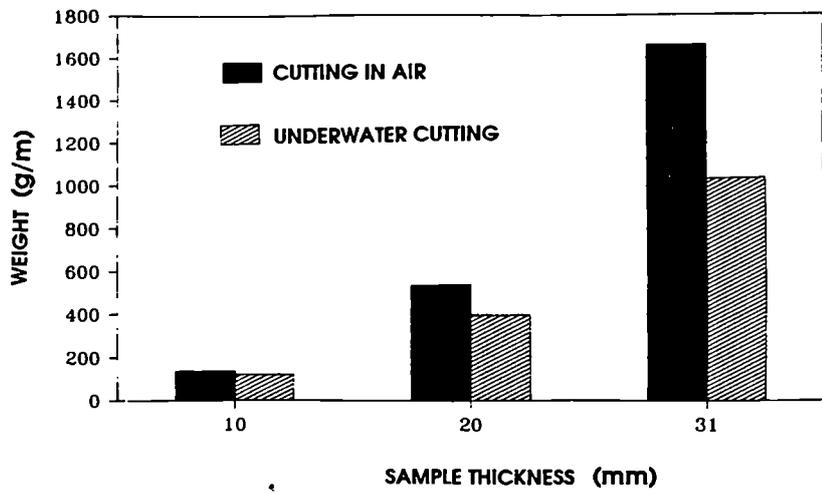
Figure 5 : Sedimented gross mass v.s. plate thickness
