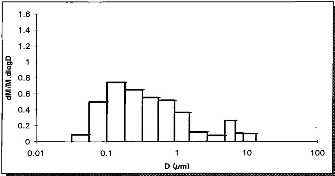
FIGURE 4 : S.D.I. sampling - particle size distribution stainless steel experiments
