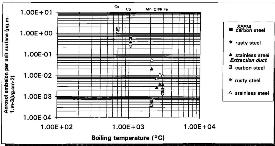
FIGURE 2 : Aerosol emission against boiling temperatures (SEPIA sampling inside the test cubicle and extraction duct filter sampling)
