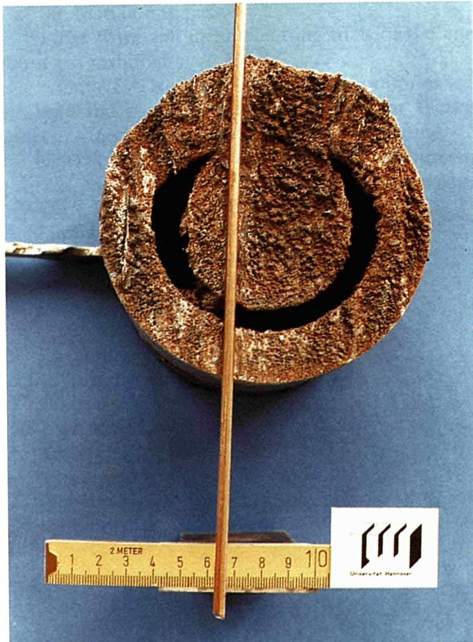
**Figure 4 : Result of cutting the "tube" model with the consumable electrode tool**
