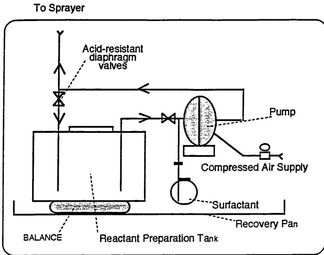
Figure 1: Simplified foam generating unit
