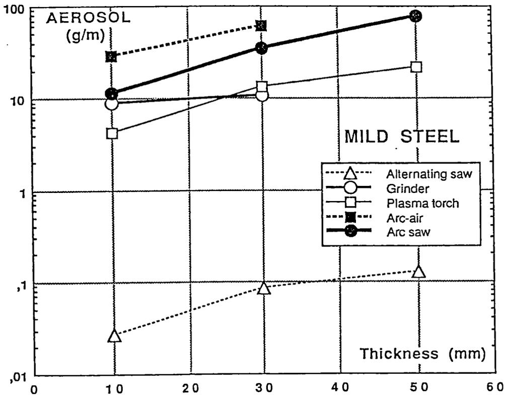
Figure 3: Aerosol production for five cutting tools versus the thickness of the mild steel plate
