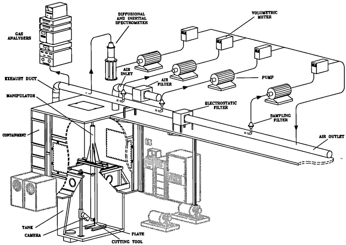
**Figure 5 : Overall view of the experimental device for gas analysis and aerosol measurement.**
