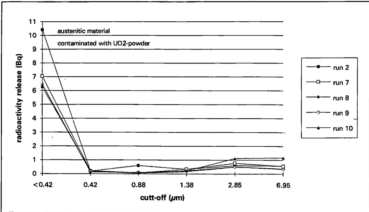
FIGURE 8 : Particle size distribution
