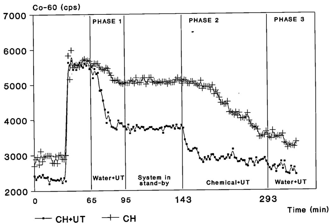
Fig. 4 On-line monitoring of the the activity on pipe C-1 and C-2 during the test
