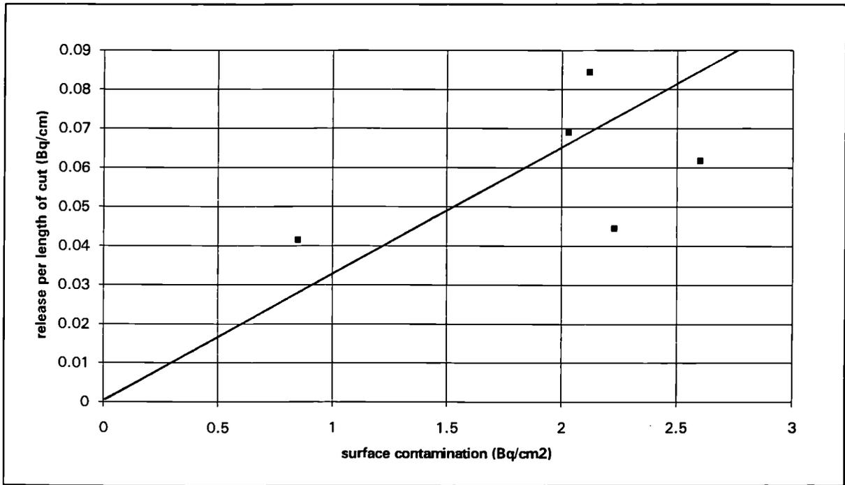
FIGURE 6 : Radioactivity release during thermal cutting of austenitic material contaminated with U-nitrate
