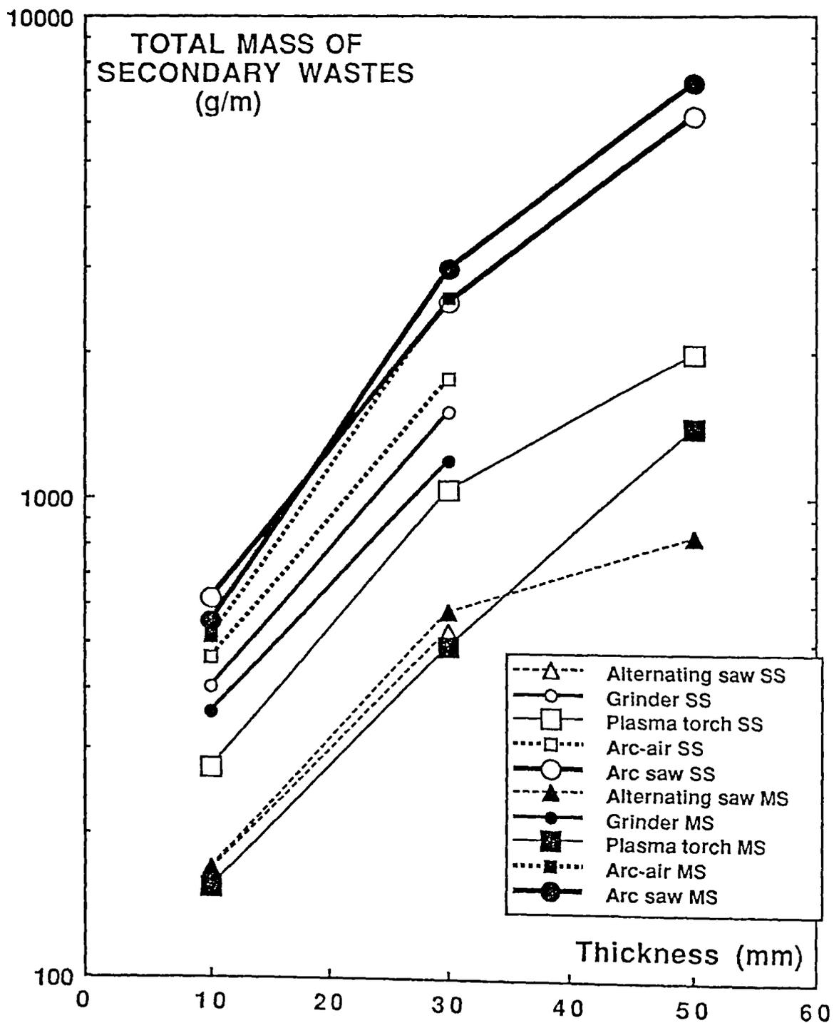
Figure 1: Total mass of secondary wastes produced by five cutting tools versus the thickness of the stainless (SS) and mild steel (MS) plates
