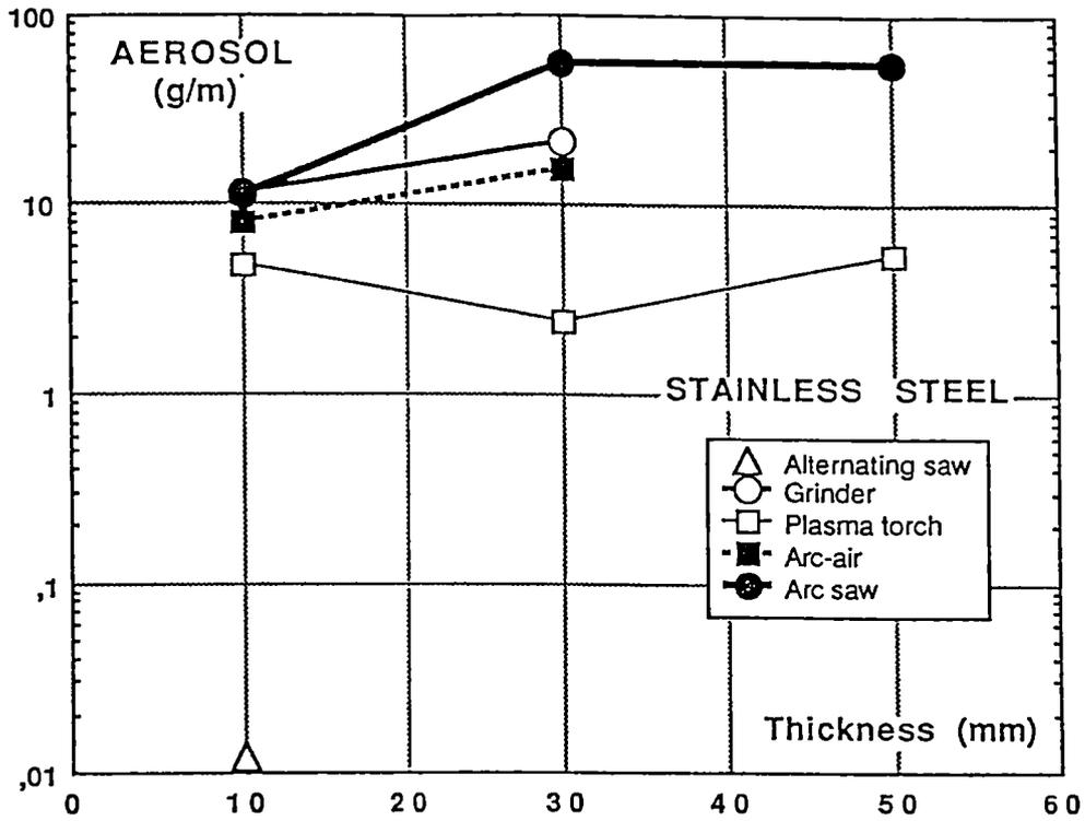
Figure 2: Aerosol production for five cutting tools versus the thickness of the stainless steel plate
