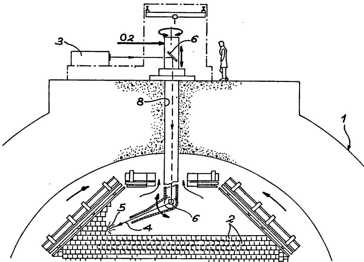
Figure: Graphite Destruction by in situ Laser Controlled Incineration
