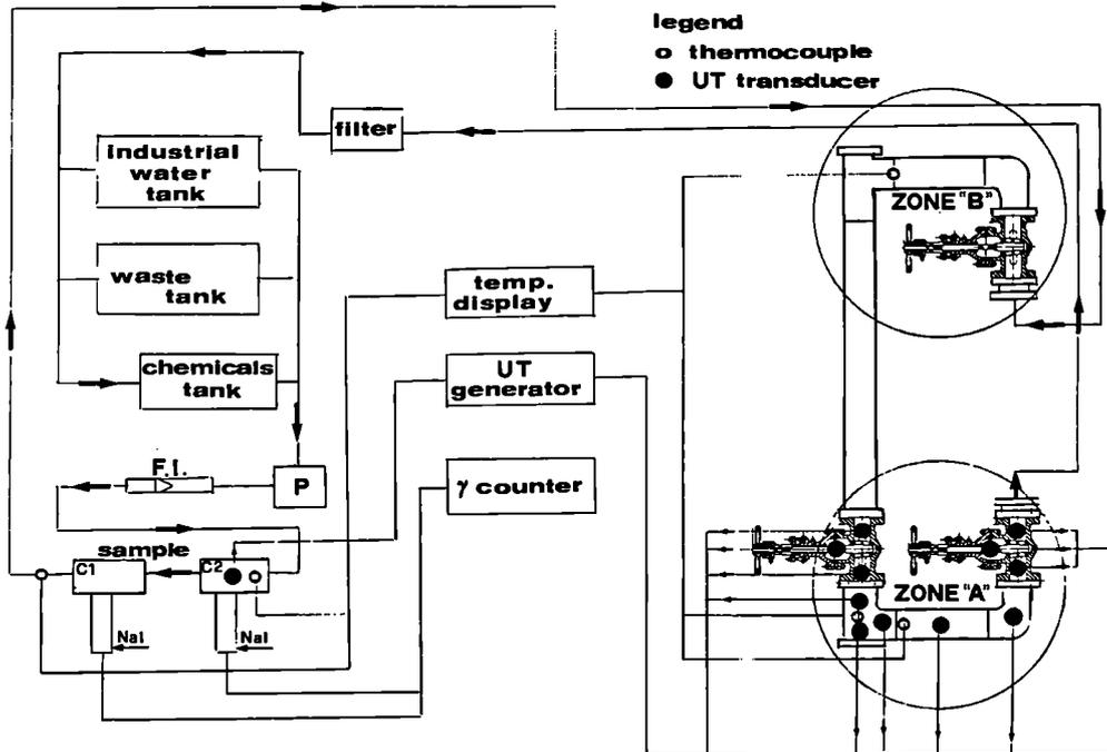
Fig. 3 Operating scheme of the decontamination test at the Garigliano BWR plant
