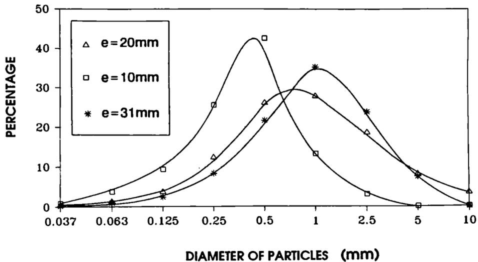
Figure 6 : Sedimented gross size distribution for 10, 20 and 31 mm thickness
