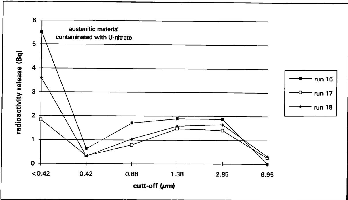
FIGURE 9 : Particle size distribution
