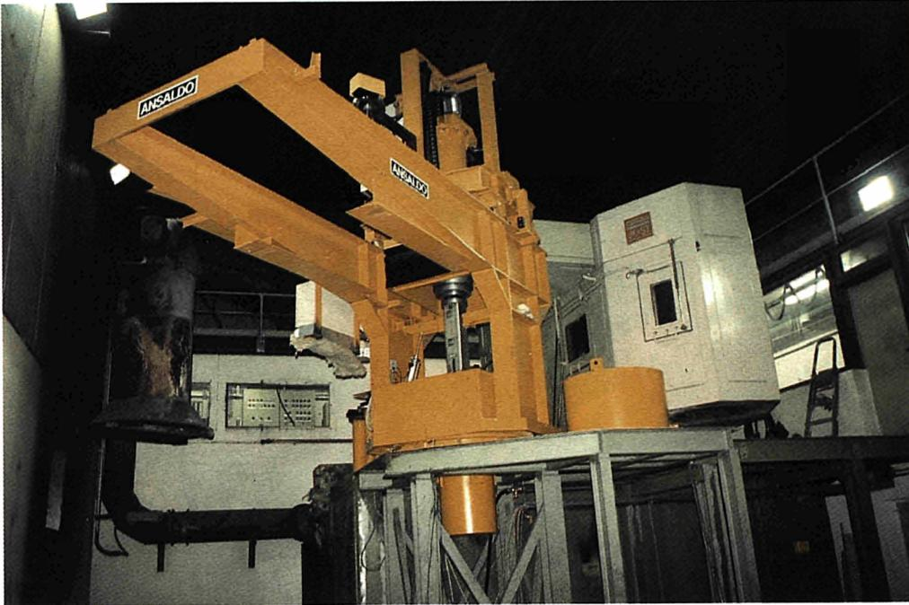
Picture 3. The manipulator installed in CARLA plant
