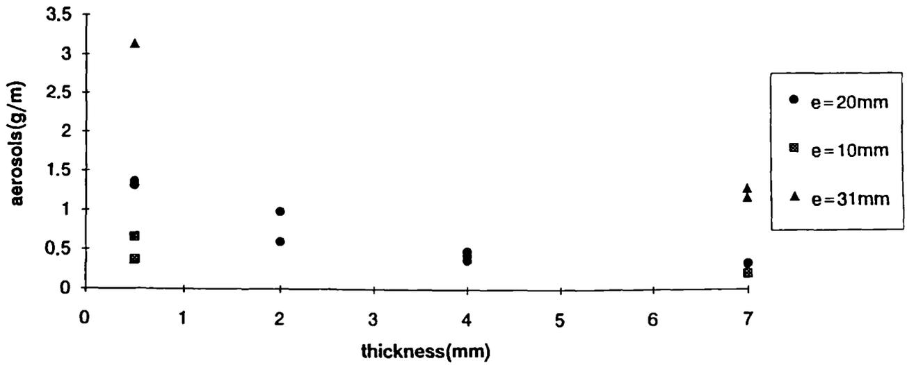
Figure 2 : Variation of the aerosols mass v.s. water depth
