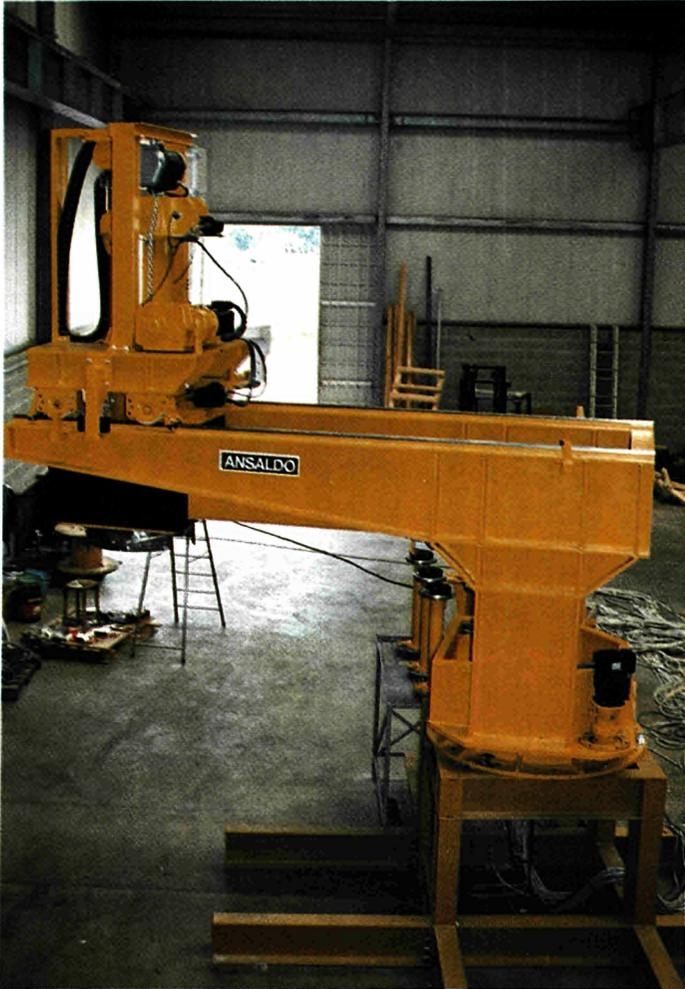
Picture 1. Workshop testing of the manipulator
