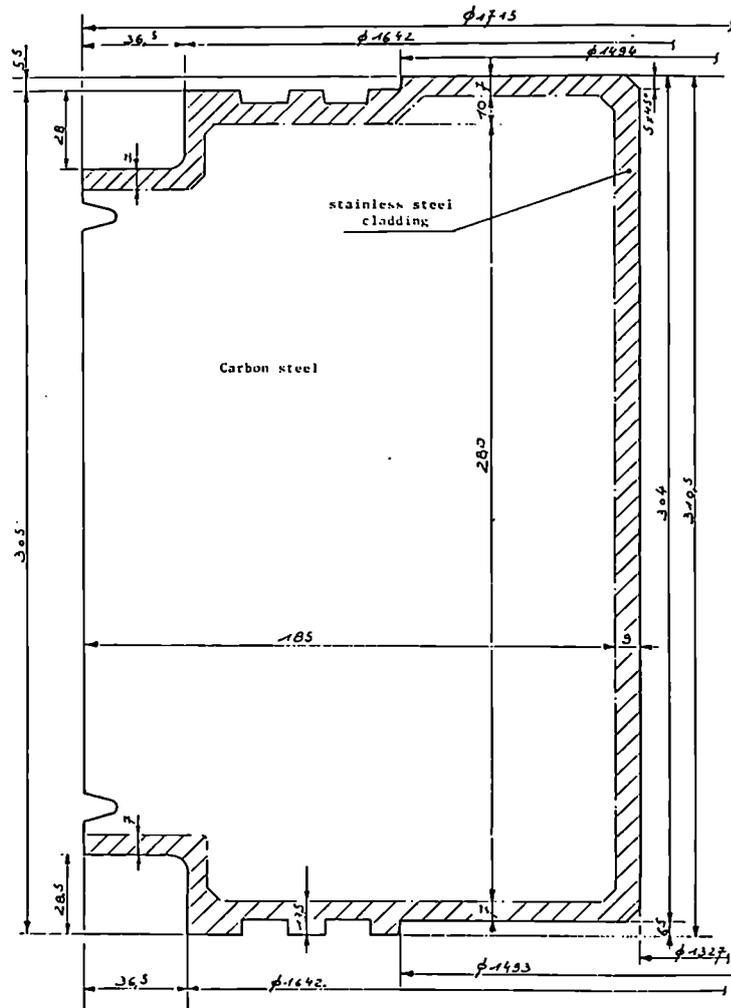
Figure 2 - Cross section of the reactor vessel collar
