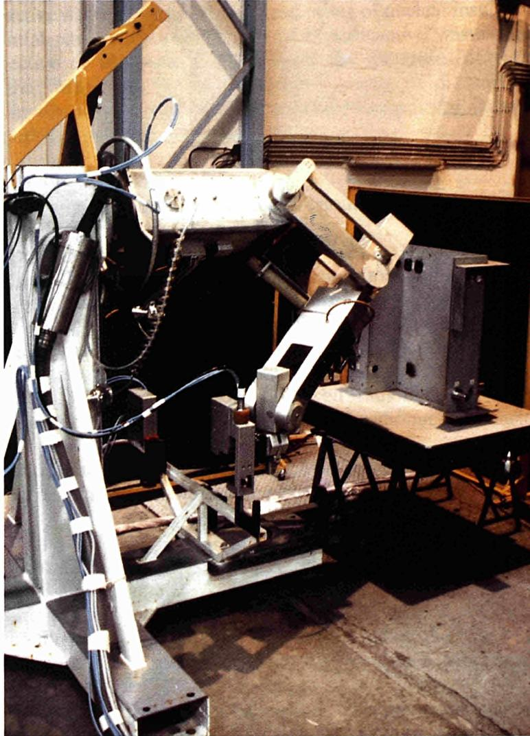
**Fig. 2: RD 500 with its tool rack
