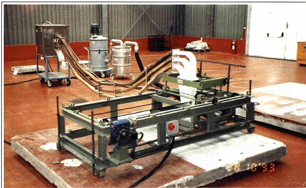
Figure 1 : Flexible wave guides
