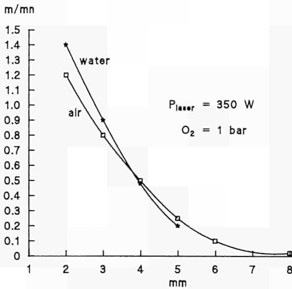
Fig. 4: cutting speed vs. thickness
