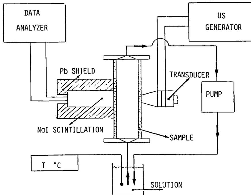
Figure 3 - Flow sheet of the experimental loop for tests with radioactive materials.
