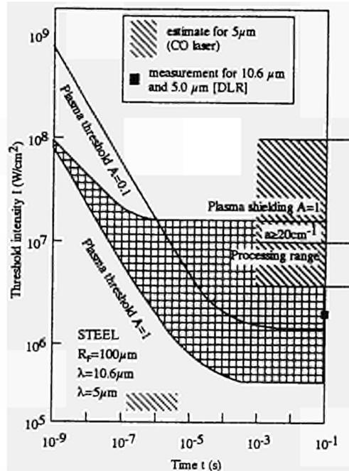
Figure 6. Plasma threshold intensity for steel/argon, calculated after Beyer [2].
