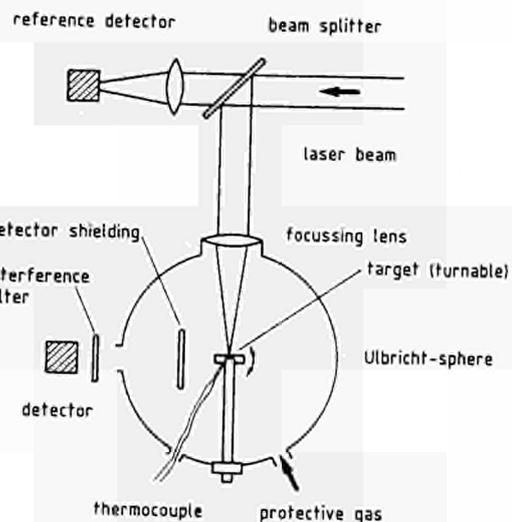
Figure 8. Schematic view of the Ulbricht integrating sphere experimental setup for absorption measurements.
