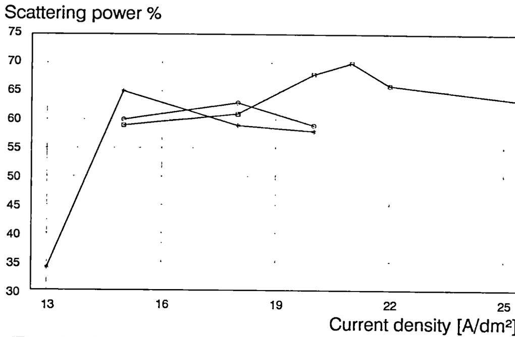
Fig.2: The scattering power as a function of the current density
