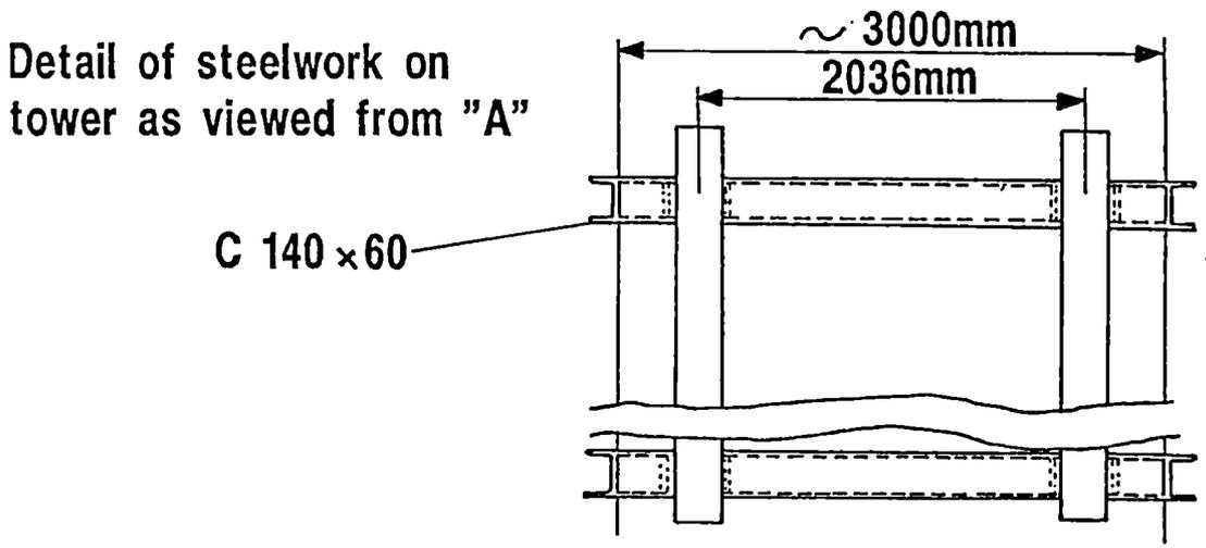
Fig.3: Disposition of testbeds on the concrete tower
