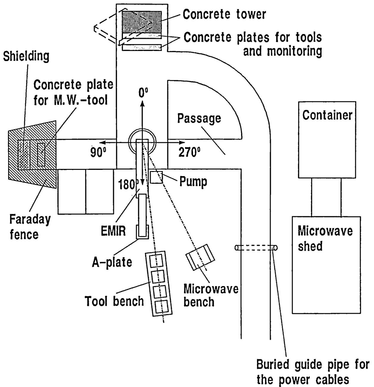
Fig.1: Layout of EMIR site and testbeds
