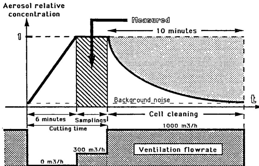
Figure 2 : Second method for sampling aerosols
