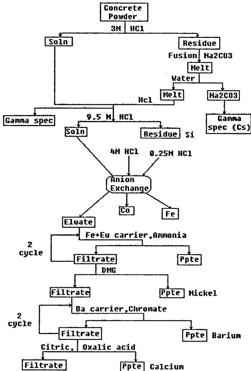
Figure 1. Block Diagram of Separation Scheme
