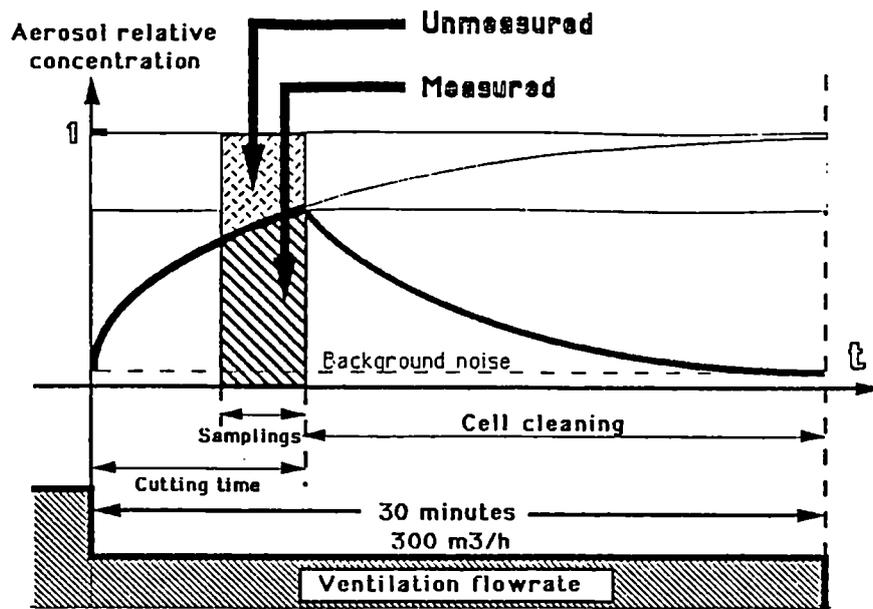
Figure 1 : First method for sampling aerosols
