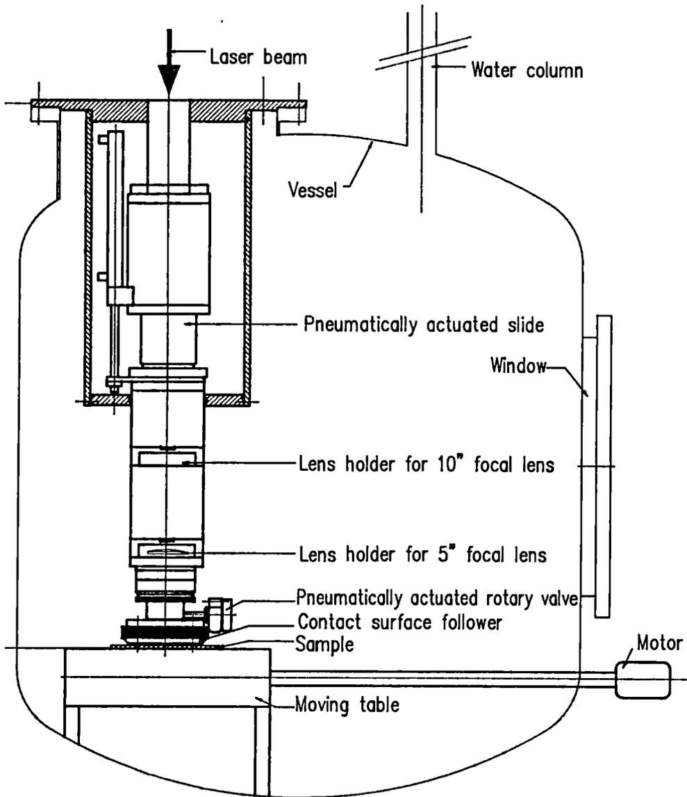
Fig. 2 : Underwater cutting head
