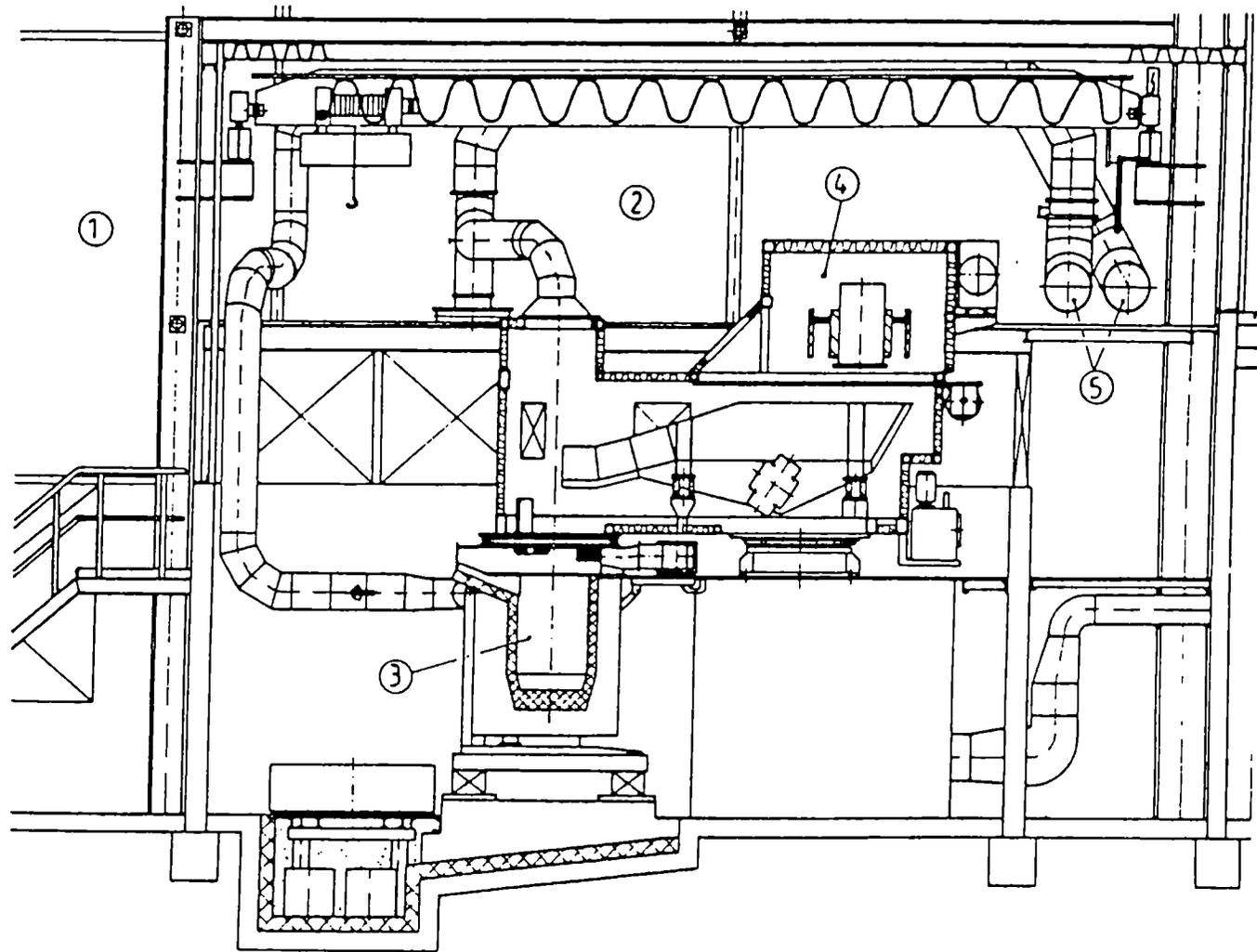
Figure 2: Layout of the new plant - inner housing and furnace.
