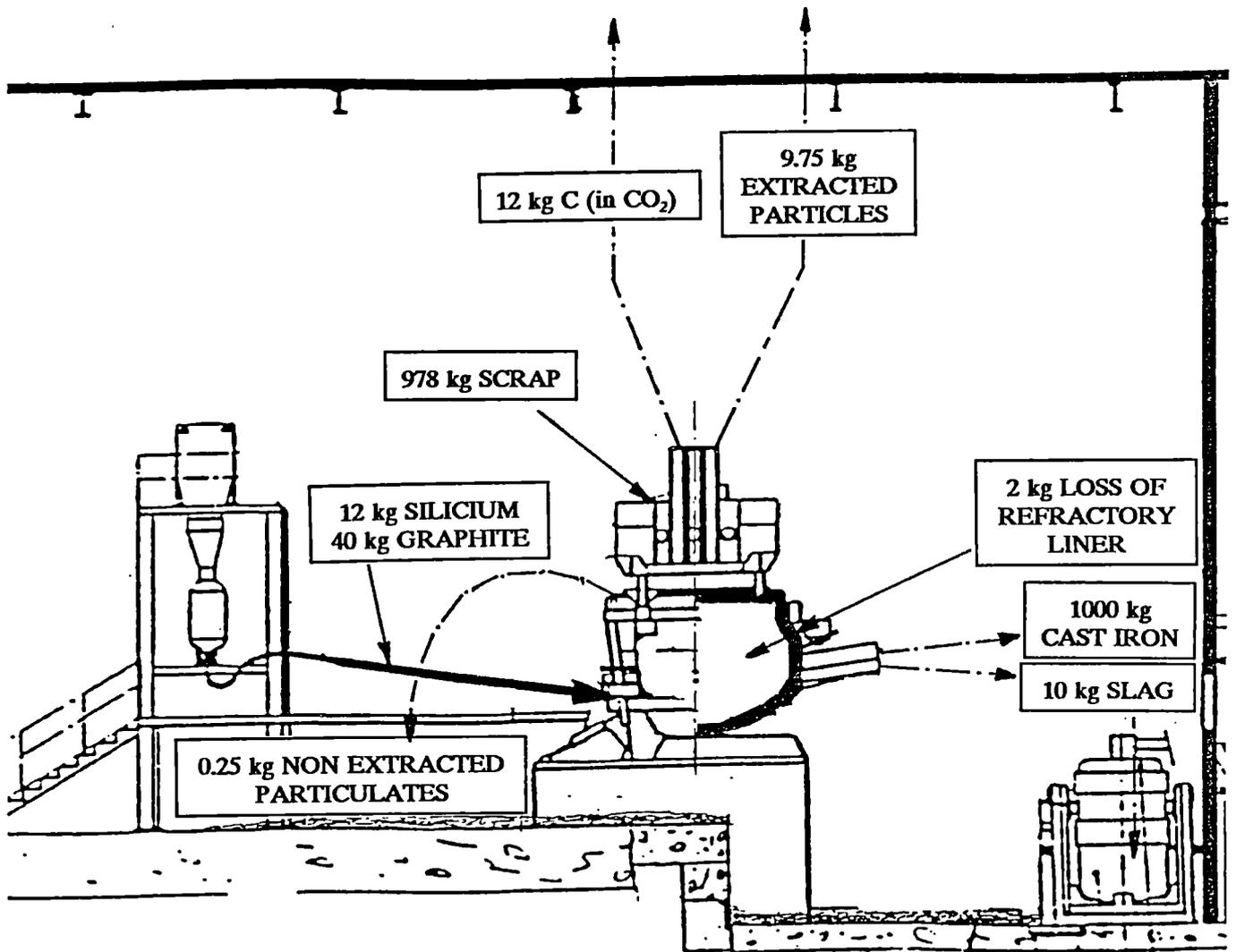
Fig. 1: Mass Balance of the G3 melter
