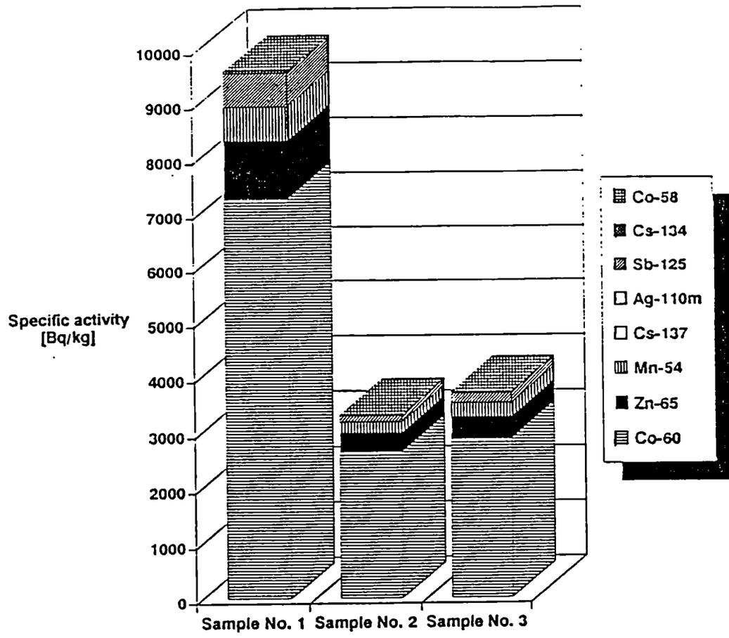
Figure 2: Concrete shielding material samples of a boiling water reactor
