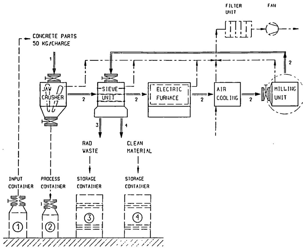
Figure 1: Schematic view of the test installation
