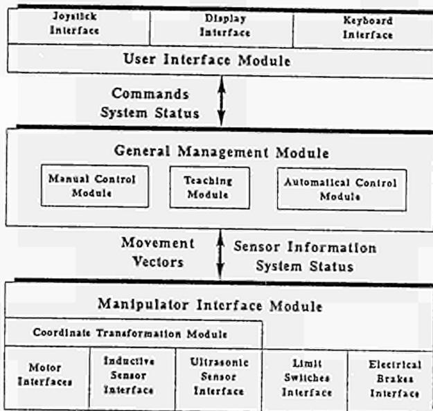
Figure 7 : Software structure and data flow
