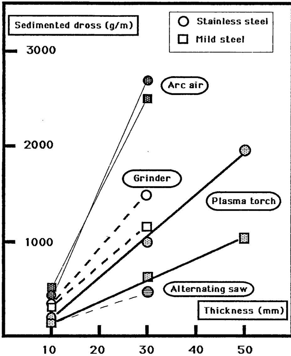
Figure 5 : Sedimented dross production versus the thickness of the plate.
