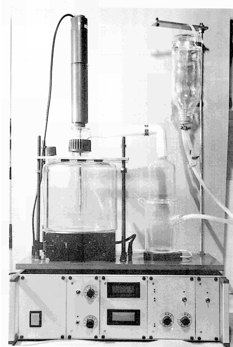
**Figure 2** Experimental set-up for the investigation of film etching using a chemical agent as a fog
