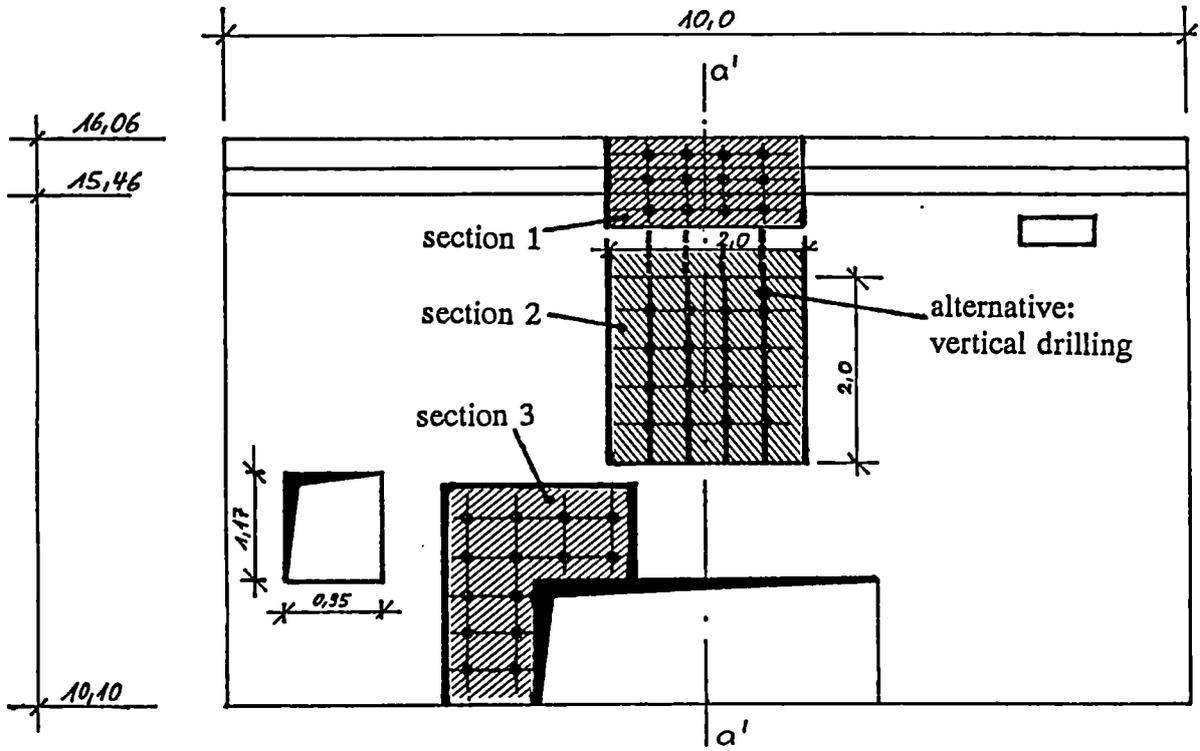
Figure 1: Shield sections for explosive dismantling tests: flattened view
