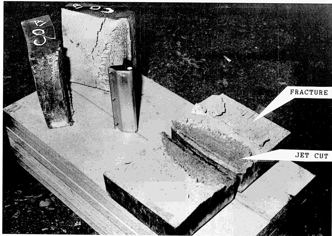
Figure 2: 200mm-THICK STEEL TARGETS
