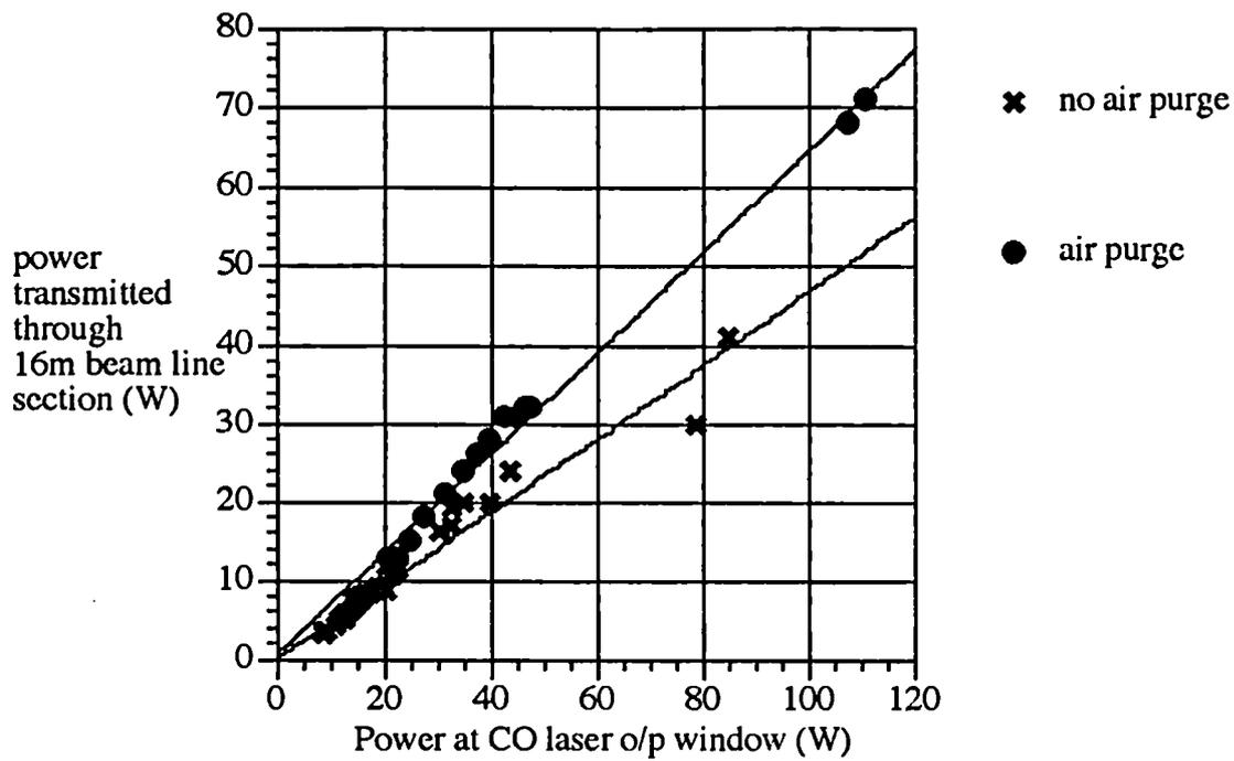
Figure 3. The transmitted power through a 16m long section of the beam line, with and without dry air purge.
