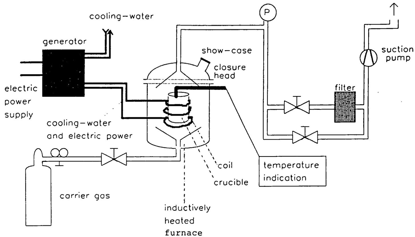
Figure 1: Schematic principle of melting contaminated steel
