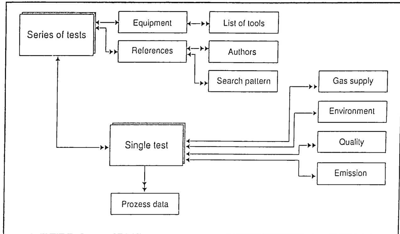
Fig. 1 Basic structure of DB
