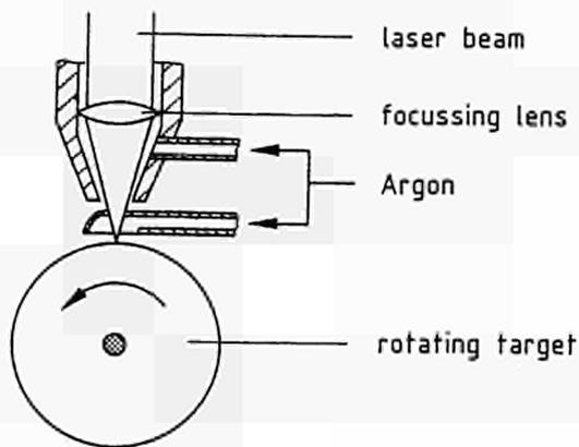
Figure 5. Experimental setup (schematic) for plasma ignition measurements.
