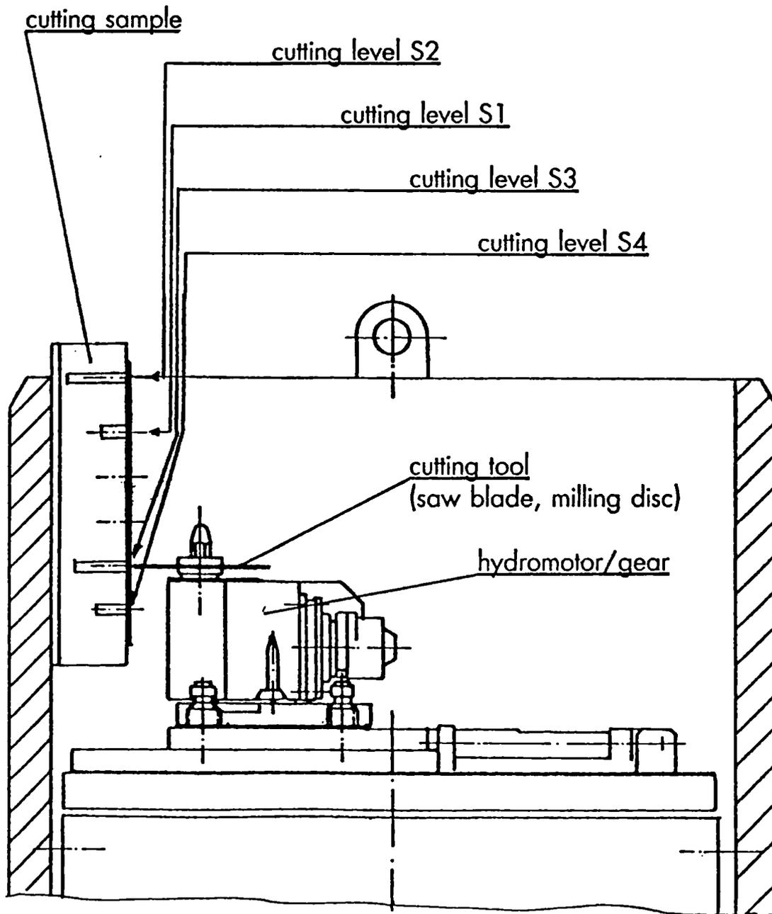
**Figure 1: Underwater milling cutter test**
