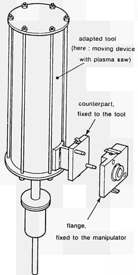
Figure 6 : Principle of connecting different tools to the manipulator
