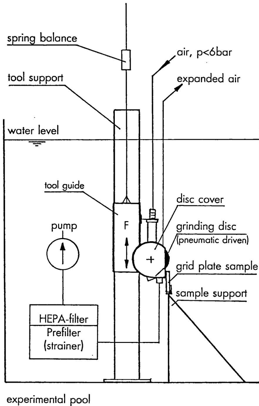
**Figure 3: Underwater grinding cutter test**
