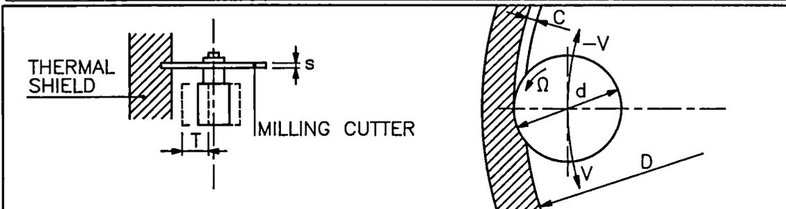
Table IV : EDM for segmentation of thermal shield
