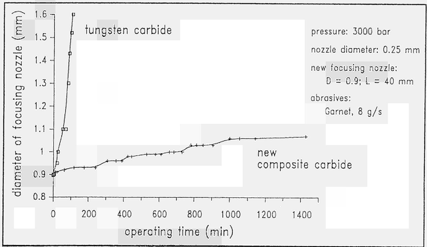
Figure 5 Wear of a new type of focusing nozzles
