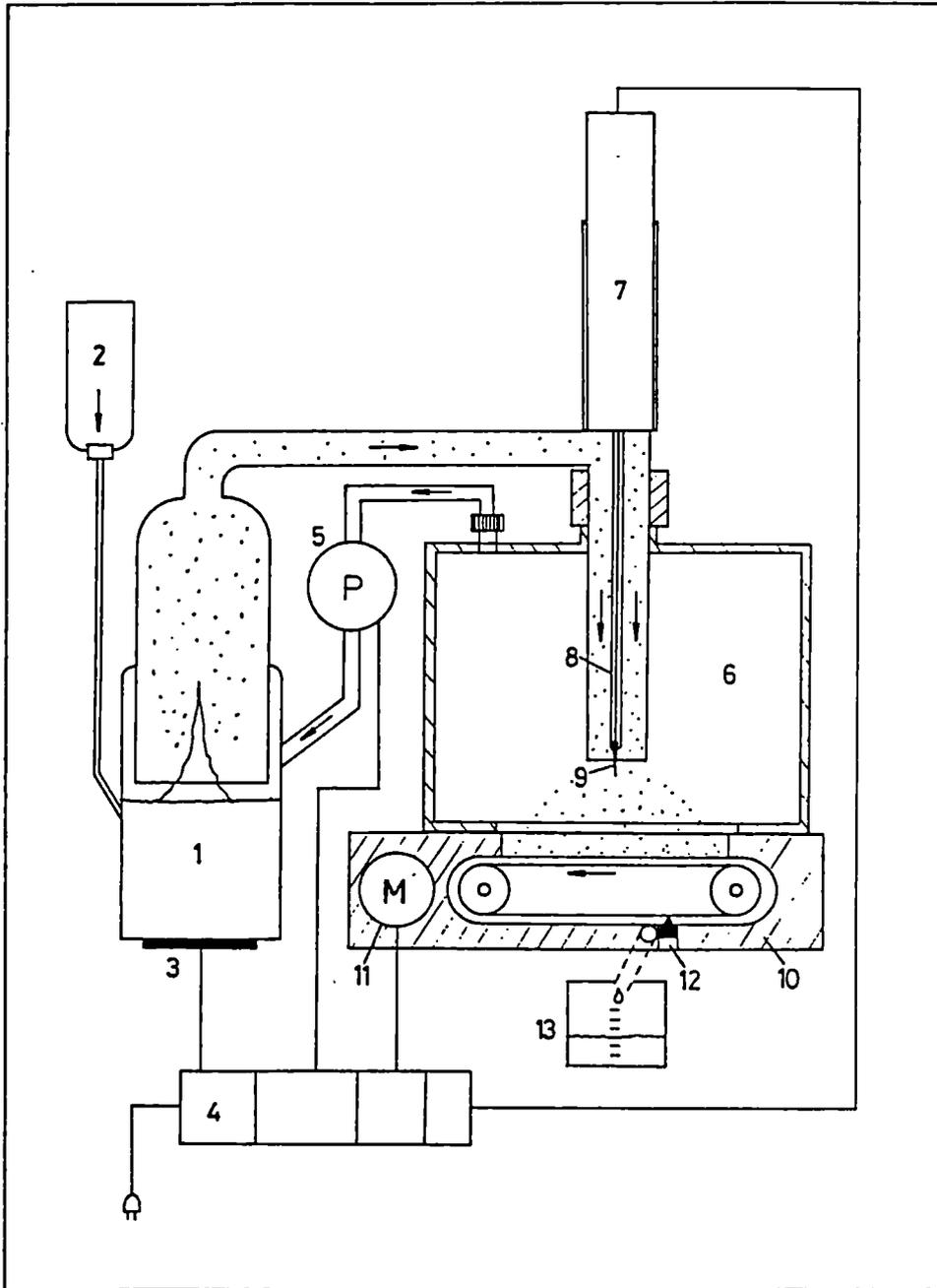
**Figure 1** Principle of the experimental set-up for demonstrating film etching using a chemical agent as a fog
