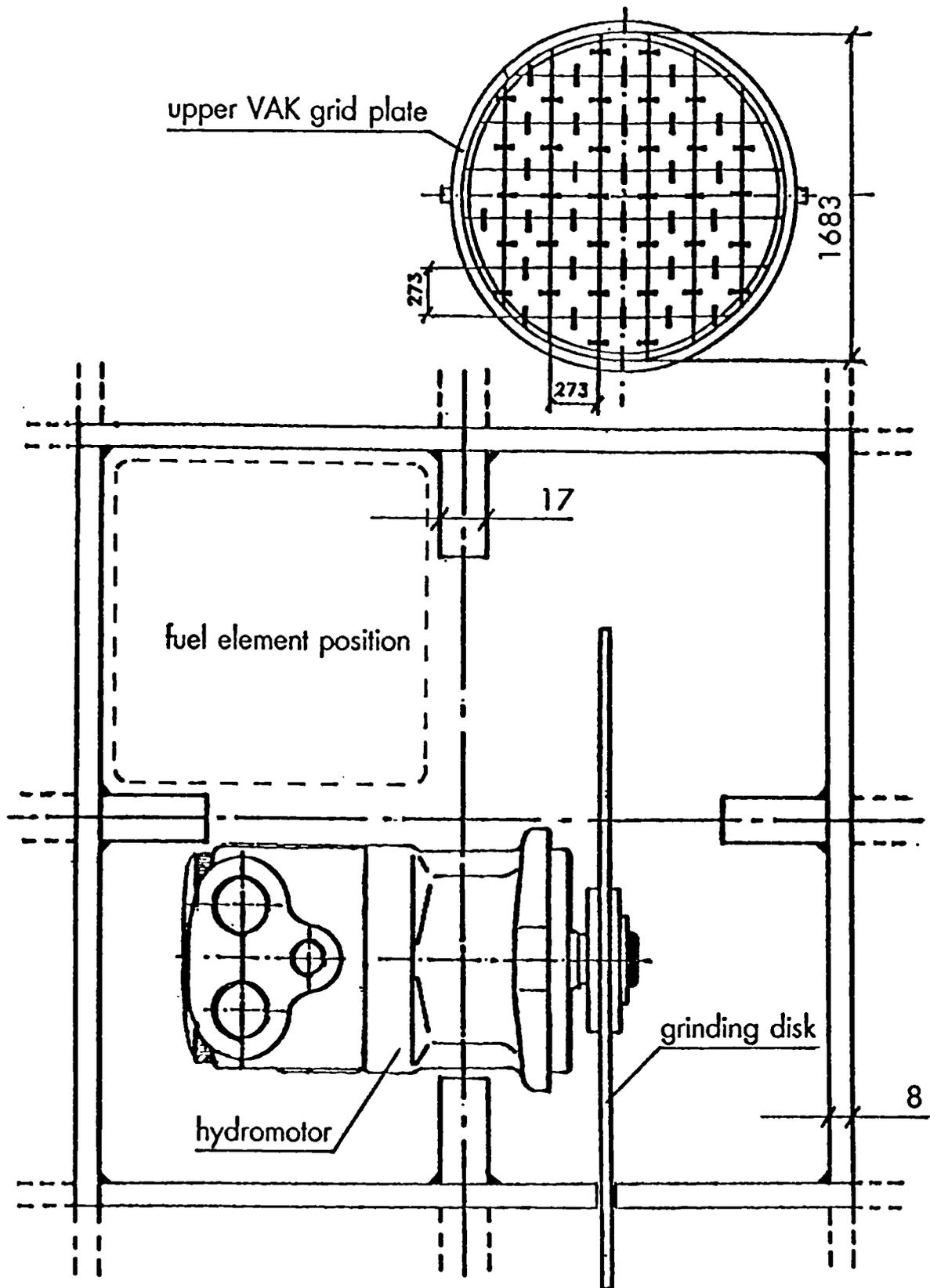
Figure 2: Planned cutting method for upper grid plate
