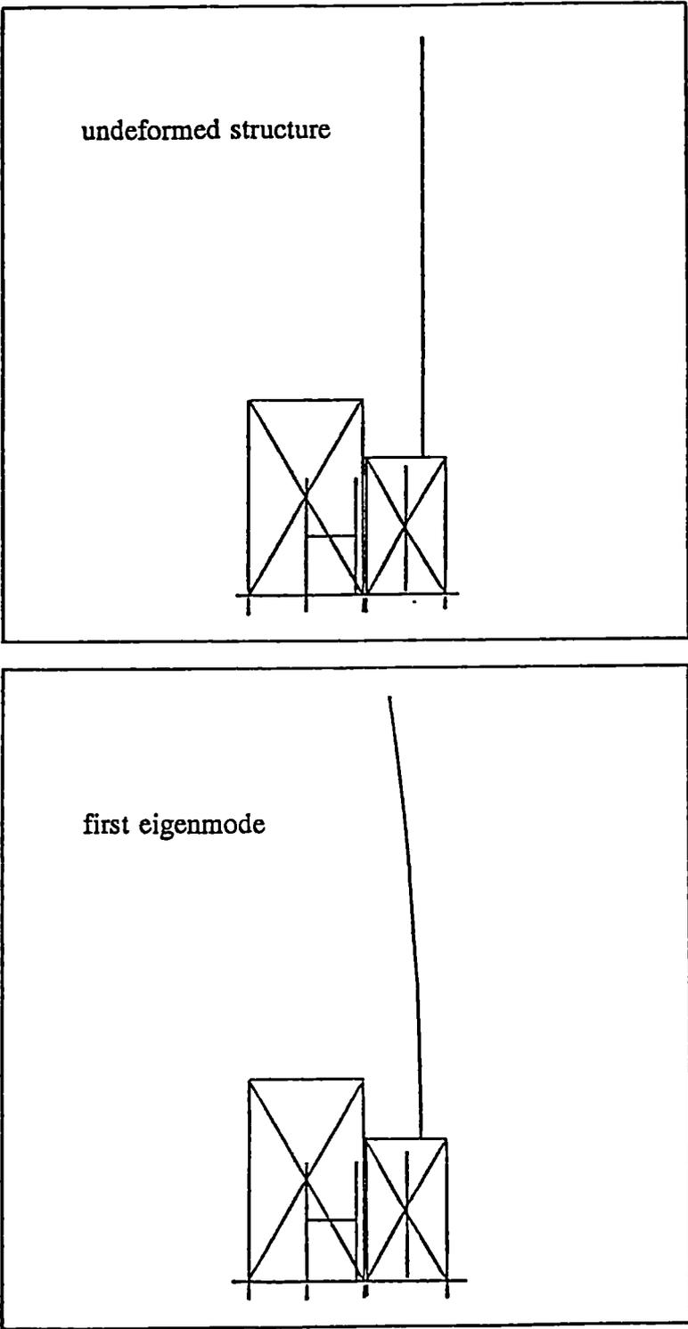
Figure 3: Computer model for reactor and auxiliary building excitation
