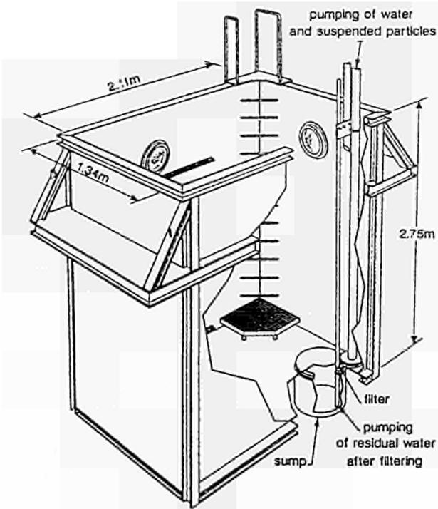
Figure 2 : Drawing of the new tank
