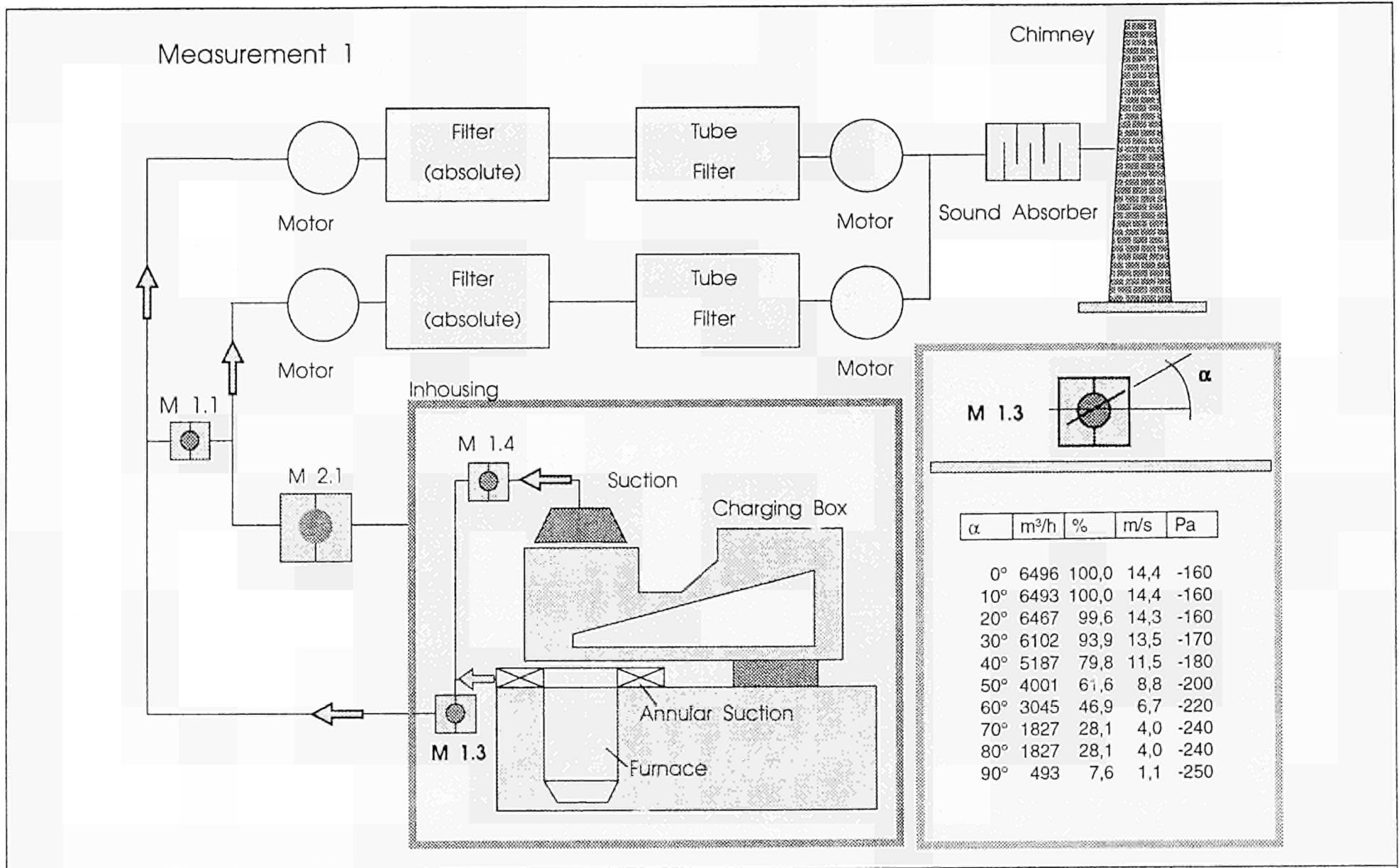
Industrial - scale melting of Tritium containing steel
