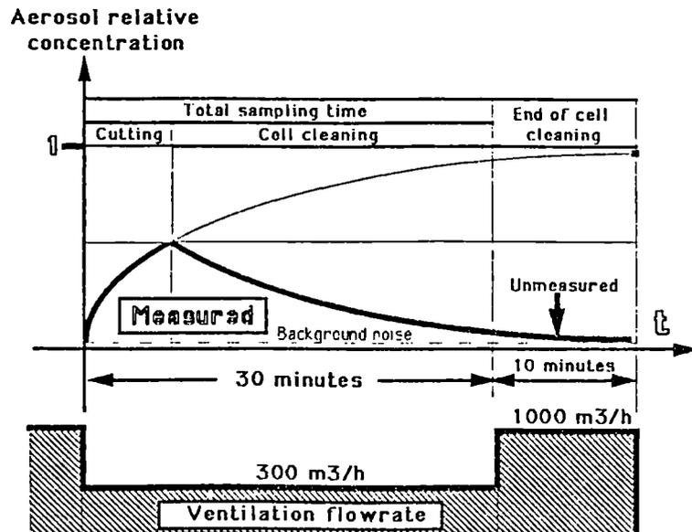
Figure 3 : Third method for sampling aerosols
