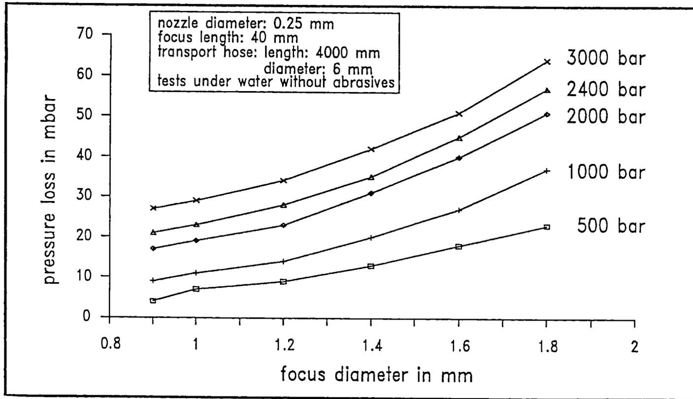
Figure 2 Effect of focus diameter on pressure loss
