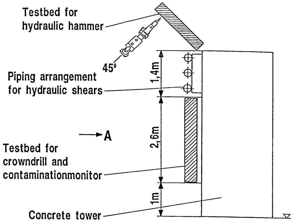
Testbeds mounted on the concrete tower
