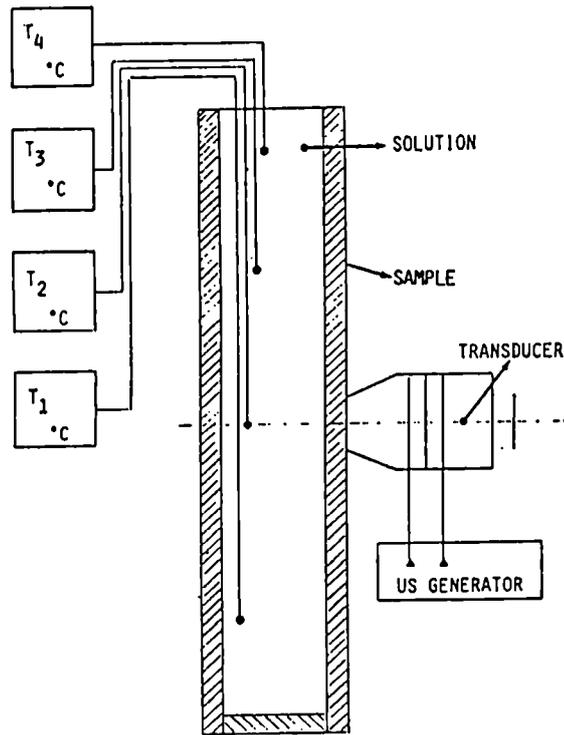
Figure 2 - Experimental device used for static test, on wole pipe.
