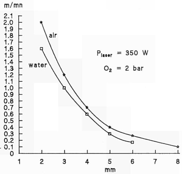
Fig. 5: cutting speed vs. thickness
