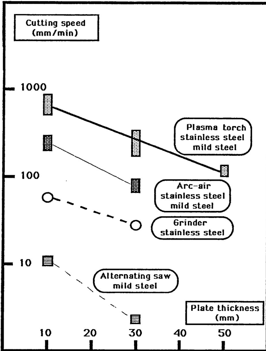
Figure 4 : Optimal cutting speed versus the thickness of stainless steel and mild steel plates for different tools.
