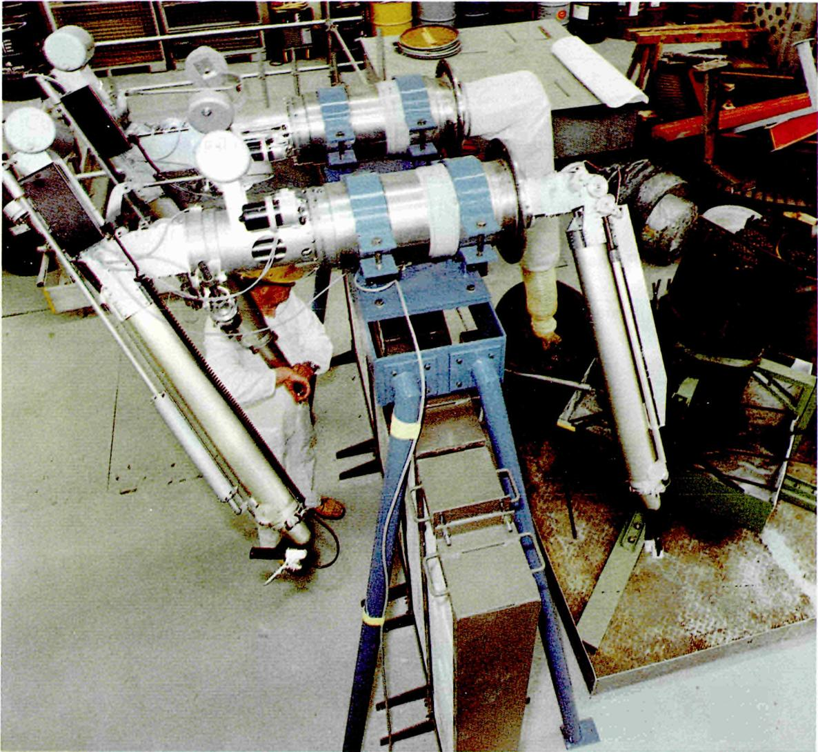
Figure 4: Handling of tubes of the primary clean-up cooler with mechanical master-slave-manipulators
