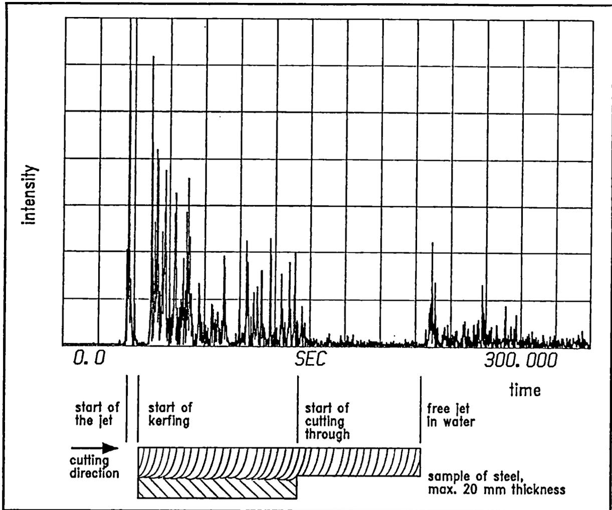
**Figure 4** Detection of kerfing by an accelerometer
