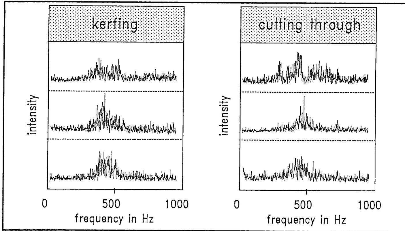
Figure 3 Comparison of sound intensity for cutting and kerfing
