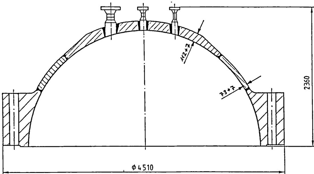
Figure 3: Dimension of the RPV-head
