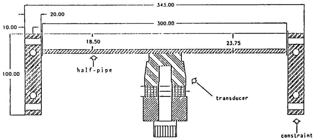
Figure 1 - Frontal view of the experimental devices used for the vibration amplitude tests, on half pipe.
