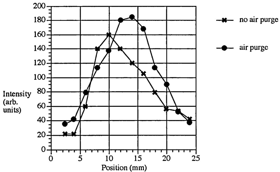
Figure 4. The measured CO laser beam profile after having traversed a 16m long section of beam line, with and without dry air purge.
