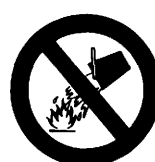
Do not extinguish with water
