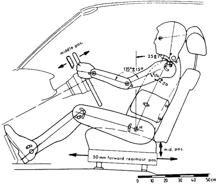
Figure 8: EUROSID positioned in Test Vehicle.
