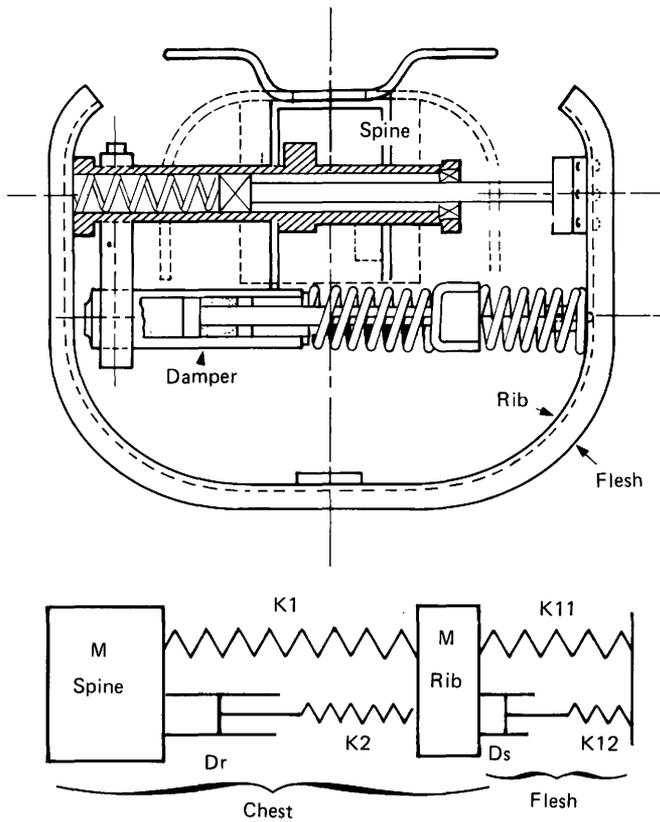
**Fig.3** Diagram of Rib-Piston Module and the Mathematical Model of the Thorax
