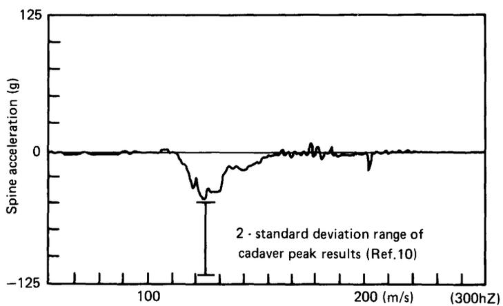
**Fig.15 15mile/h Rigid wall test. Spine acceleration
