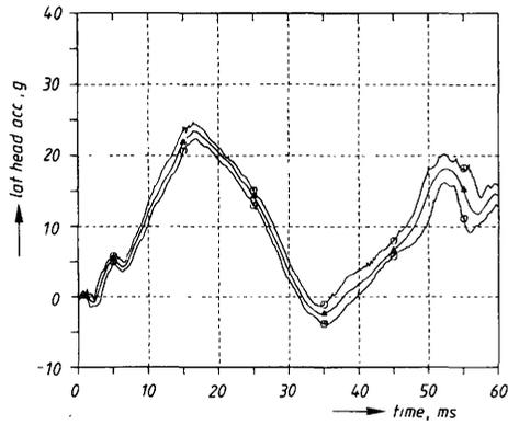
Fig. 5. Lateral head acceleration versus time corridor (o-o), including mean result ( $\Delta$ - $\Delta$ ), obtained from TNO neck repeatability tests.
