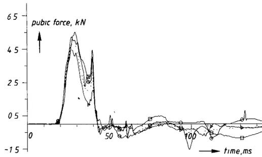
Fig. 31. Pubic symphysis force versus time histories, including mean result (----), obtained from three MDB tests performed by BAST.
