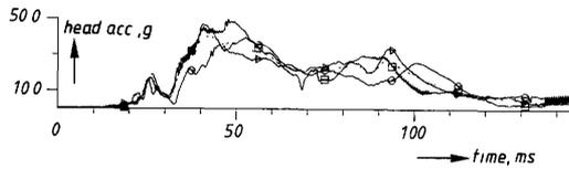
Fig. 26. Resultant head acceleration versus time histories, including mean result (----), obtained from three MDB tests performed by BAST.
