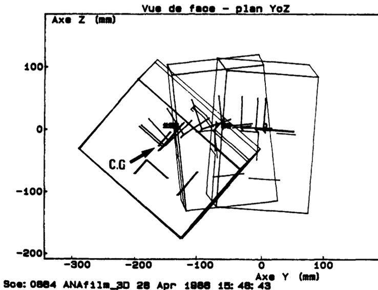
Figure 7 : HEAD KINEMATICS RELATIVE TO THE SLED
