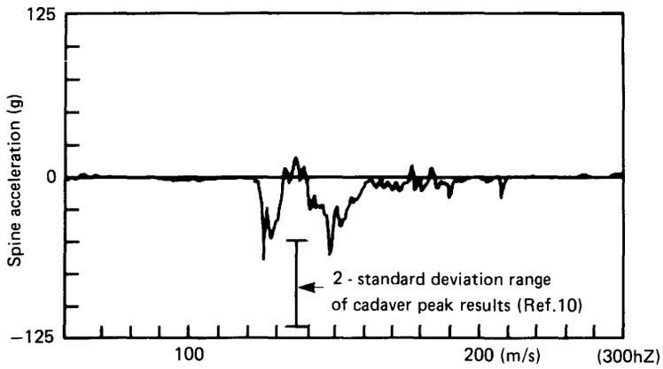
**Fig.13 15mile/h Rigid wall test. Spine acceleration
