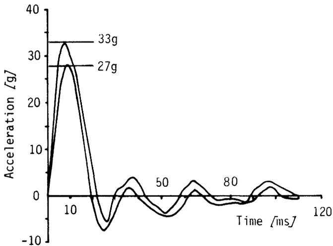
Figure 2: Pendulum acceleration-time corridor
