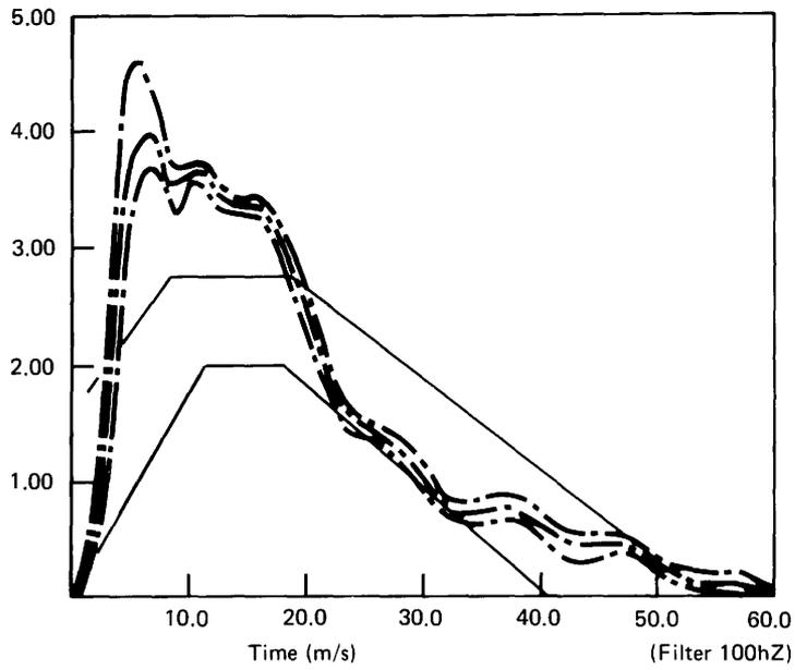
**Fig.5 Force on Thorax produced by a 23.4kg impactor at 4.3m/s**
