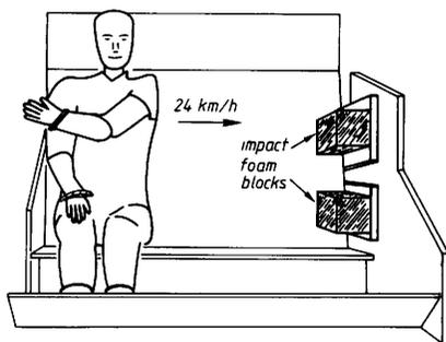
Fig. 17. Test set-up INRETS padded wall sled tests.
