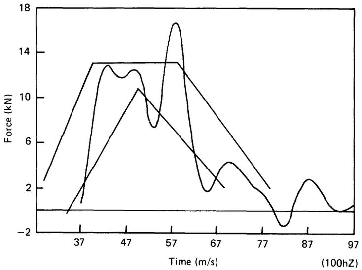
**Fig.8 Thoracic wall force, 20mile/h (8.9m/s) rigid wall test and performance corridor (Ref.8)**
