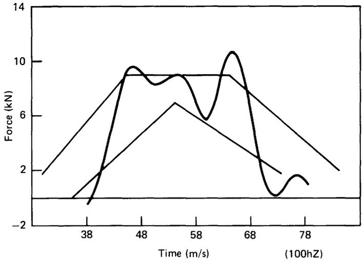
**Fig.7 Thoracic wall force, 15 mile/h (6.7m/s) rigid wall test and performance corridor ( 9Ref.8)**
