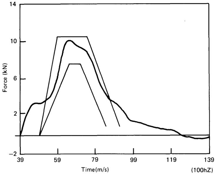
**Fig.9 Thoracic wall force, 15mile/h (6.7m/s) padded wall test and performance corridor (Ref.9)**
