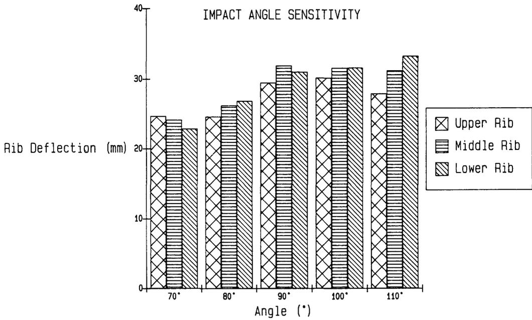
Fig. 7 : Comparison of peak rib deflection for the five impact angles
