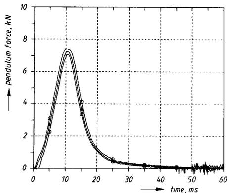
Fig. 14. Pendulum force versus time corridor (o-o), including mean result ( $\Delta$ - $\Delta$ ), obtained from TNO pelvis repeatability tests.
