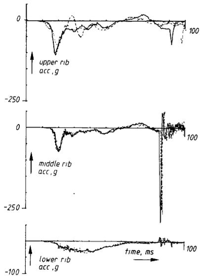
Fig. 21. Lateral chest acceleration versus time histories obtained from three padded wall (APR-padding) sled tests performed by INRETS.
