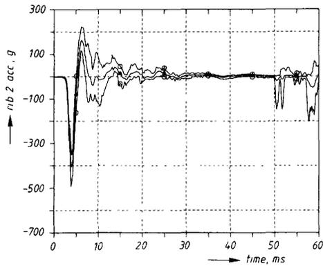
Fig. 10. Middle rib acceleration versus time corridor (o-o), including mean result ( $\Delta$ - $\Delta$ ), obtained from TNO chest repeatability tests (slope alignment applied).
