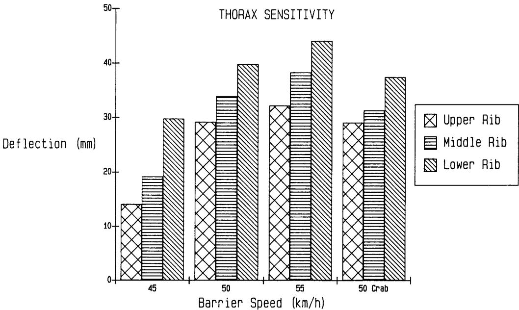
Fig. 20 : Thoracic deflection in MDB tests at different speeds, and for crabbed configuration
