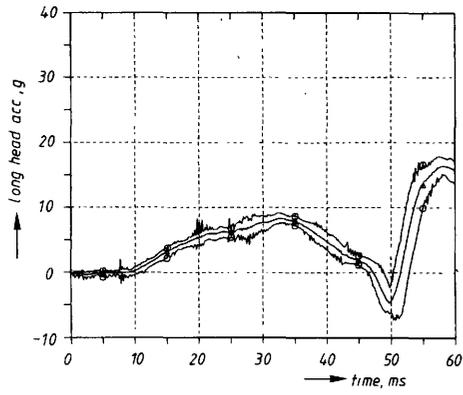
Fig. 4. Longitudinal head acceleration versus time corridor (o-o), including mean result ( $\Delta$ - $\Delta$ ), obtained from TNO neck repeatability tests.
