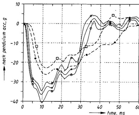
Fig. 2. Pendulum acceleration versus time corridor (o-o) including mean results (Δ-Δ), obtained from TNO neck repeatability test, compared with the APR corridor (●-□).
