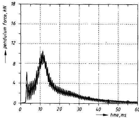
Fig. 13. Pendulum force versus time corridor (o-o), including mean result ( $\Delta$ - $\Delta$ ), obtained from TNO abdomen repeatability tests (slope alignment applied).
