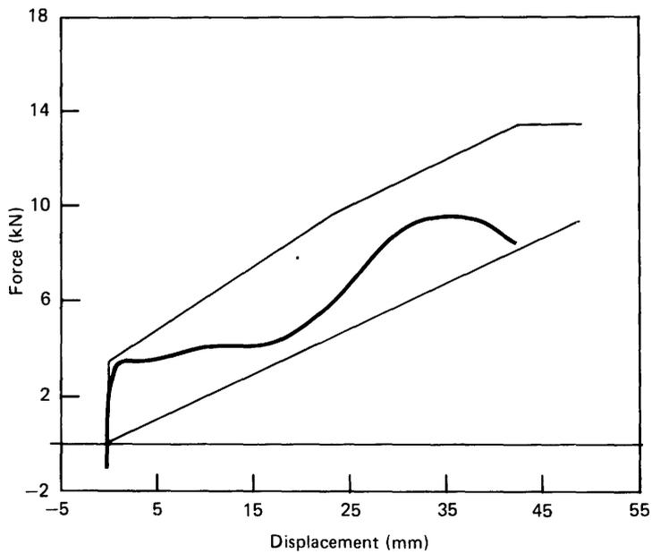
**Fig.6 Thorax force-displacement curve for padded wall test and performance corridor based on APR cadaver tests**
