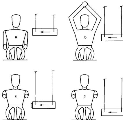
Fig. 7. Test set-up impactor tests; shoulder repeatability tests (a), chest repeatability tests (b), abdomen repeatability tests (c) and pelvis repeatability tests (d).
