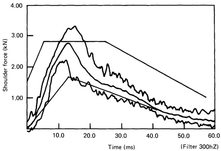
Fig.2 Shoulder force produced by a 23.4kg impactor at 4.3m/s
