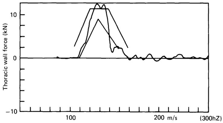
**Fig.12 15mile/h Rigid wall test. Thoracic wall force
