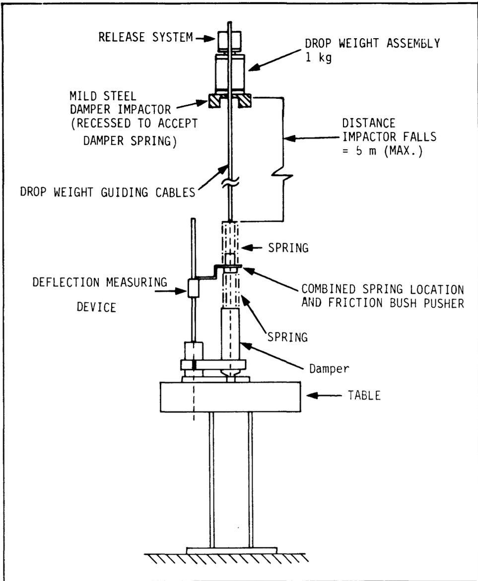
Figure 5: Rib Certification Rig with Damper-Spring Unit
