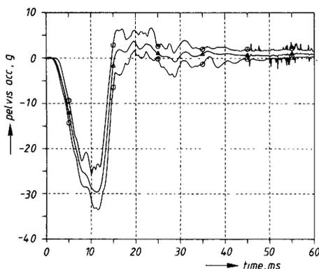
Fig. 15. Lateral pelvis acceleration versus time corridor (o-o), including mean result ( $\Delta$ - $\Delta$ ), obtained from TNO pelvis repeatability tests.
