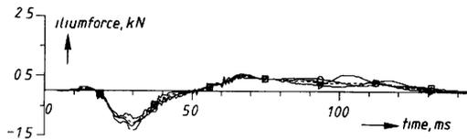
Fig. 32. Left ilium force versus time histories, including mean result (----), obtained from three MDB tests performed by BAST.
