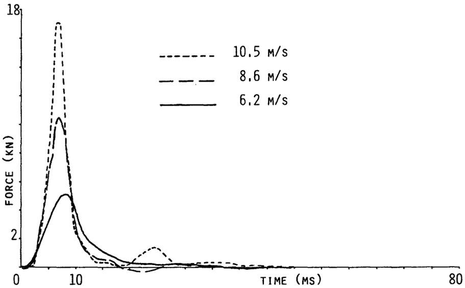
Fig. 14 : Time histories of pubic force in impactor tests for three impact speeds
