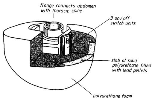
Fig. 5. First prototype of EUROSID abdomen section.
