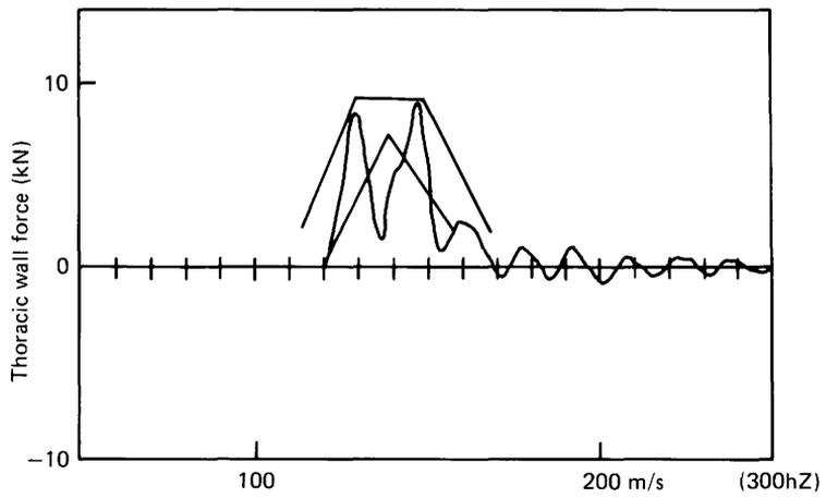
**Fig.10 15mile/h Rigid wall test. Thoracic wall force Arm (steel skeleton) 40° forward**
