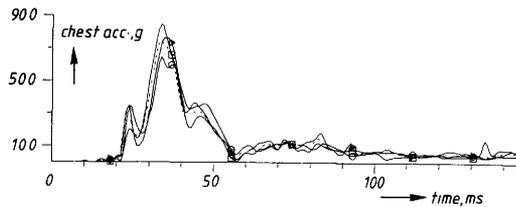
Fig. 27. Resultant chest acceleration versus time histories, including mean result (----), obtained from three MDB tests performed by BAST.
