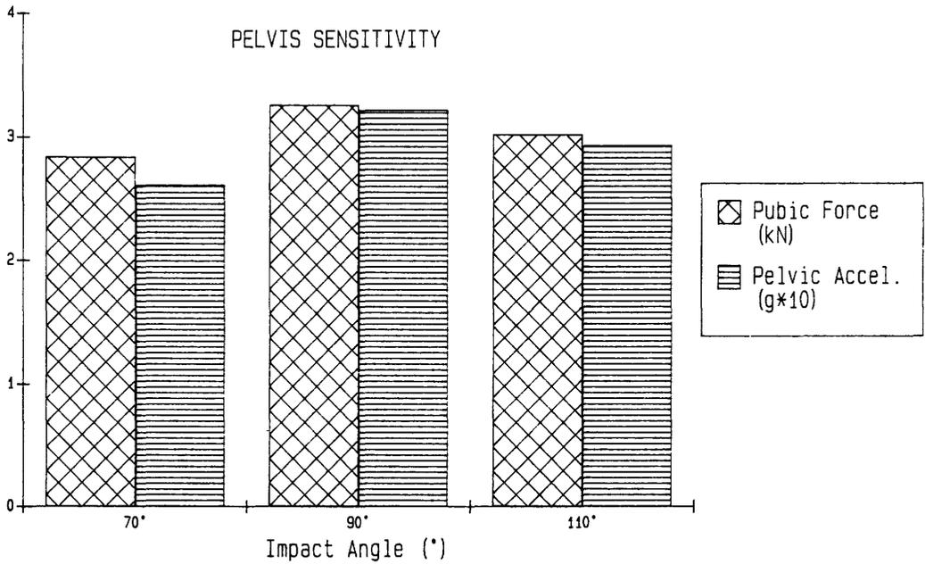
Fig. 18 : Sensitivity of the pelvis to impact angle
