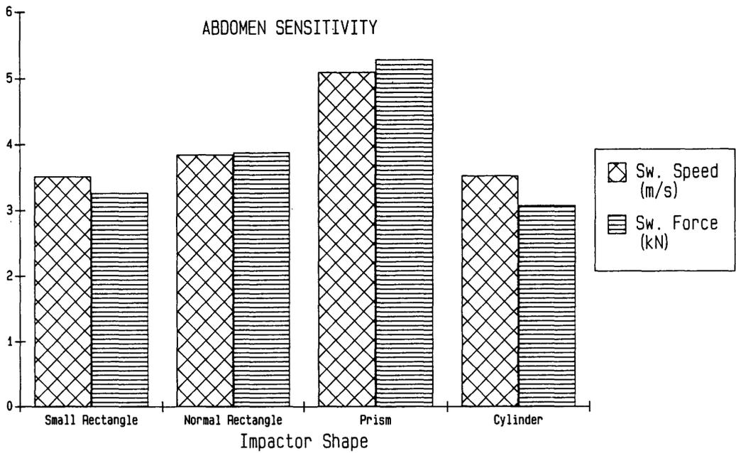
Fig. 11 : Effect of impactor shape on abdominal switching speed and switching force
