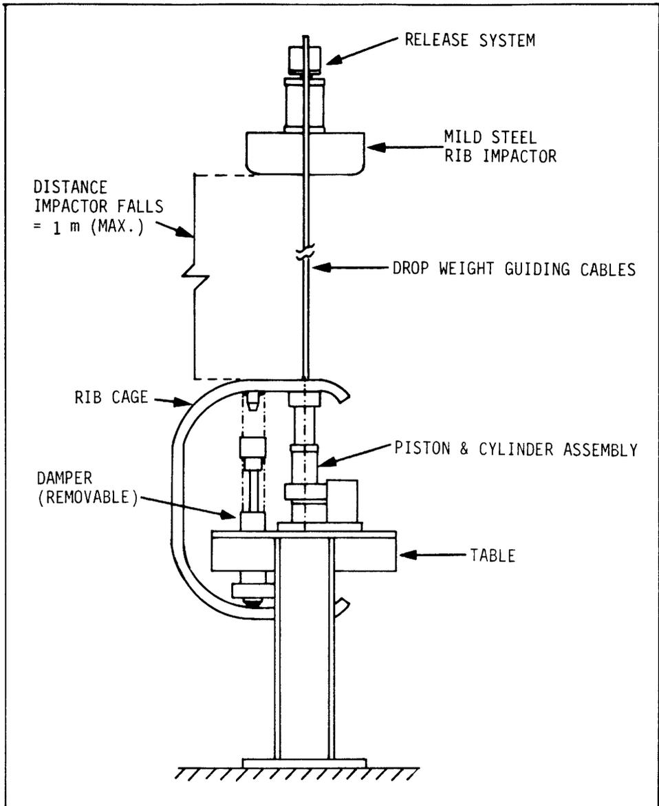
**Figure 4:** Rib certification rig with complete rib module.
