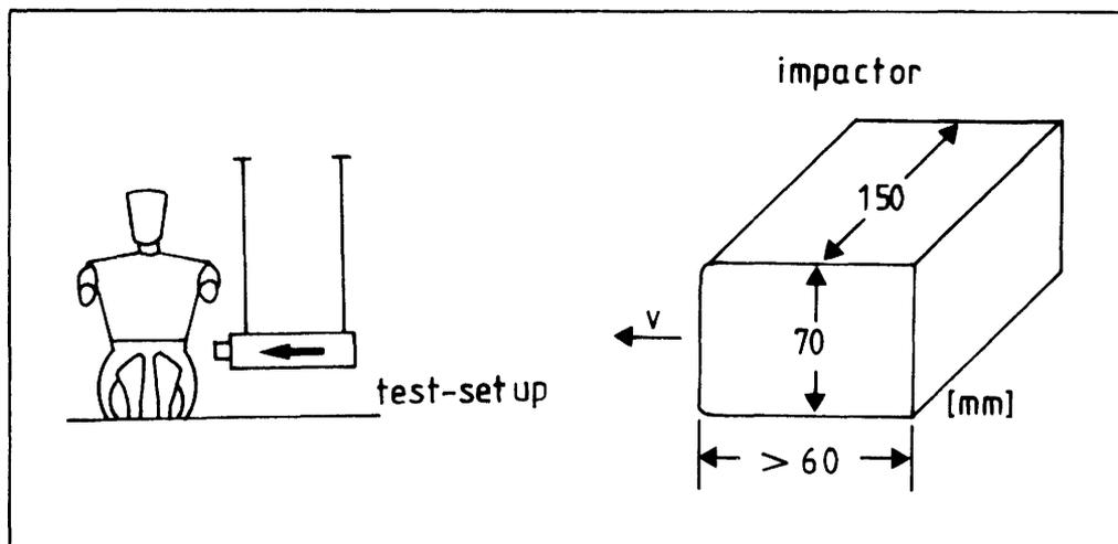
Figure 6: Test Set-Up and Impactor Face for EUROSID Abdomen Certification
