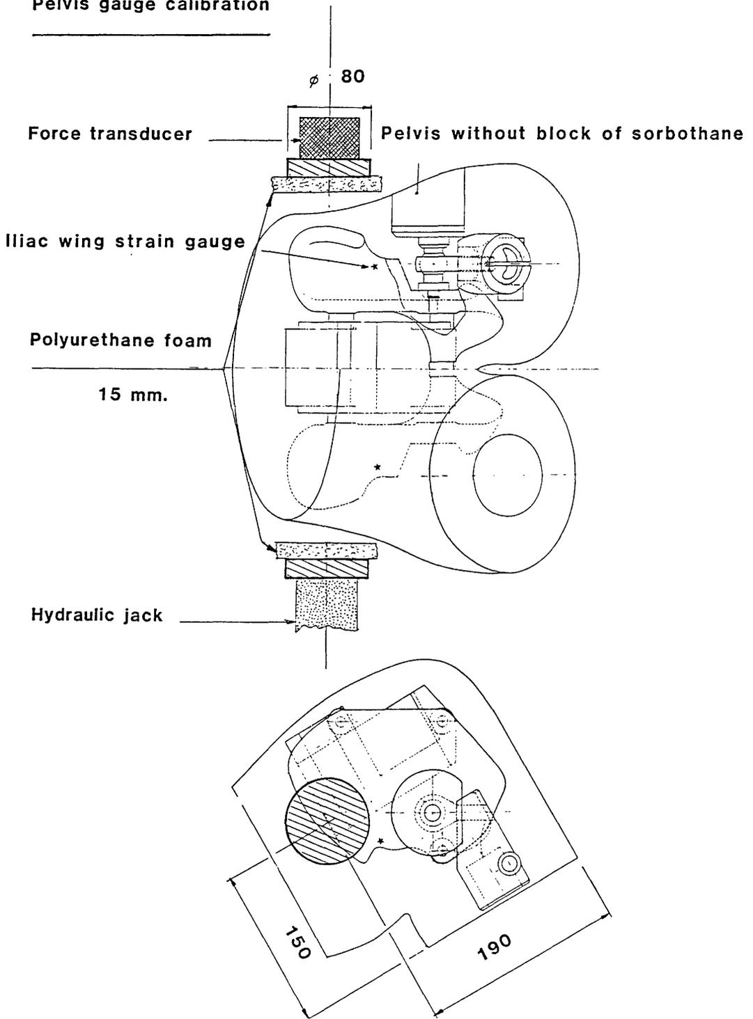
**Fig 7 Pelvis gauge calibration**
