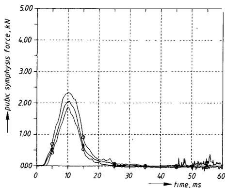
Fig. 16. Pubic symphysis force versus time corridor (o-o), including mean result ( $\Delta$ - $\Delta$ ), obtained from TNO pelvis repeatability tests.
