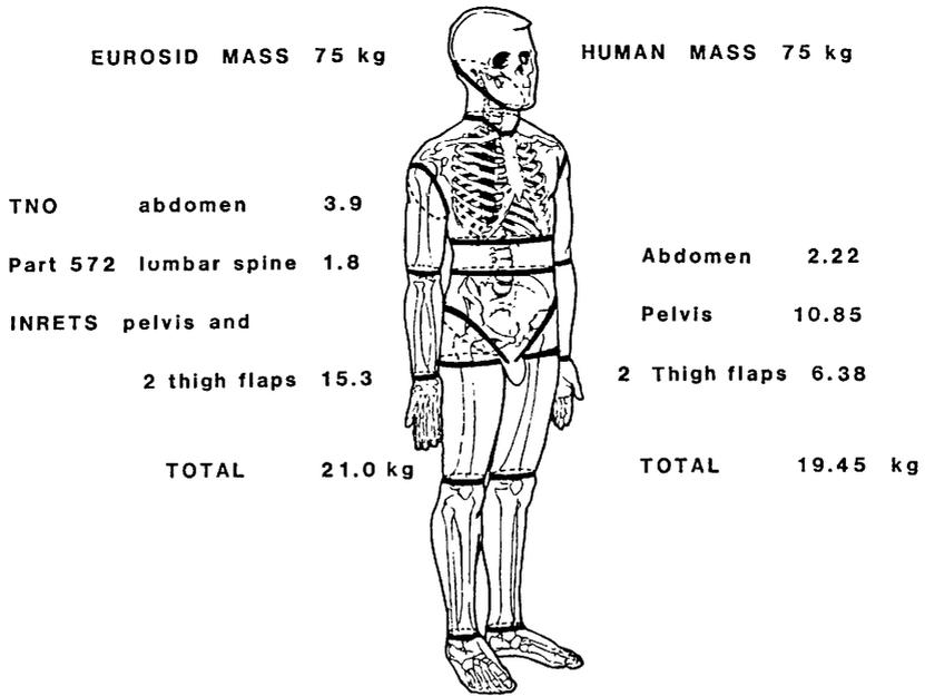
**Fig 4 Total body segmentation scheme**
