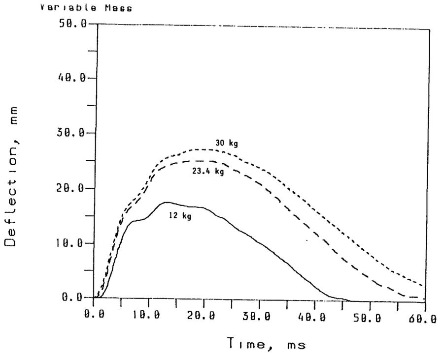
Fig. 4 : Time histories of rib deflection for three pendulum masses
