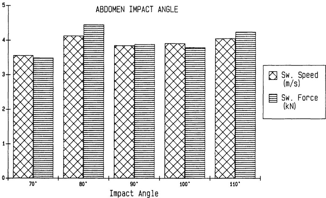
Fig. 10 : Abdominal switching speed and switching force as a function of impact angle
