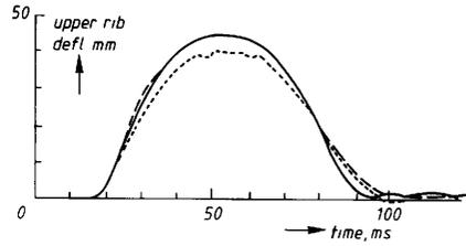
Fig. 19. Middle rib deflection versus time histories obtained from three padded wall (APR-padding) sled tests performed by INRETS.
