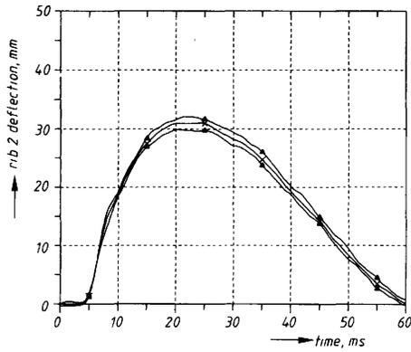
Fig. 9. Middle rib deflection versus time corridor ( $\Delta$ - $\Delta$ ), including mean result (x-x), obtained from TNO chest repeatability tests (slope alignment applied).
