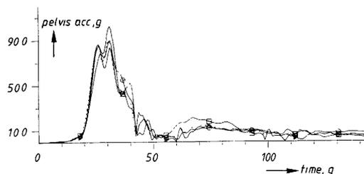
Fig. 30. Resultant pelvis acceleration versus time histories, including mean result (----), obtained from three MDB tests performed by BAST.
