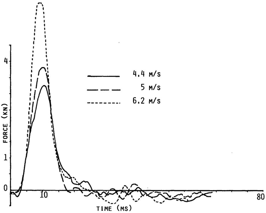
Fig. 13 : Time histories of pubic force in pendulum tests for three impact speeds
