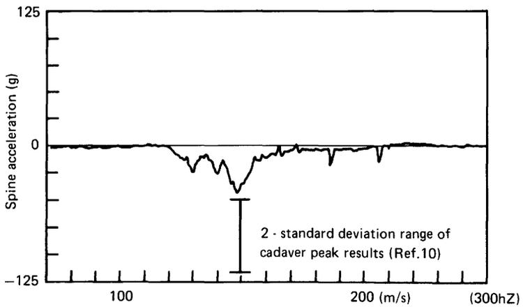
**Fig.14 15mile/h Rigid wall test. Spine acceleration
