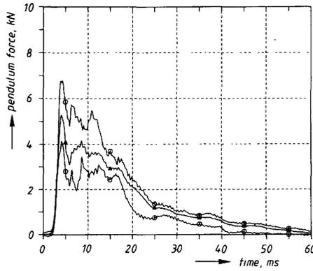
Fig. 12. Pendulum force versus time corridor (o-o), including mean result ( $\Delta$ - $\Delta$ ), obtained from TNO chest repeatability tests (slope alignment applied).
