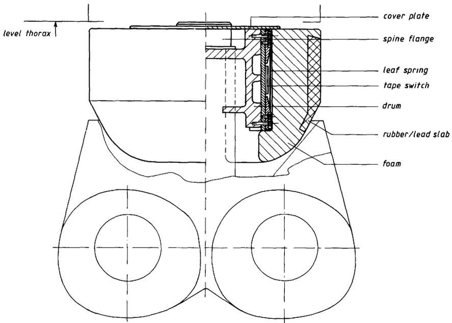
Fig. 8. Production prototype of EUROSID abdomen section.
