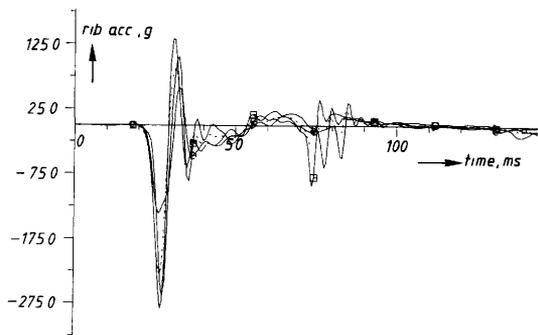
Fig. 28. Middle rib acceleration versus time histories, including mean result (----), obtained from three MDB tests performed by BAST.
