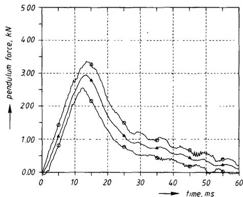
Fig. 8. Pendulum force versus time corridor (o-o), including mean result (Δ-Δ), obtained from TNO shoulder repeatability tests.
