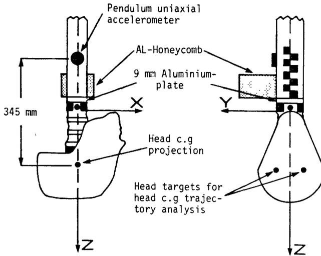
Figure 1: Neck Certification Test Set-Up
