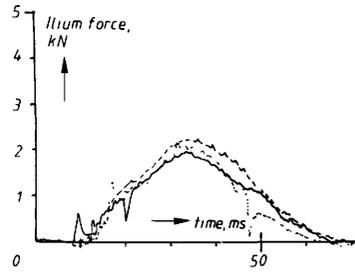
Fig. 23. Pubic symphysis force versus time histories obtained from three padded wall (APR-padding) sled tests performed by INRETS.
