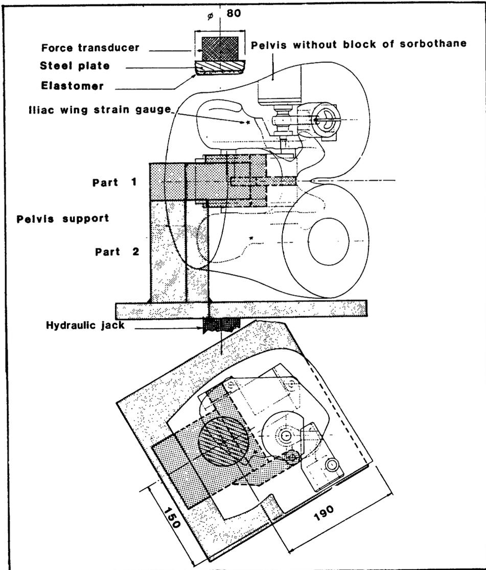
Figure 7: Pelvis Strain Gauge Calibration Test Set-Up
