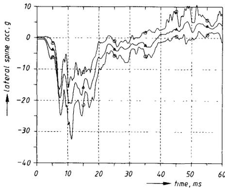
Fig. 11. Lateral spine acceleration versus time corridor (o-o), including mean result ( $\Delta$ - $\Delta$ ), obtained from TNO chest repeatability tests (slope alignment applied).
