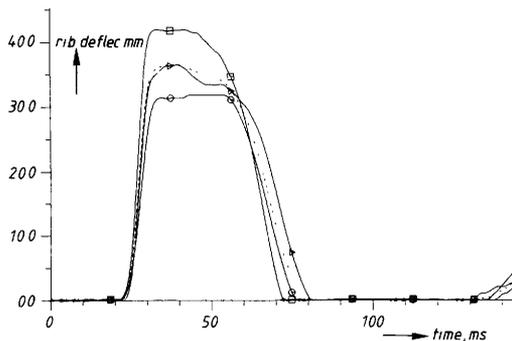
Fig. 29. Middle rib deflection versus time histories, including mean result (----), obtained from three MDB tests performed by BAST.
