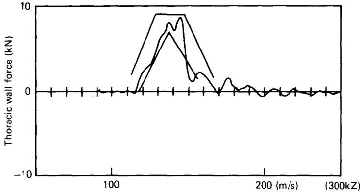
**Fig.11 15mile/h Rigid wall test. Thoracic wall force
