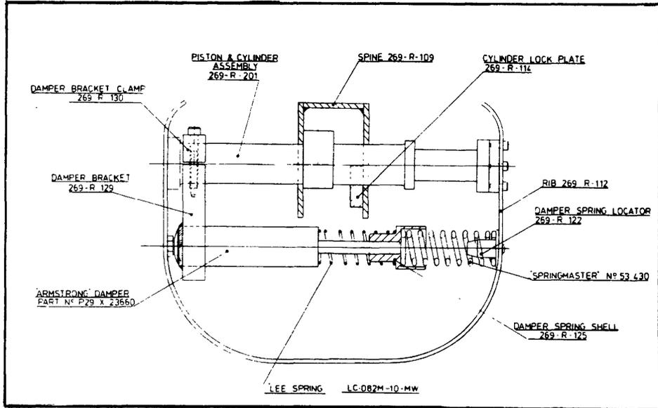
Figure 3: Rib module of the EUROSID
