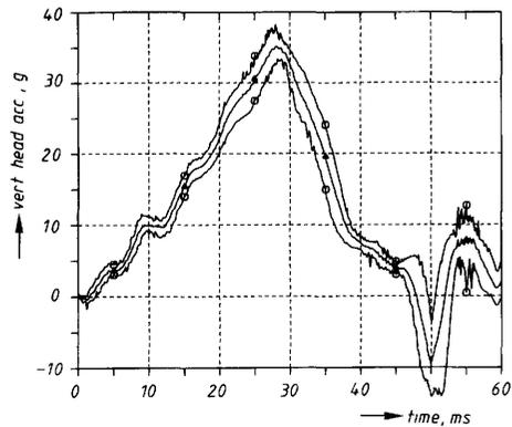
Fig. 6. Vertical head acceleration versus time corridor (o-o), including mean result ( $\Delta$ - $\Delta$ ), obtained from TNO neck repeatability tests.
