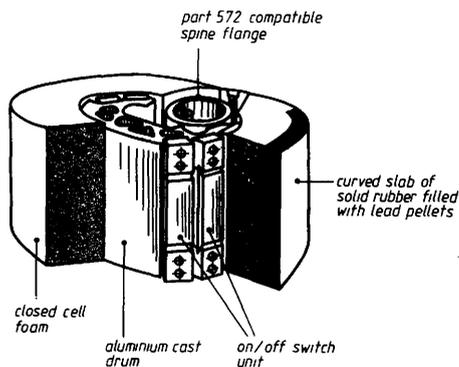
Fig. 4. Early prototype of TNO abdomen section (partly cut open to show principle).
