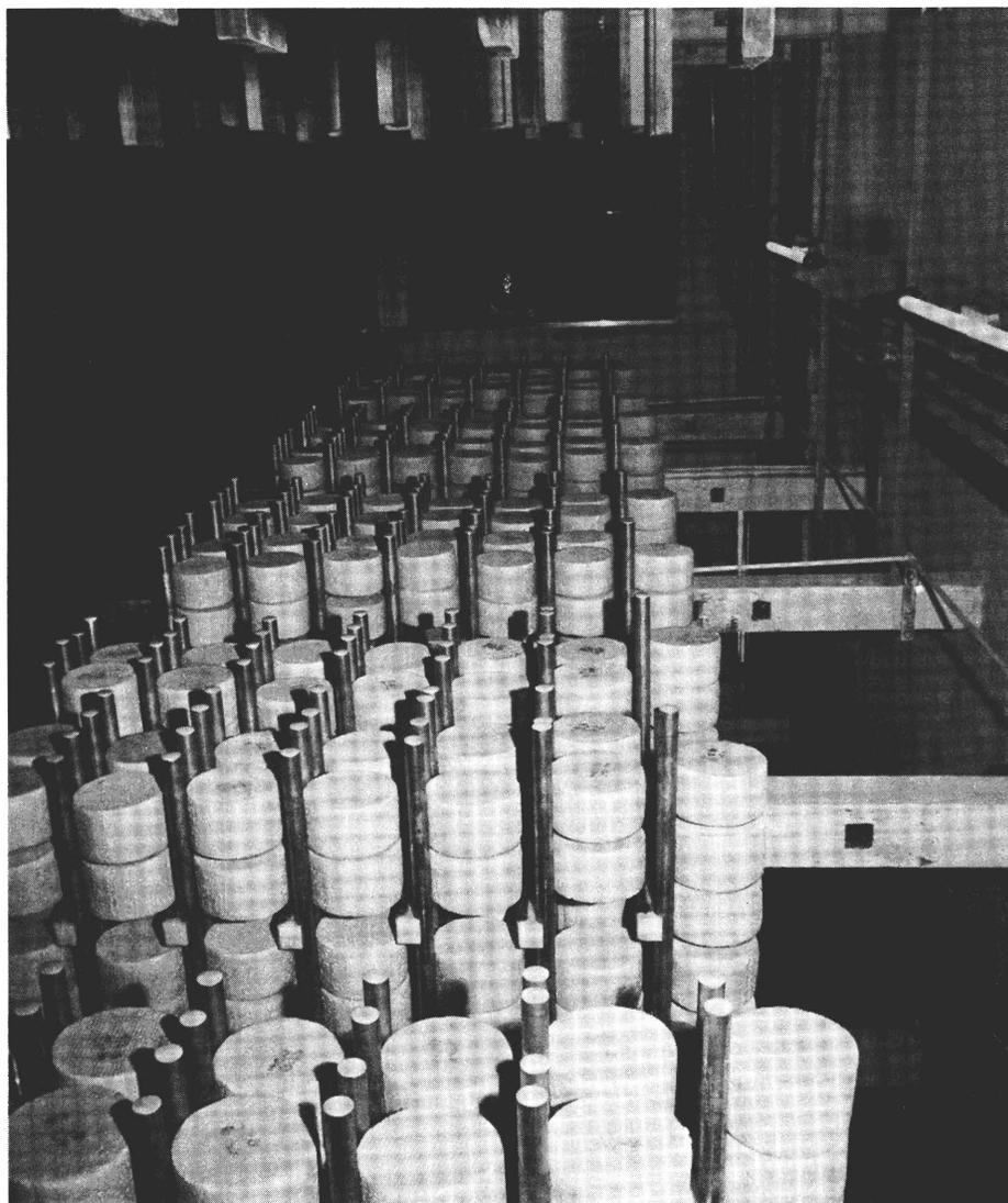
*manufacture of blue-veined cheese, for instance, takes place continuously without any human contact at the impressive rate of one cheese per second. The cheese is left to set, after which it is salted and stored for from five to six weeks at constant temperature and humidity. Finally it is washed and packaged. The EC Member States are the main buyers, but considerable quantities are also exported to other parts of the world, such as Canada, the USA, and Australia.*
