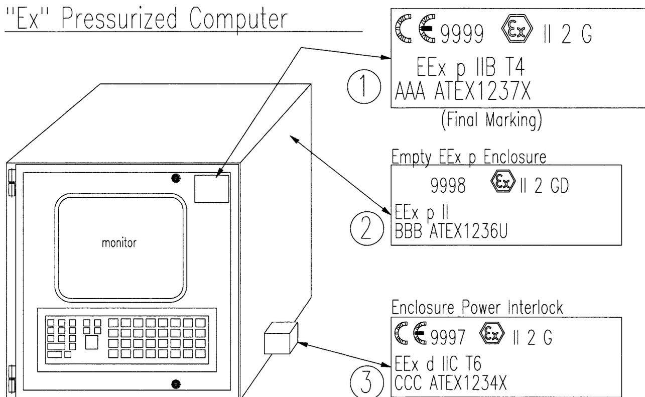
The system comprises a computer, which is adapted for safe use in a potentially explosive atmosphere by being contained within a pressurized atmosphere, within an enclosure, which also contains the pressurization control system and an interlock that will only allow power to be supplied when the enclosure has been purged. Power to the system is provide via a sealed cable gland. The system is designed in conformity with the pressurization protection standard "p" (EN 50016)
