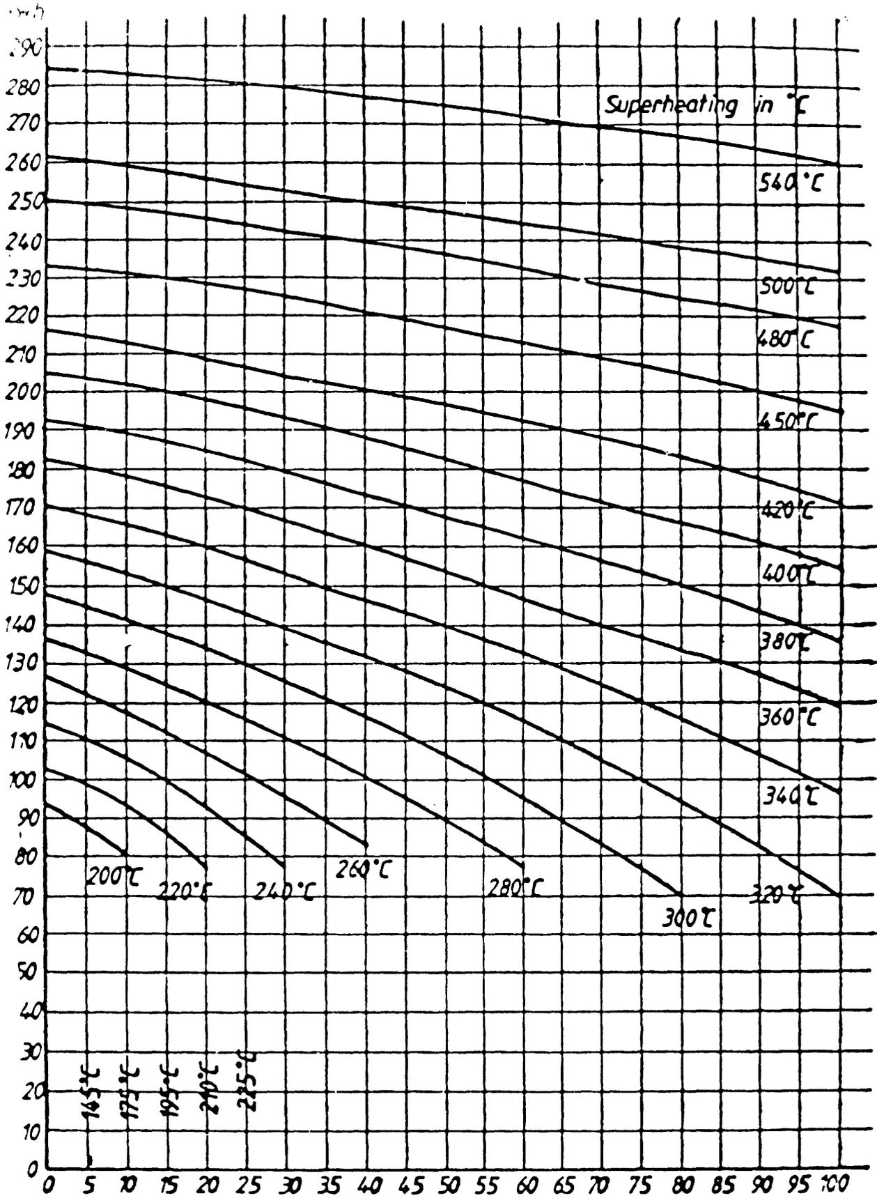
Figure 1. Energy content of 1 ton superheated steam in kWh by condensing to 20°C
