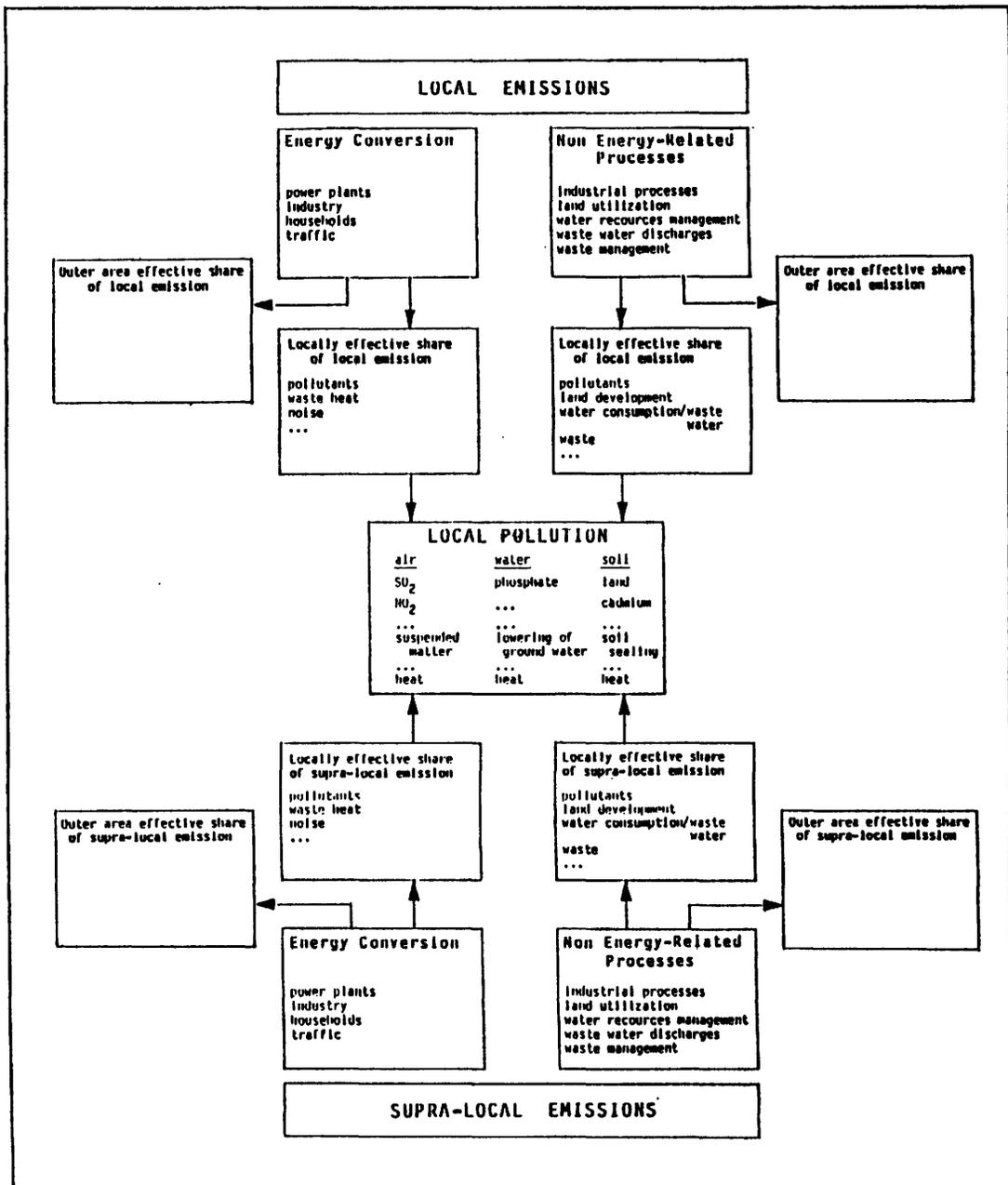
Figure 5. Structure of a Comprehensive Energy-environmental Planning Model.
