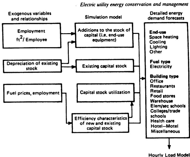
Figure 9. Schematic Diagram of Disaggregated Commercial Energy End-Use Forecasting Model.
