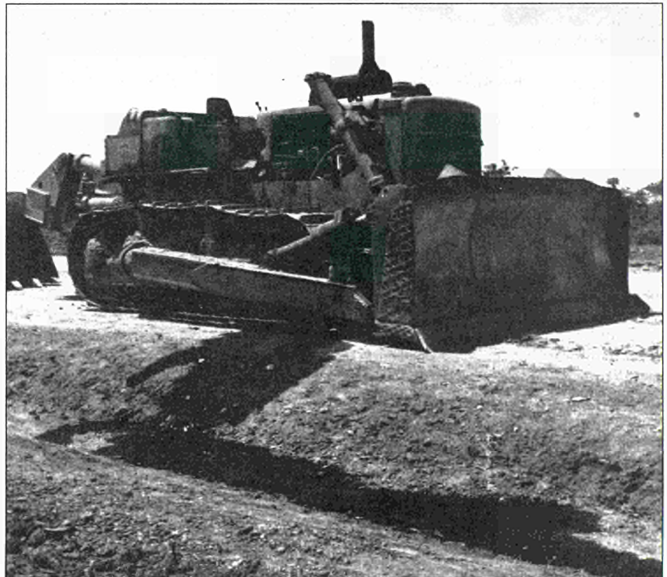
'Problems with the operation of equipment fleets'. Lack of maintenance has immobilised this earth mover
