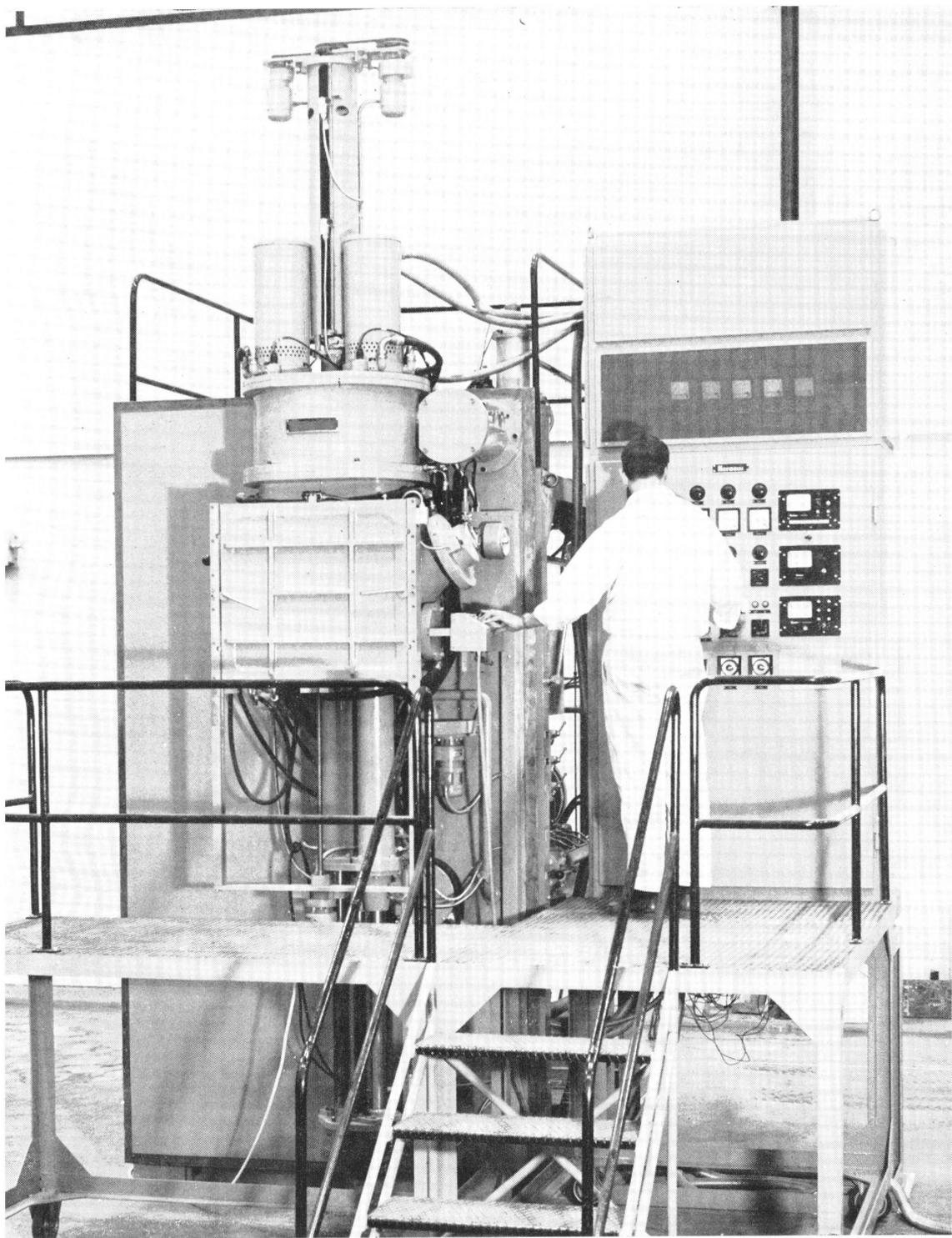
KARLSRUHE — FOUR DE FUSION PAR BOMBARDEMENT D'ELECTRONS
