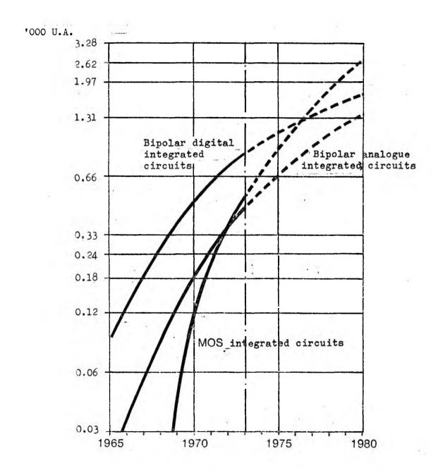
Source: Electronic Components Programme of the Federal Republic of Germany 1974 - 1978 b) Drop in price per logical unit (transistor) with complete integration.
