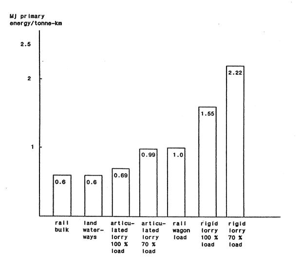
[articulated lorry = 5 axle articulated 38 tons] [rigid lorry = 4 axle rigid 20 tons] Figure 4
